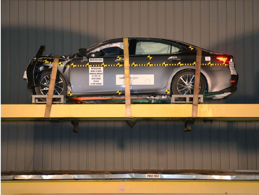
FIGURE 72. Vehicle at 0° on Static Rollover Device
