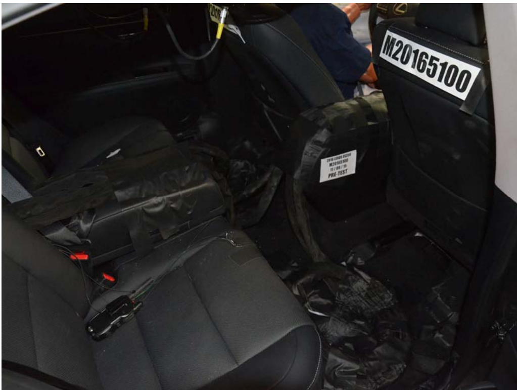
FIGURE 27. Pre-Test Dummy Cable Routing
