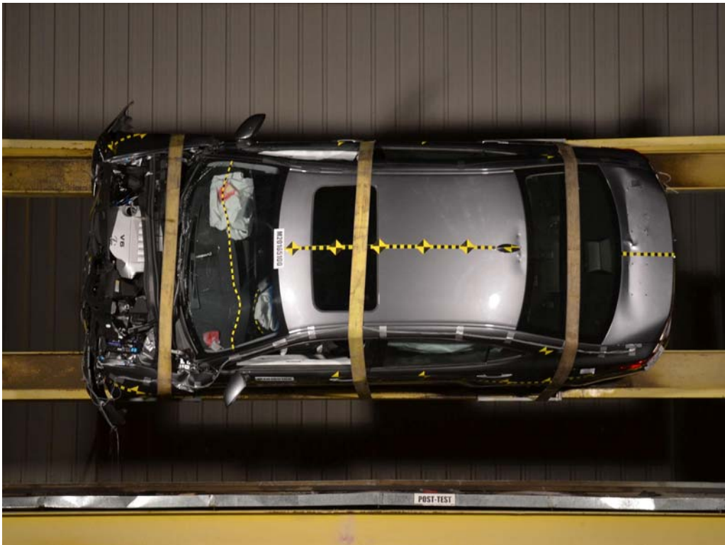
FIGURE 73. Vehicle at 90° on Static Rollover Device
