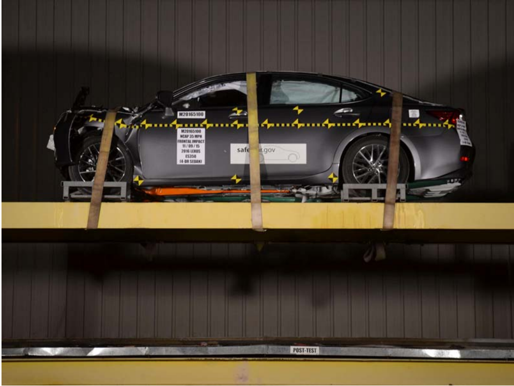
FIGURE 76. Vehicle at 360° on Static Rollover Device
