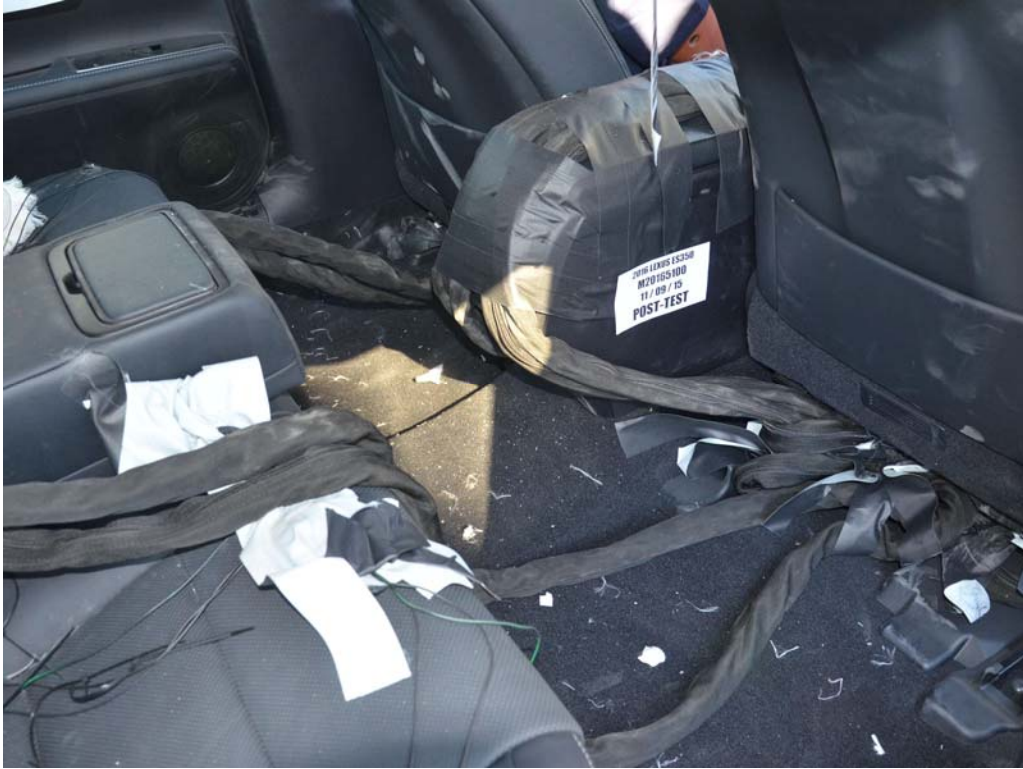
FIGURE 28. Post-Test Dummy Cable Routing
