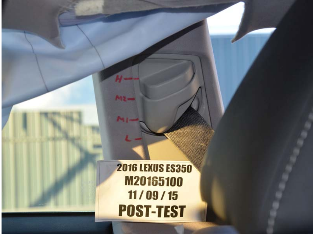
FIGURE 38. Post-Test View of Belt Anchorage for Driver Dummy
