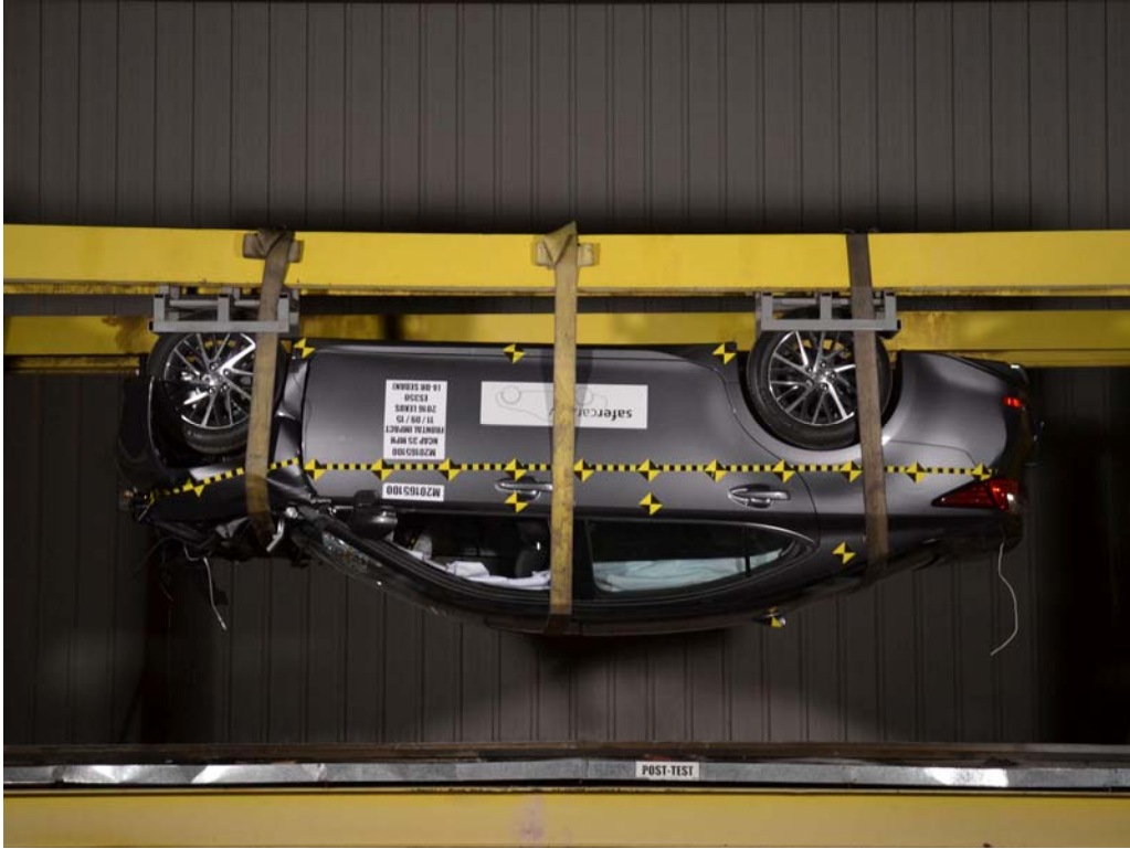
FIGURE 74. Vehicle at 180° on Static Rollover Device
