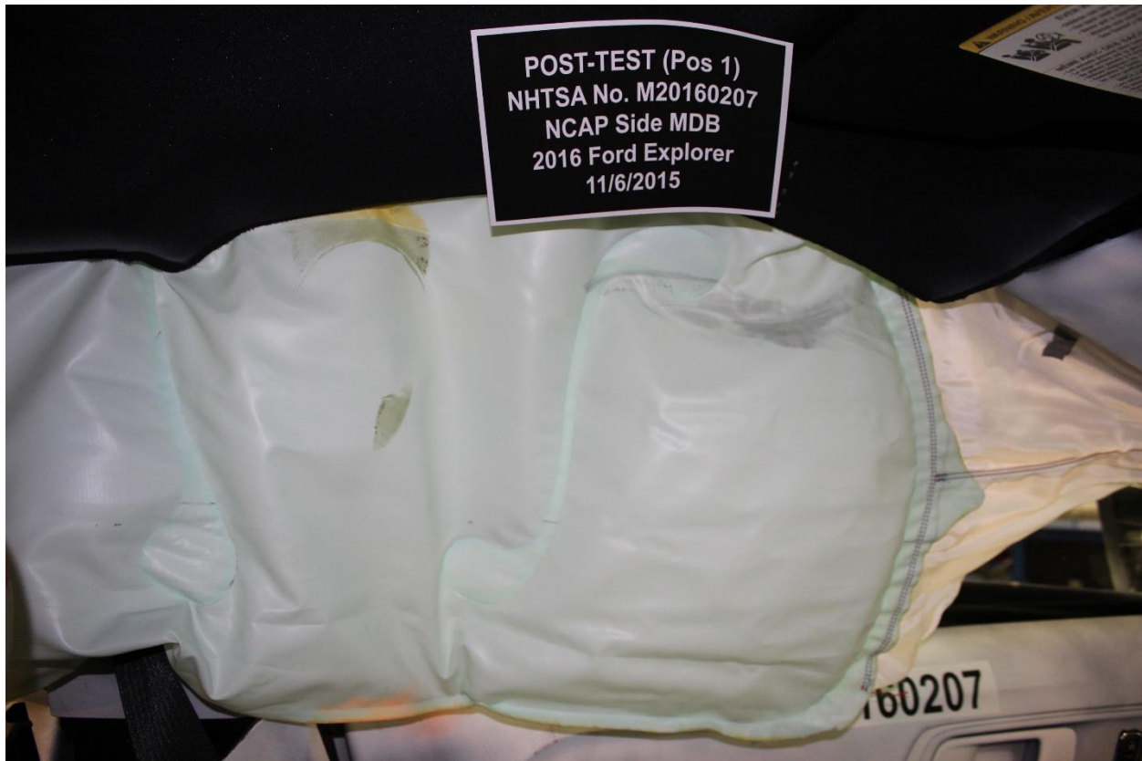
Figure A-49: Post-Test Driver Dummy Close-Up Head Contact with Side Airbag View
