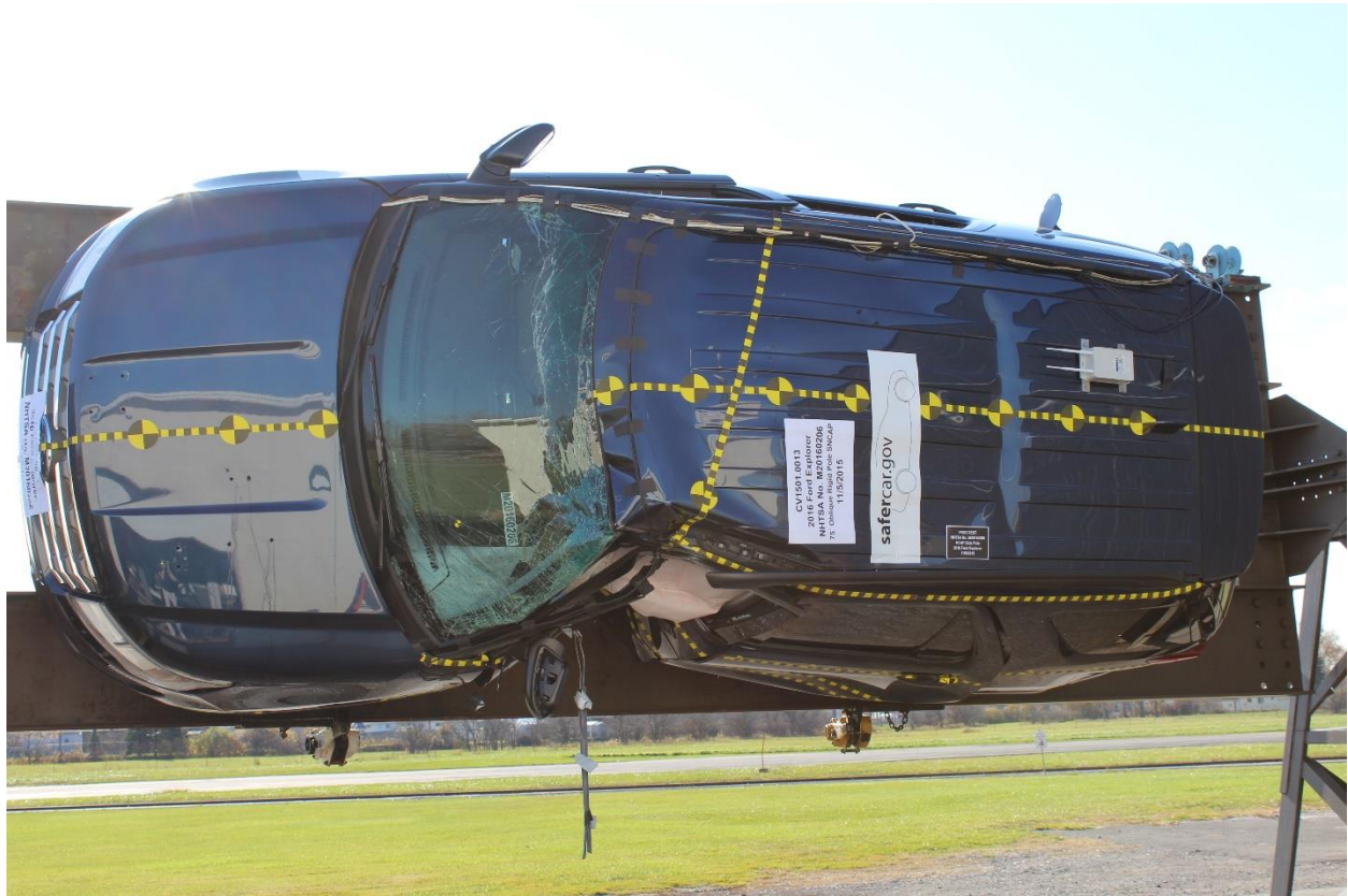
Figure A-66: FMVSS No. 301 Static Rollover 270 Degrees
