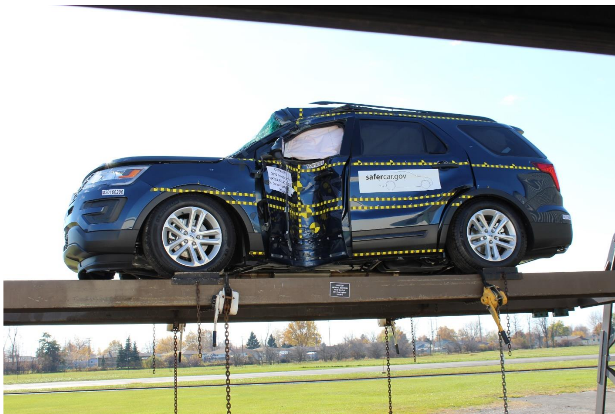
Figure A-63: FMVSS No. 301 Static Rollover 0 Degrees
