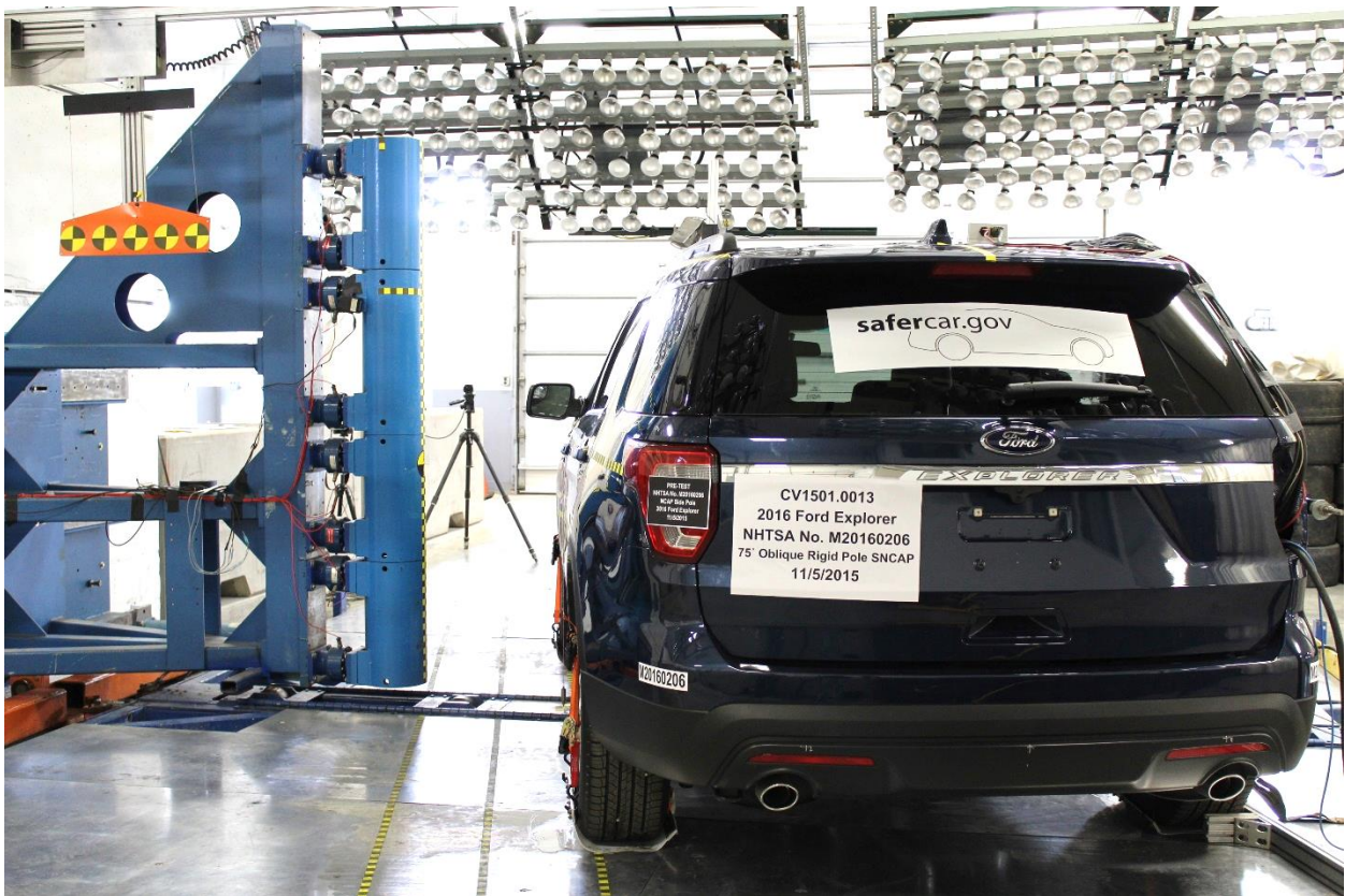
Figure A-18: Pre-Test Right Side View of Pole Positioned Against Side of Vehicle
