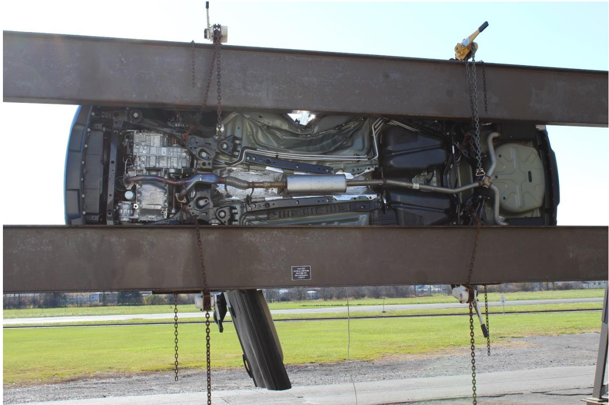
Figure A-64: FMVSS No. 301 Static Rollover 90 Degrees
