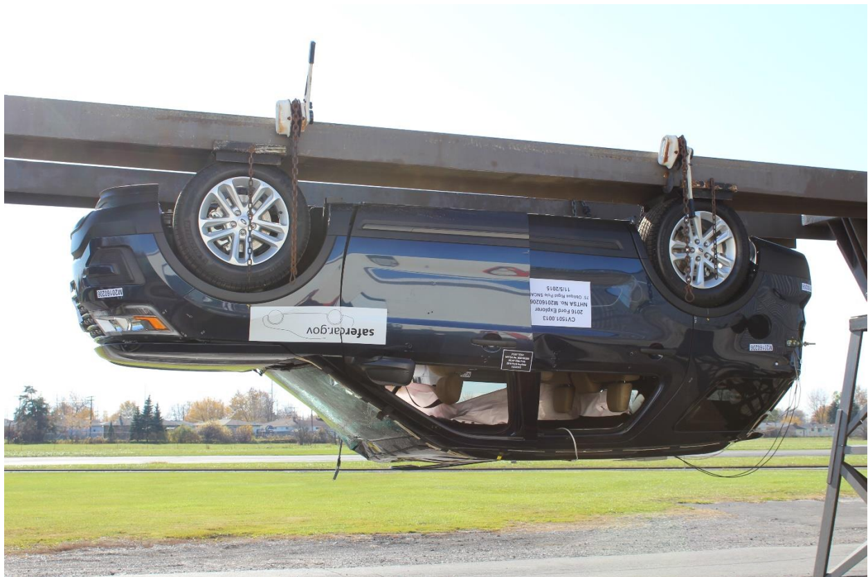
Figure A-65: FMVSS No. 301 Static Rollover 180 Degrees
