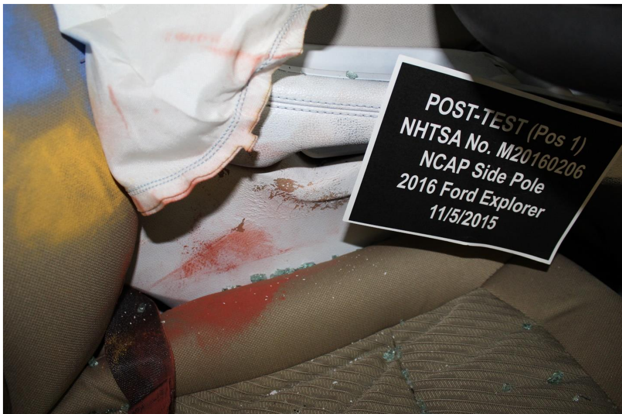
Figure A-50: Post-Test Dummy Close-Up Pelvis Contact with Vehicle Interior View
