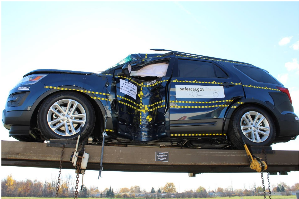
Figure A-67: FMVSS No. 301 Static Rollover 360 Degrees
