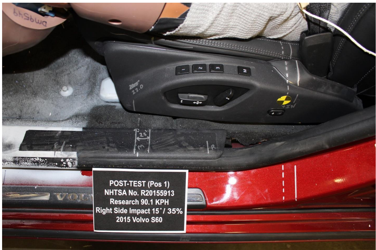
No. 062 Post-Test Driver Seat Fore Aft Markings
