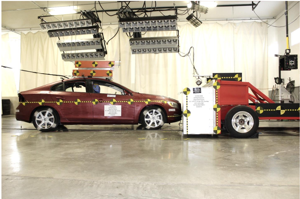
No. 185: Pre-Test OMDB & Vehicle, Left Side
