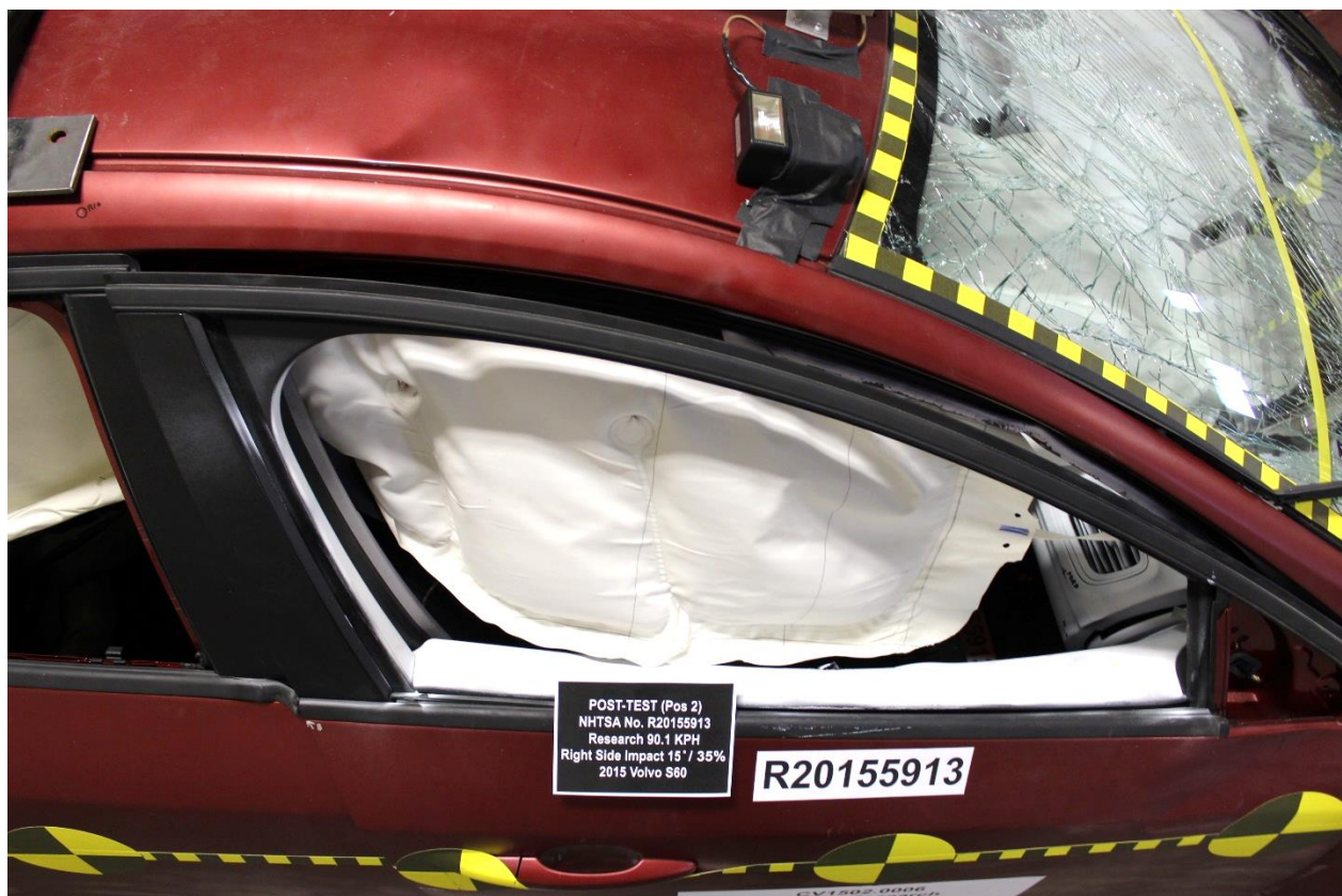
No. 103: Post-Test View of Passenger Door Clearance
