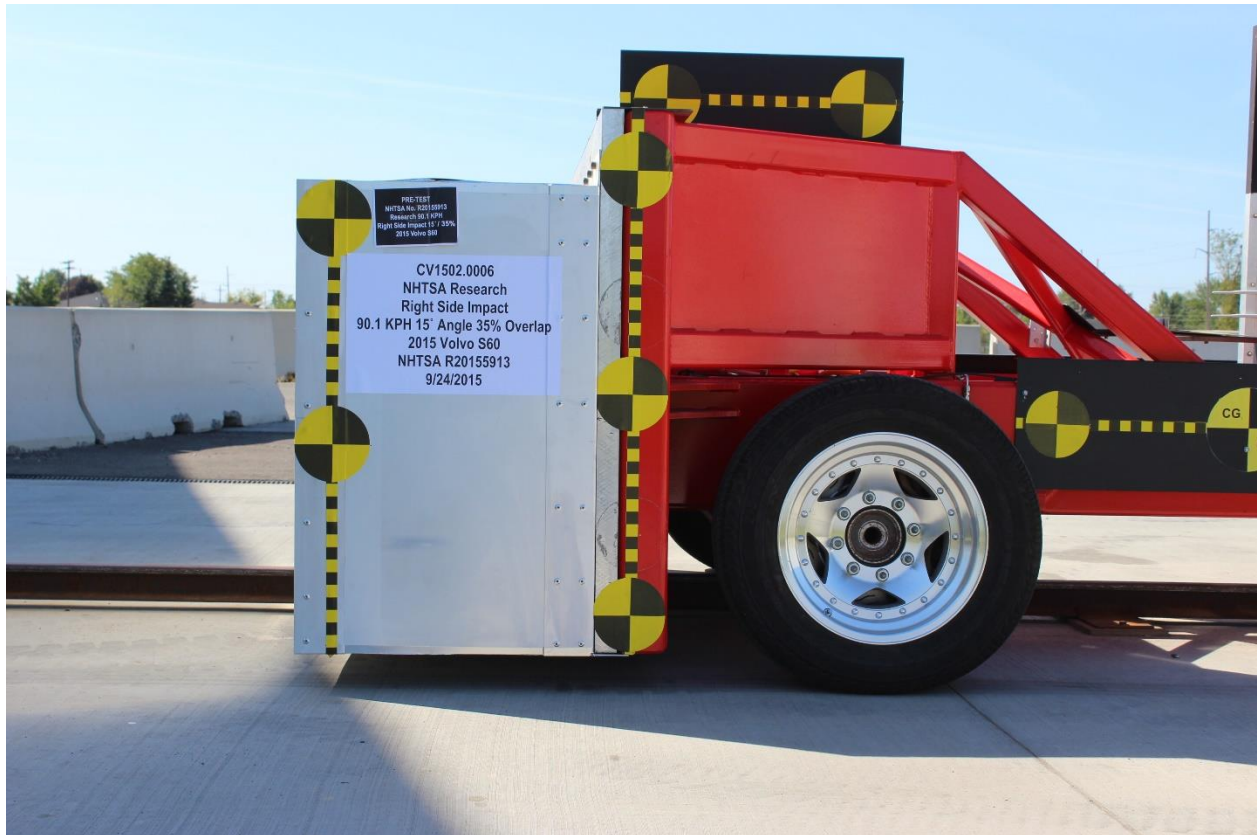
No. 167: Pre-Test Left Side View of OMDB
