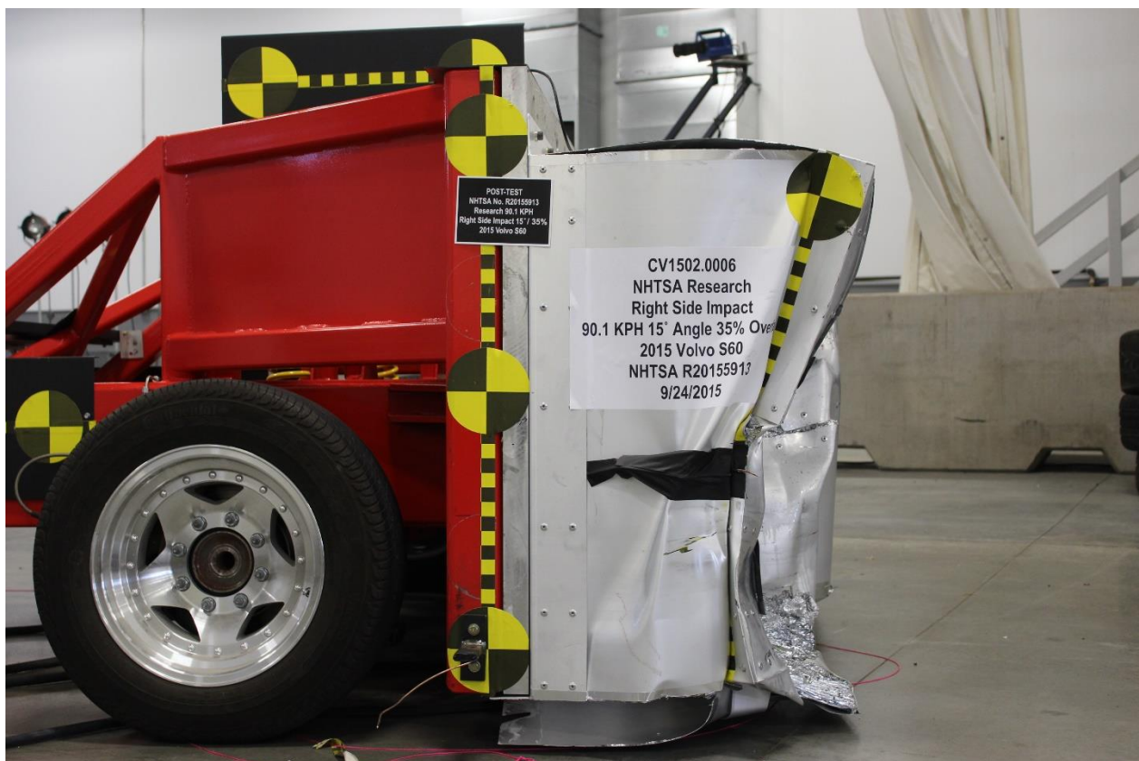
No. 170: Post-Test Right Side View of OMD
