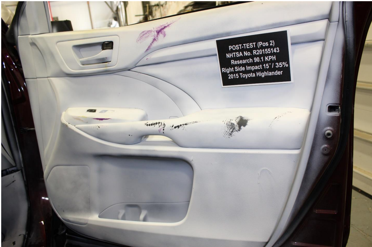
No. 037 Post-Test View of Passenger Inner Door Panel
