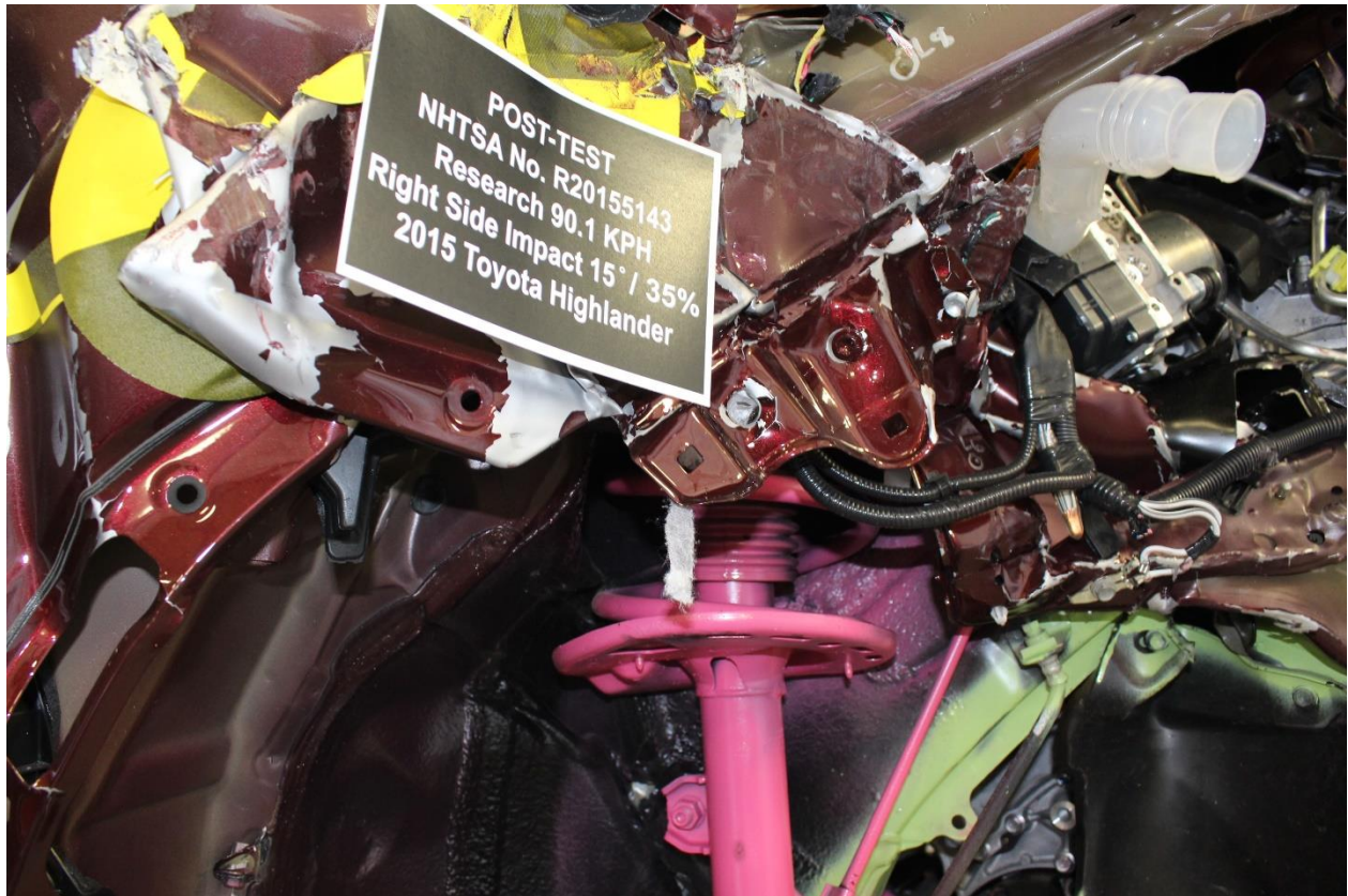
No. 159: Post-Test Front Passenger Close up View of Suspension w/ Tire Removed
