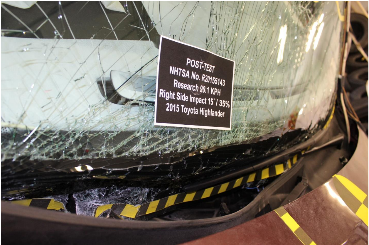
No. 166: Post-Test View of Windshield Separation
