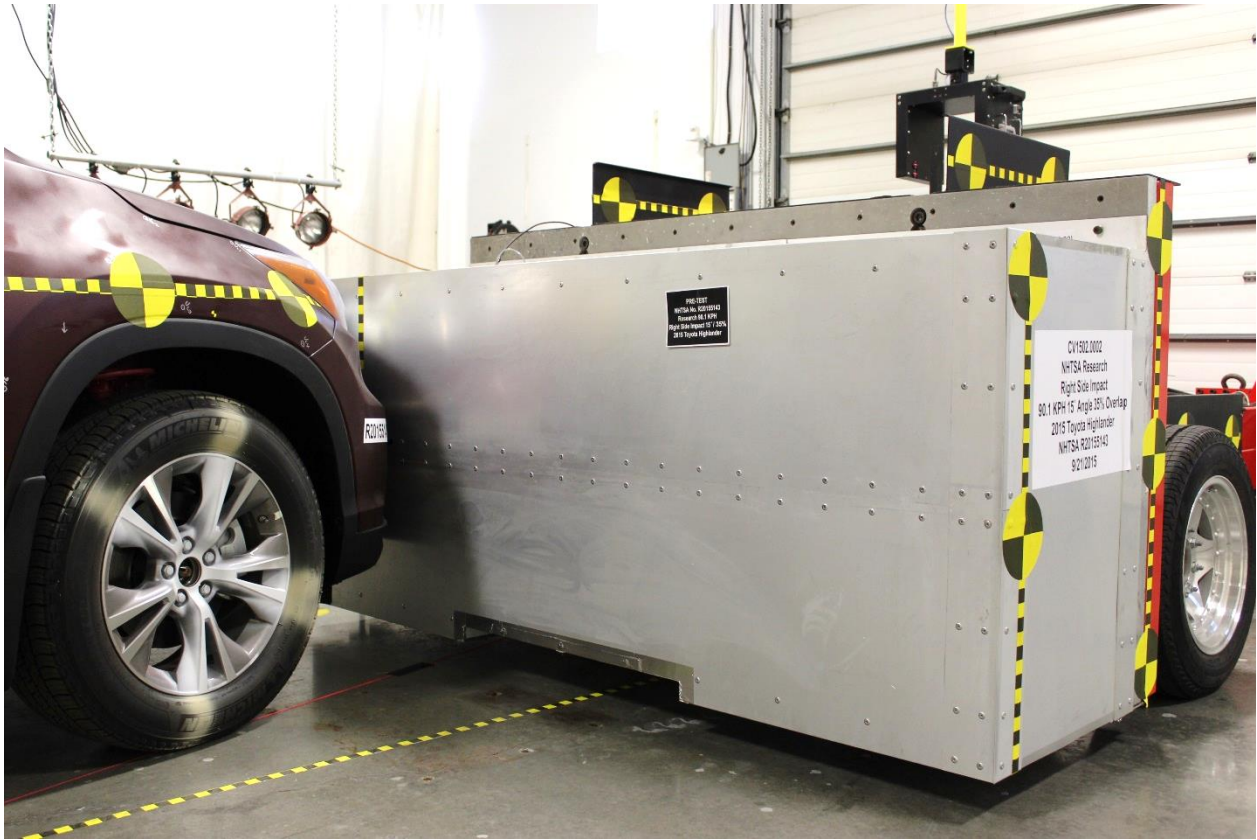
No. 193: Pre-Test OMDB & Vehicle Alignment
