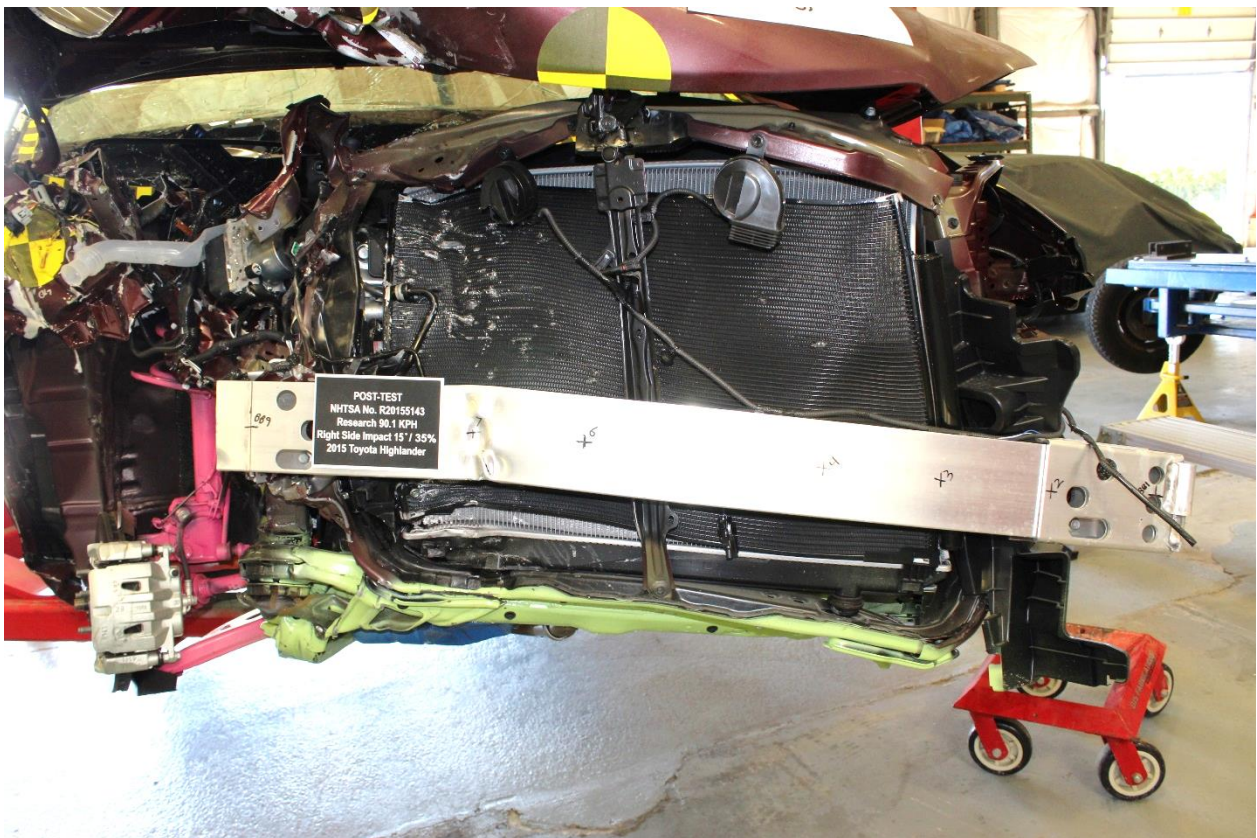
No. 205 Post-Test Vehicle Bumper Front View
