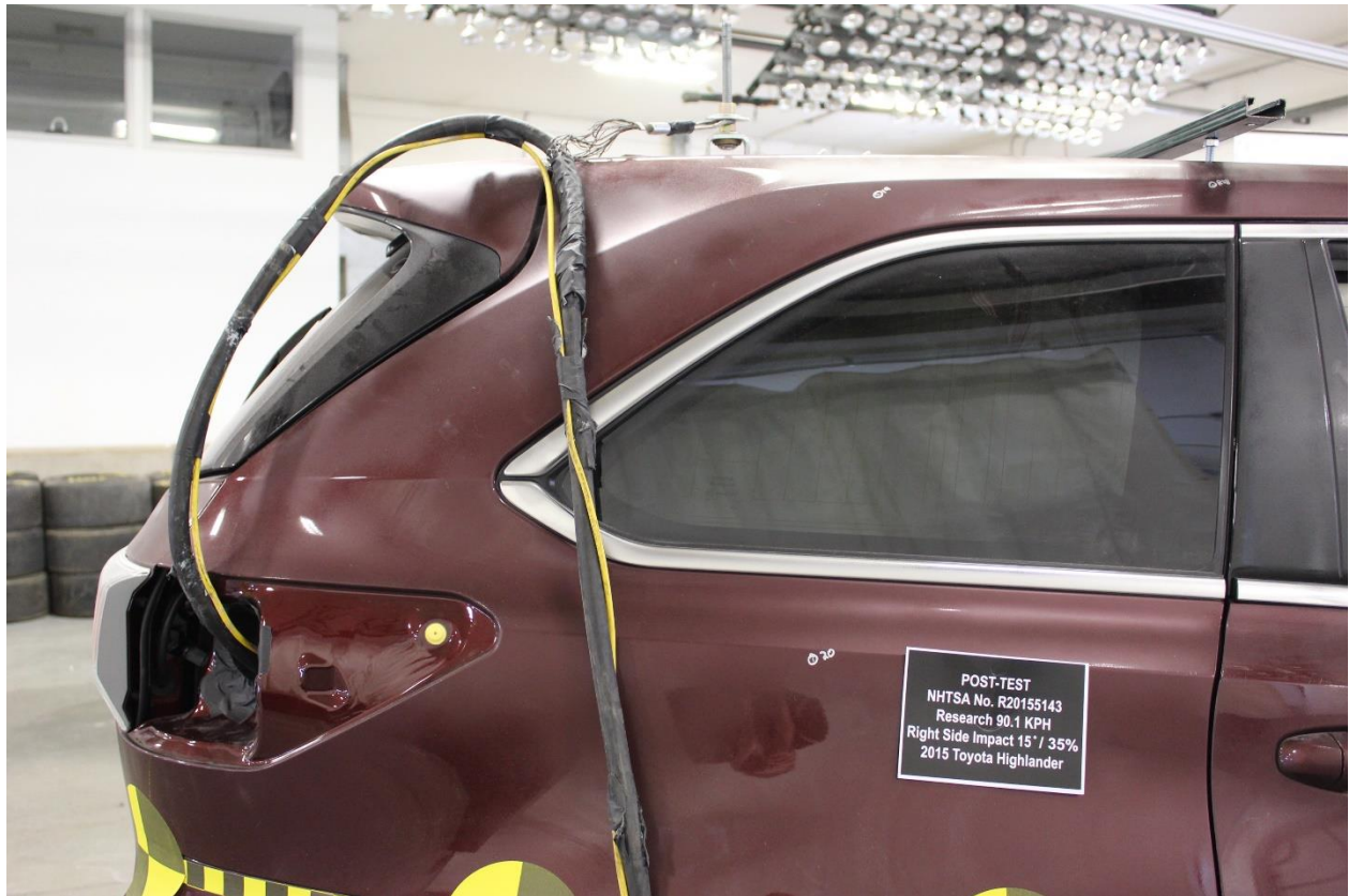
No. 163: Post-Test View of Deformation of C pillar-Struck Side
