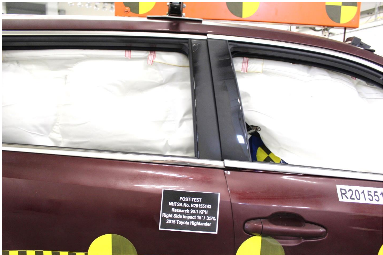
No. 162: Post-Test View of Deformation of B pillar-Struck Side
