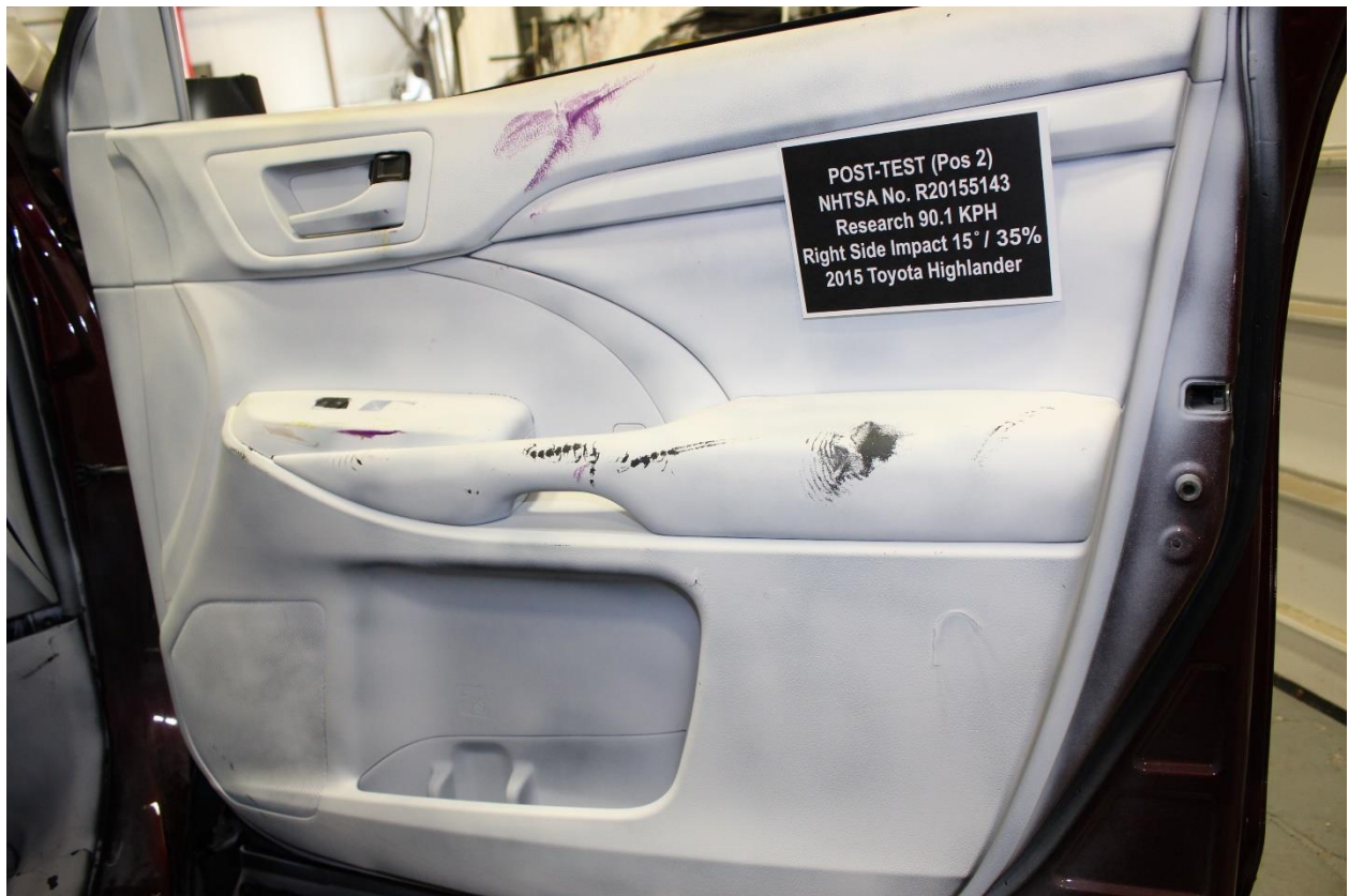
No. 121: Post-Test View of Passenger Body contact with Interior
