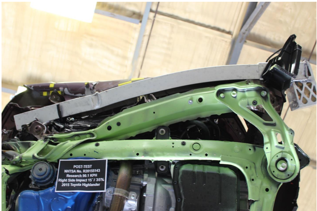
No. 143: Post-Test Bumper to Rail Attachments and Crush Initiators
