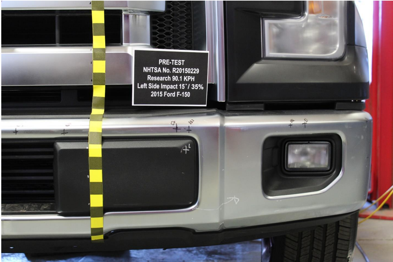
No. 202 Pre-Test Vehicle Bumper Left Front View
