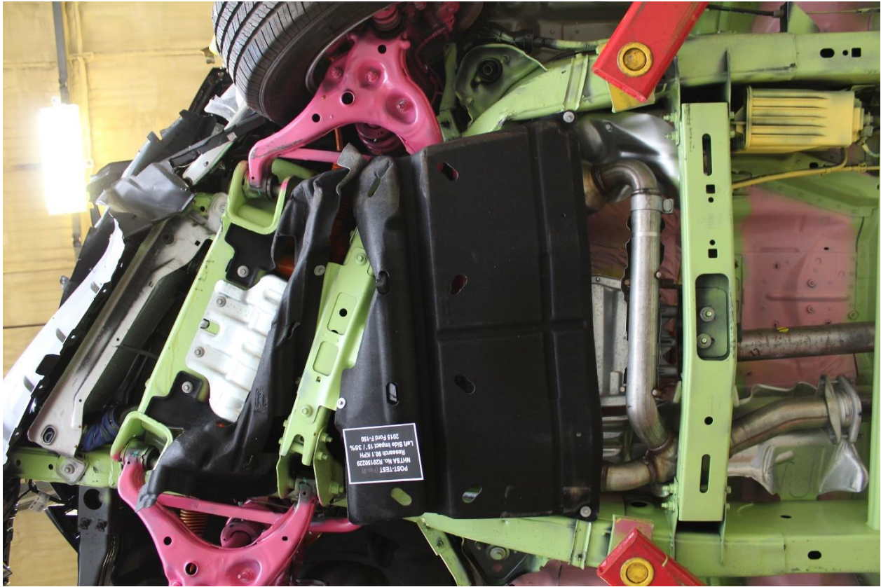
No. 144: Post-Test View of Front Sub-Frame Deformation
