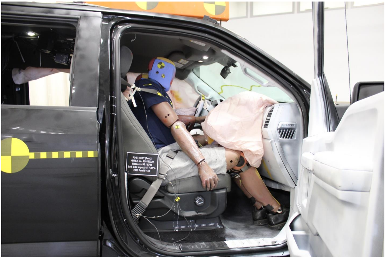
No. 101: Post-Test Right Side Passenger and Interior View
