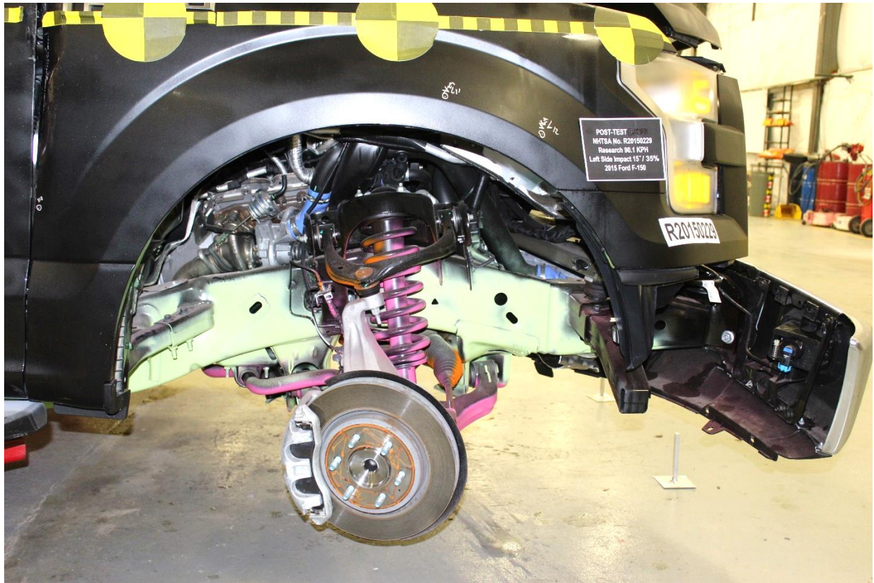
No. 155: Post-Test Side View of Front Passenger Wheel Well w/ Tire Removed
