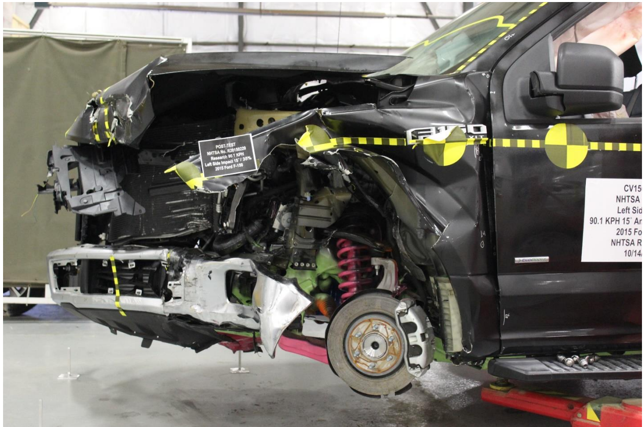
No. 149: Post-Test Side View of Front Driver Wheel Well w/ Tire Removed
