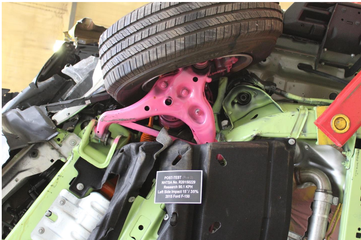
No. 146: Post-Test Frame Rail with tire removed
