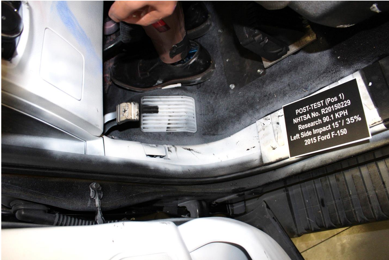
No. 165: Post-Test View of Deformation of Rocker or Post-Struck Side
