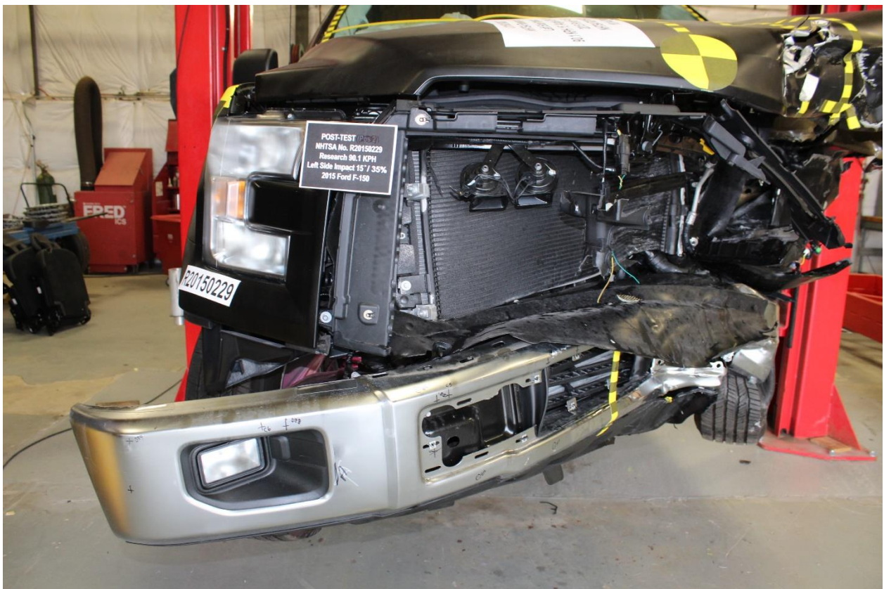
No. 205 Post-Test Vehicle Bumper Front View
