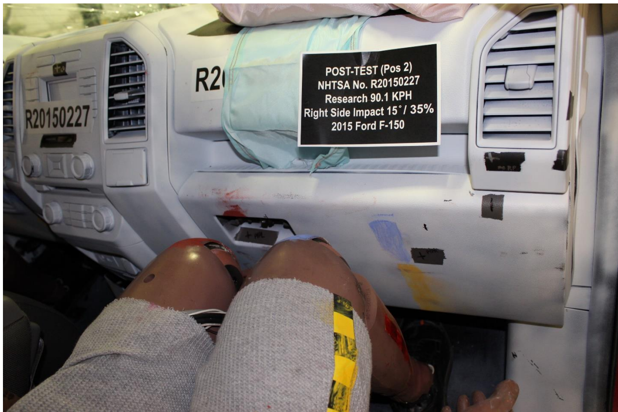
No. 123: Post-Test Passenger Contact With Glovebox
