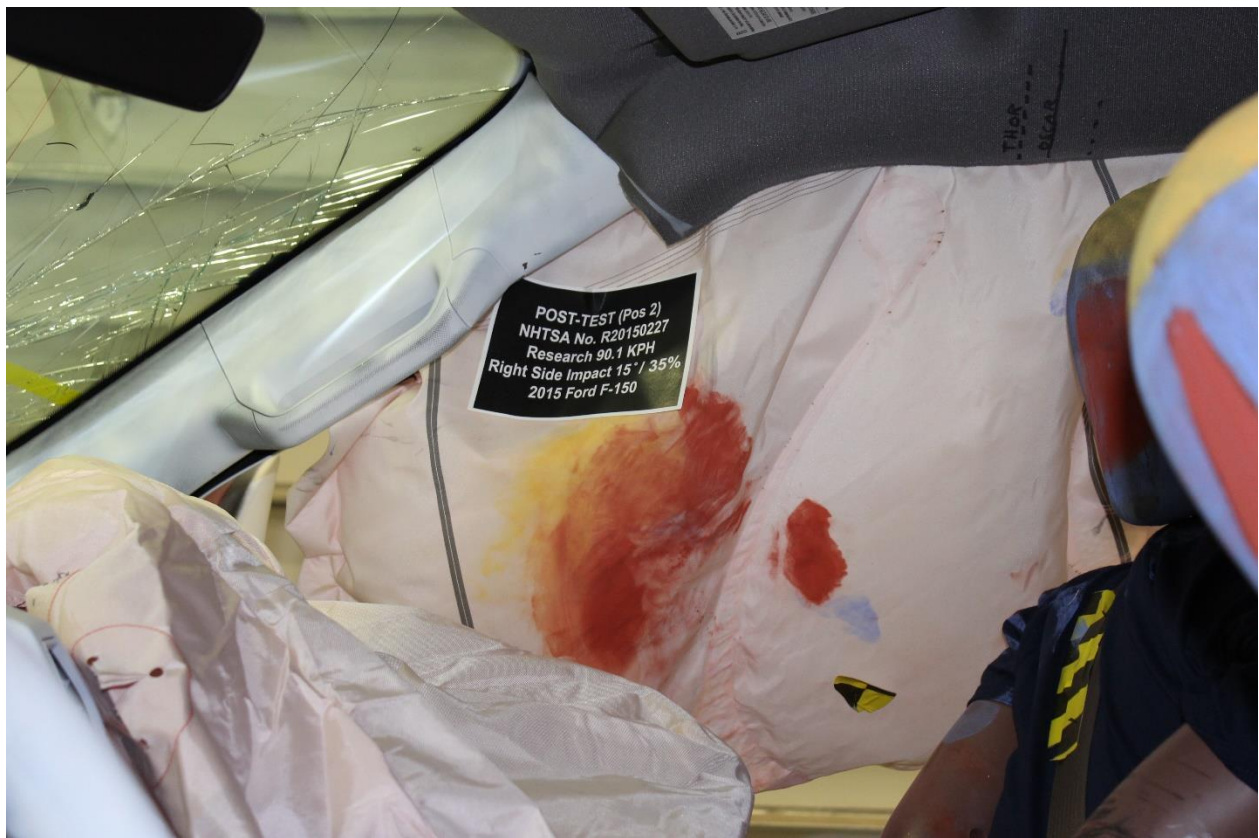
No. 119: Post-Test View of Passenger Head contact with Airbag - Curtain
