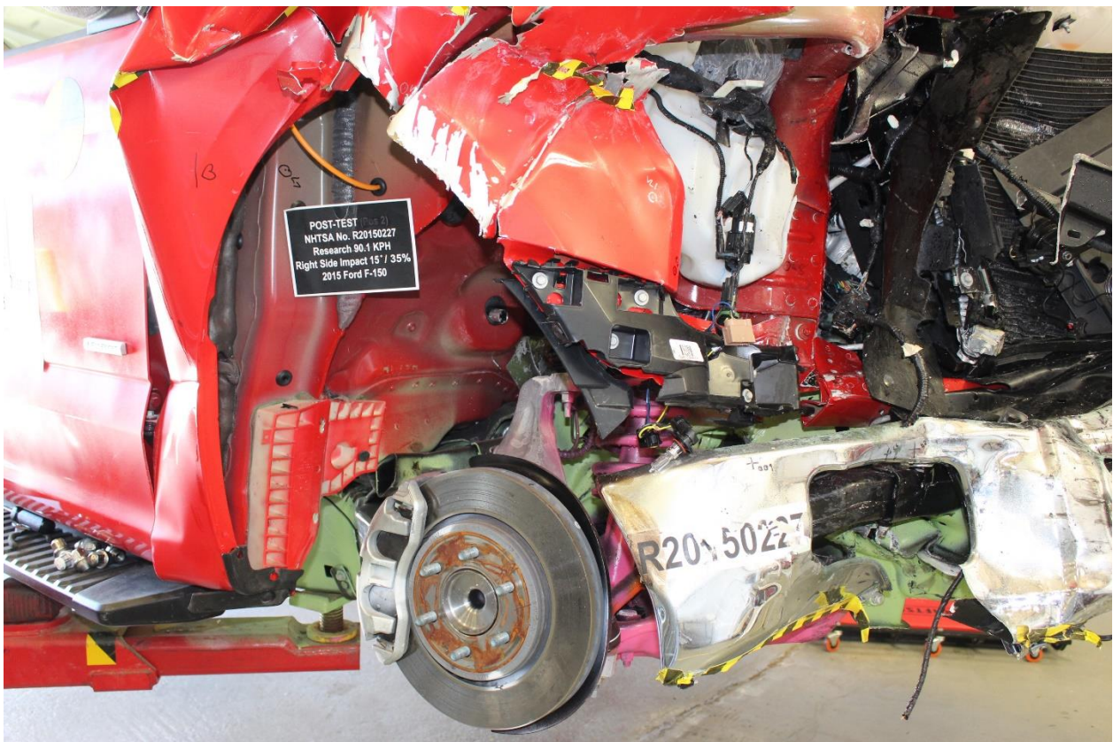
No. 154: Post-Test ¾ View of Front Passenger Wheel Well w/ Tire Removed
