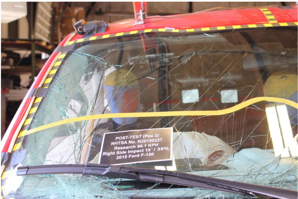
No. 095: Post-Test Passenger Front Close-up View, Windshield
