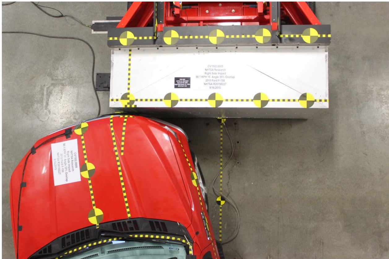
No. 022 Pre-Test Overhead View of OMDB against target vehicle at ideal Impact Point
