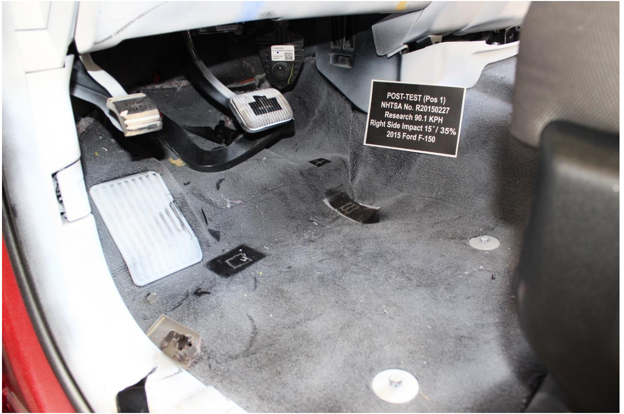
No. 045 Post-Test View of Driver Floor pan at Left sill level, w/carpet
