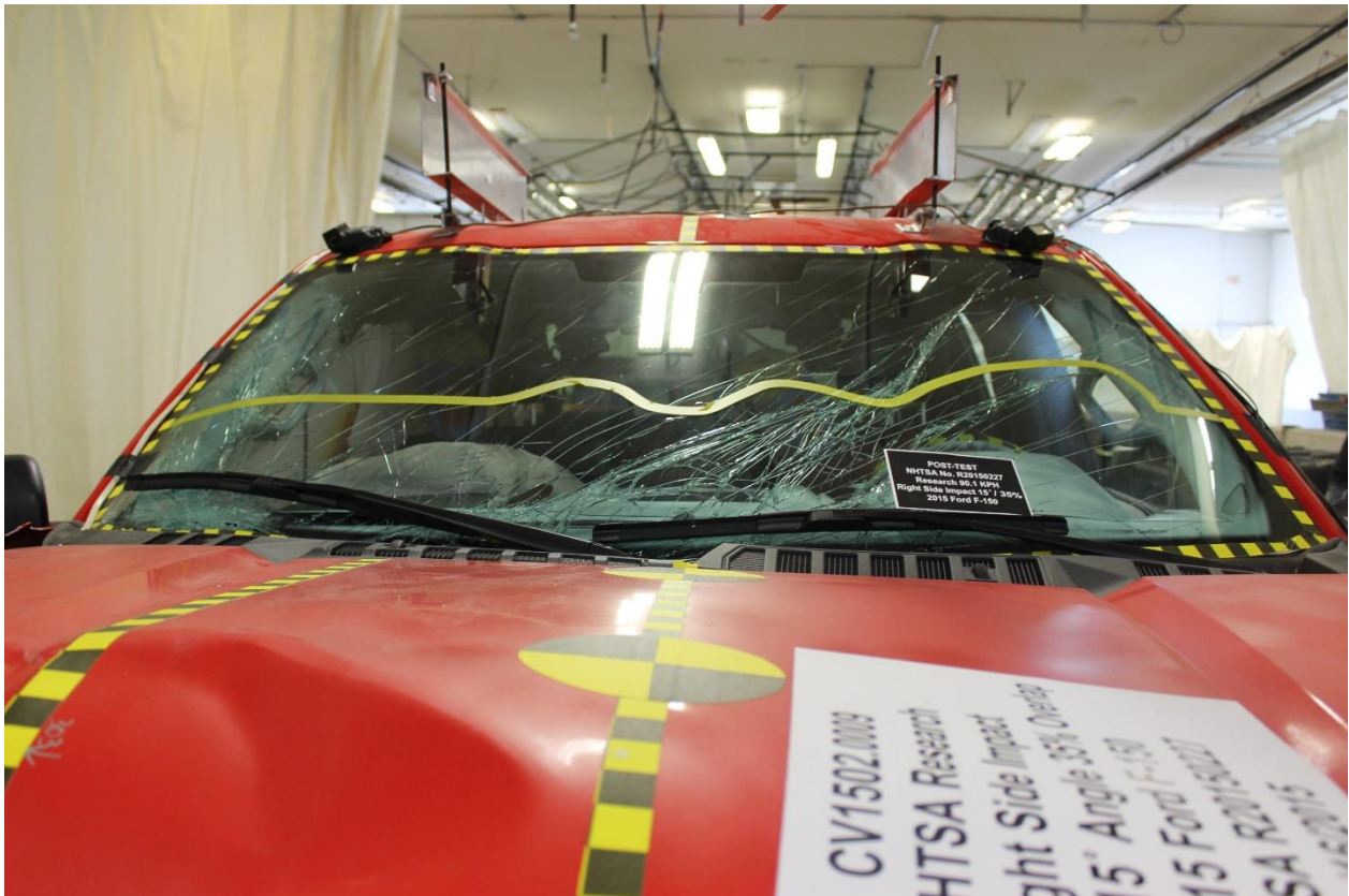
No. 166: Post-Test View of Windshield Separation
