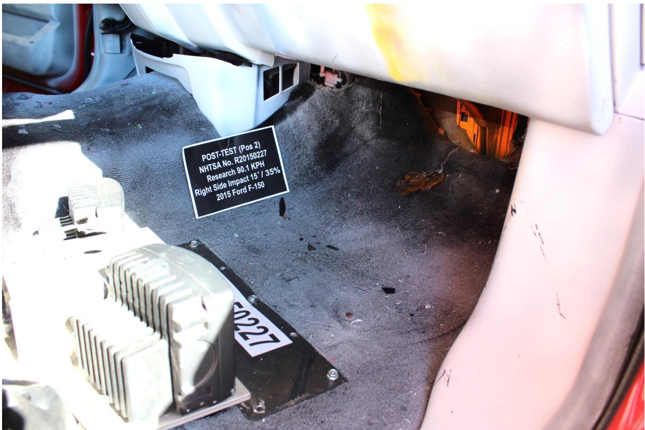
No. 089: Post-Test View of Passenger Floor pan at Right sill level, w/carpet
