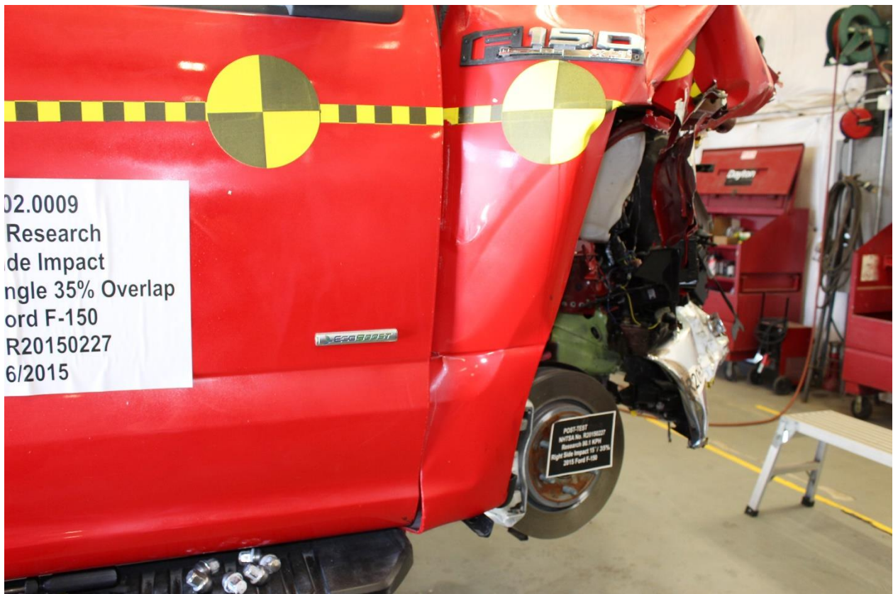
No. 156: Post-Test Right Side 3/4 Rear View of the Front Passenger Wheel Well w/ Tire Removed
