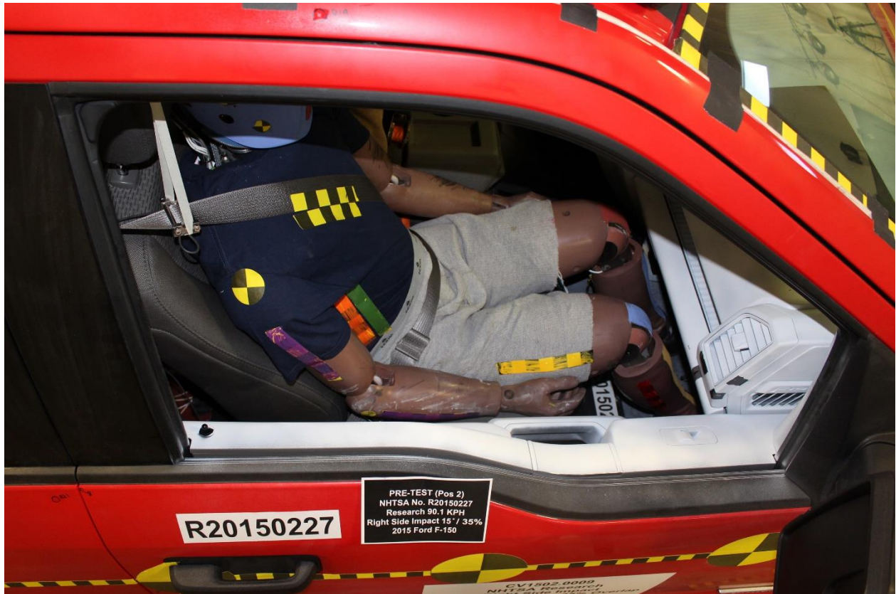
No. 102: Pre-Test View of Passenger Door Clearance
