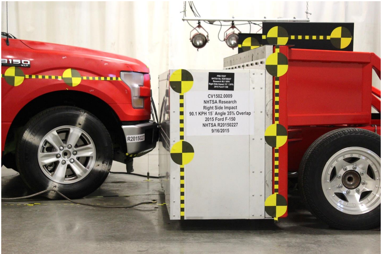
No. 023 Pre-Test Left Side View of OMDB against target vehicle at ideal Impact Point
