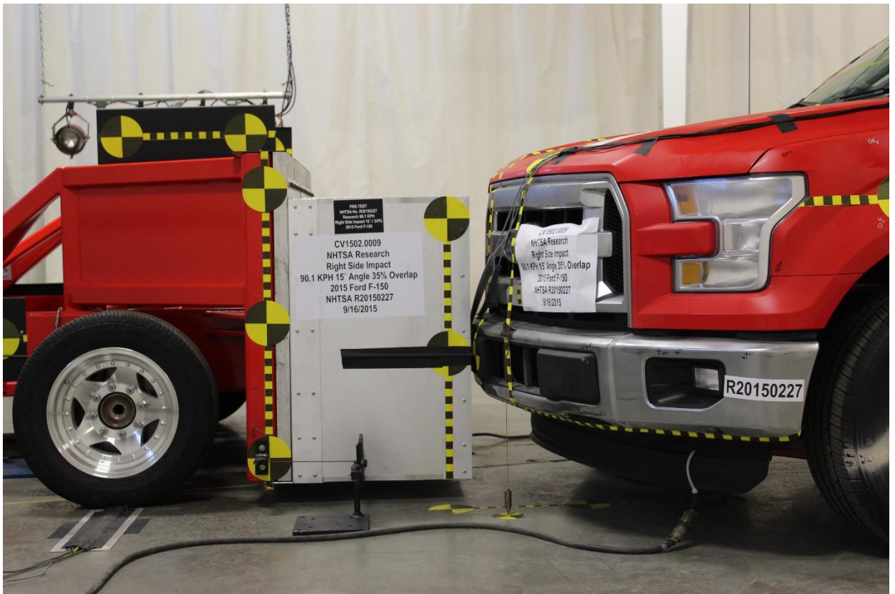
No. 024 Pre-Test Right Side View of OMDB against target vehicle at ideal Impact Point
