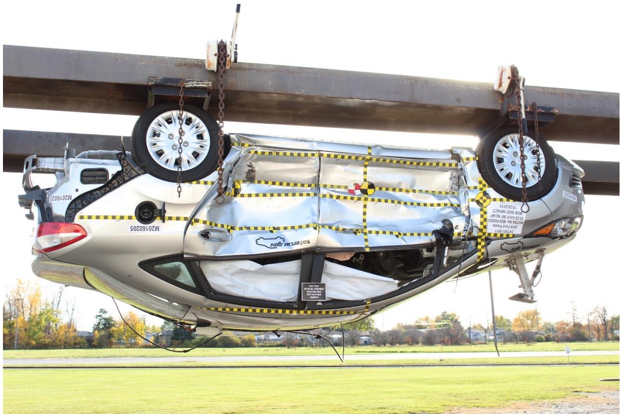
Figure A-98: FMVSS No. 301 Static Rollover 180 Degrees
