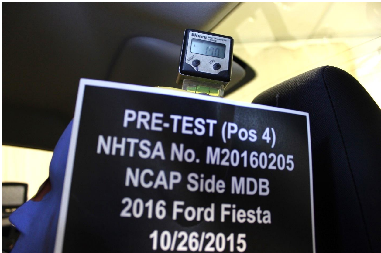
Figure A-63: Pre-Test View of Rear Passenger Dummy's Head Showing Dummy's Head Level
