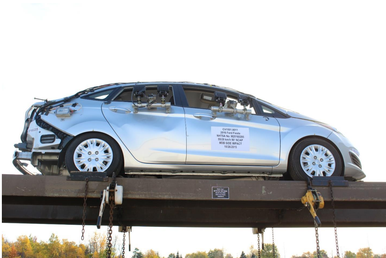
Figure A-96: FMVSS No. 301 Static Rollover 0 Degrees
