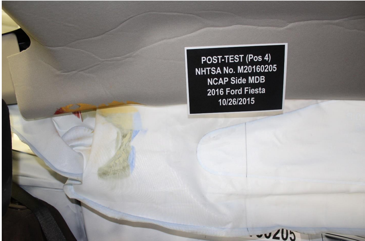
Figure A-76: Post-Test Rear Passenger Dummy Close-Up Head Contact with Side Airbag View
