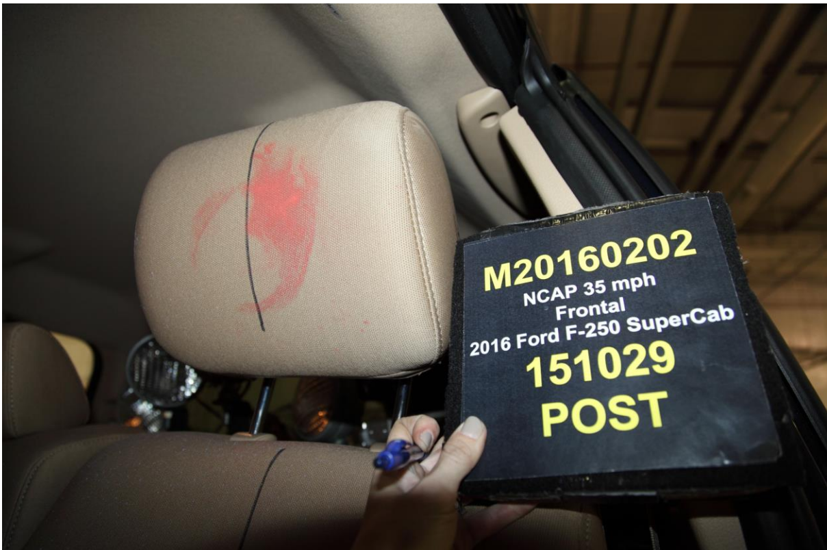
048 Post-Test Driver Dummy Contact With Headrest
