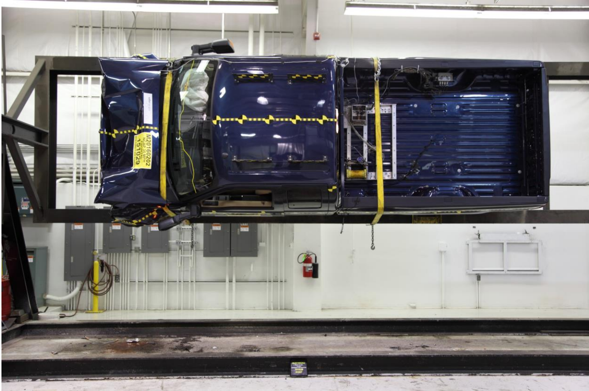
074 Vehicle at 90° on Static Rollover Device
