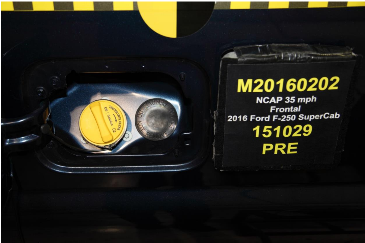
022 Pre-Test Fuel Filler Cap View
