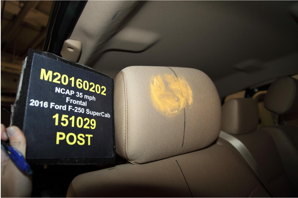
069 Post Test Passenger Dummy Contact With Headrest
