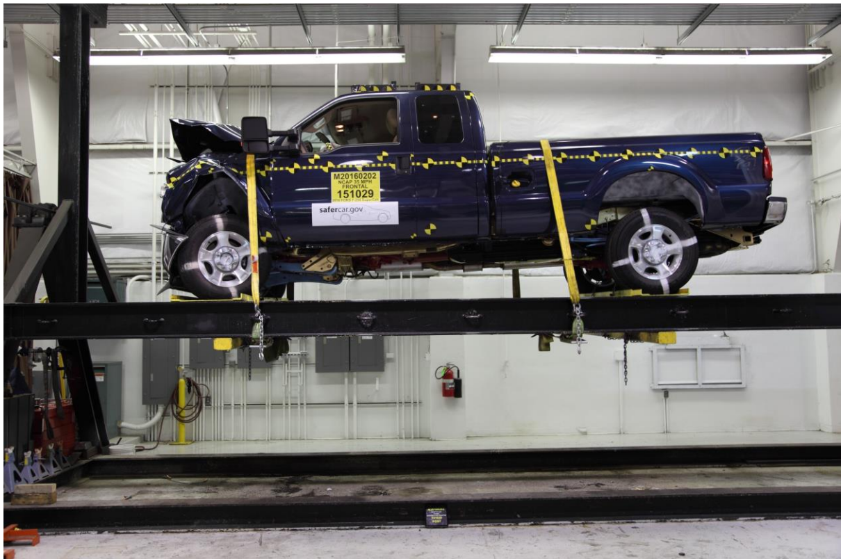
073 Vehicle at 0° on Static Rollover Device
