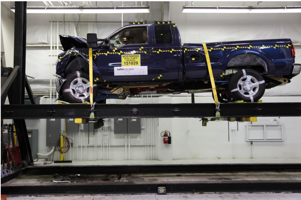
077 Vehicle at 360° on Static Rollover Device
