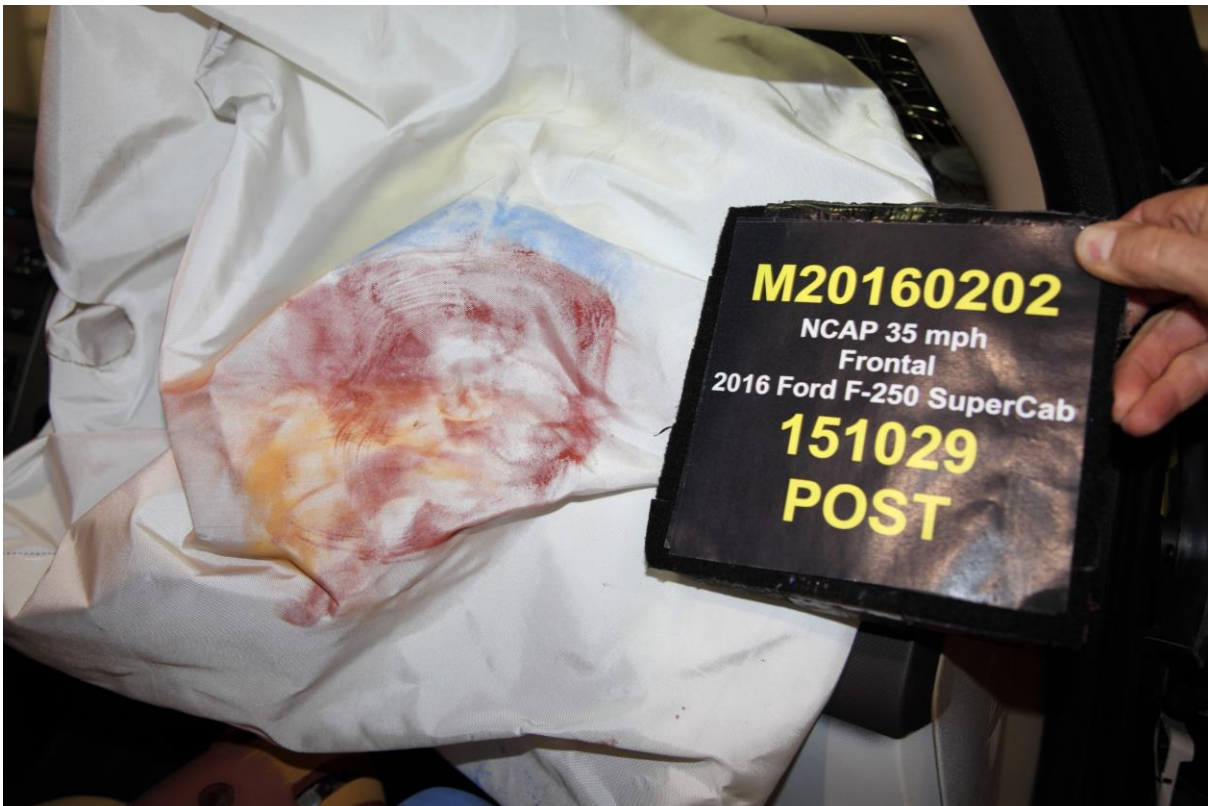
068 Post-Test Passenger Dummy Contact With Airbag
