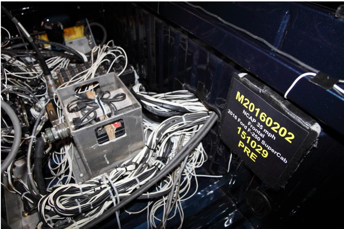
029a Pre-Test Dummy Cable Routing
