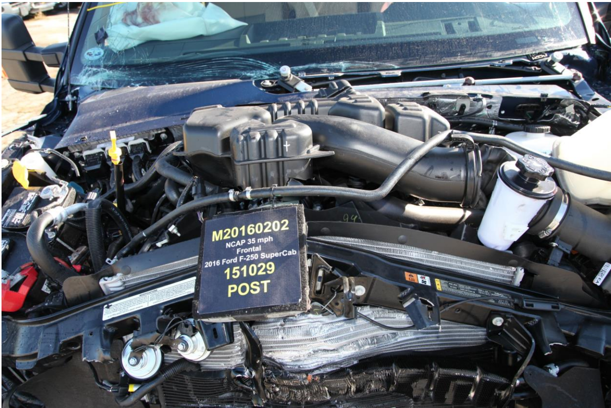
021 Post-Test Engine Compartment View
