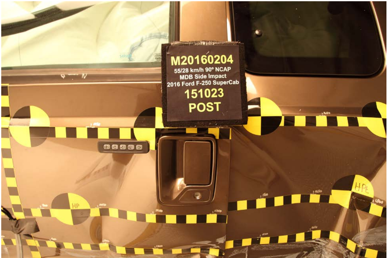
022 Post-Test Left Front Door Latch Close-up
