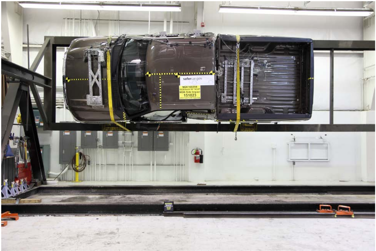
097 FMVSS No. 301 Static Rollover 90 Degrees
