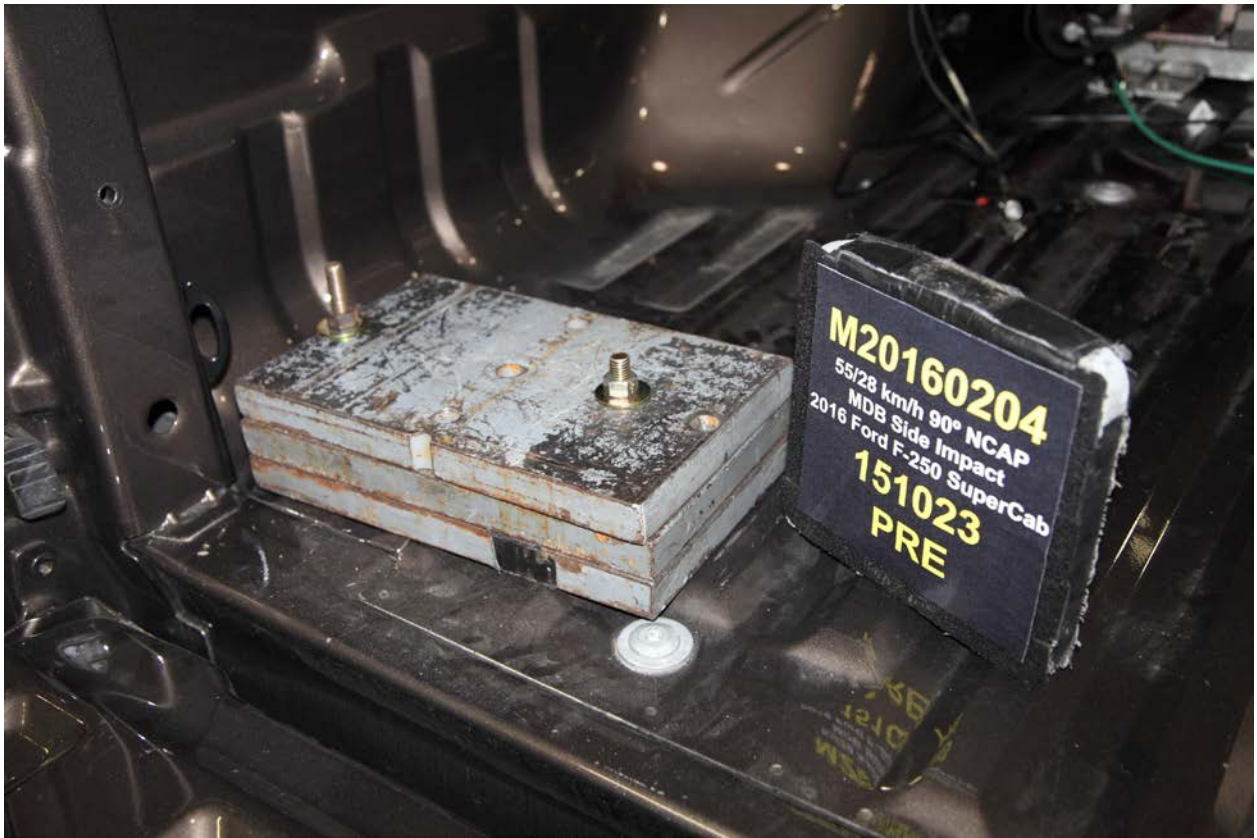
094a Pre-Test Ballast View
