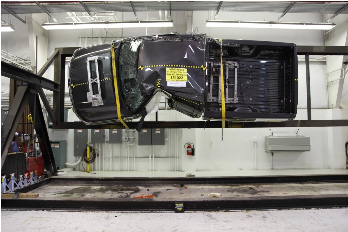
064 FMVSS No. 301 Static Rollover 90 Degrees
