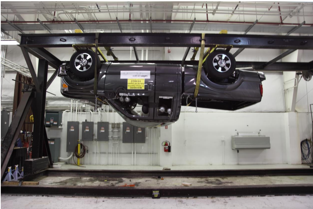
065 FMVSS No. 301 Static Rollover 180 Degrees
