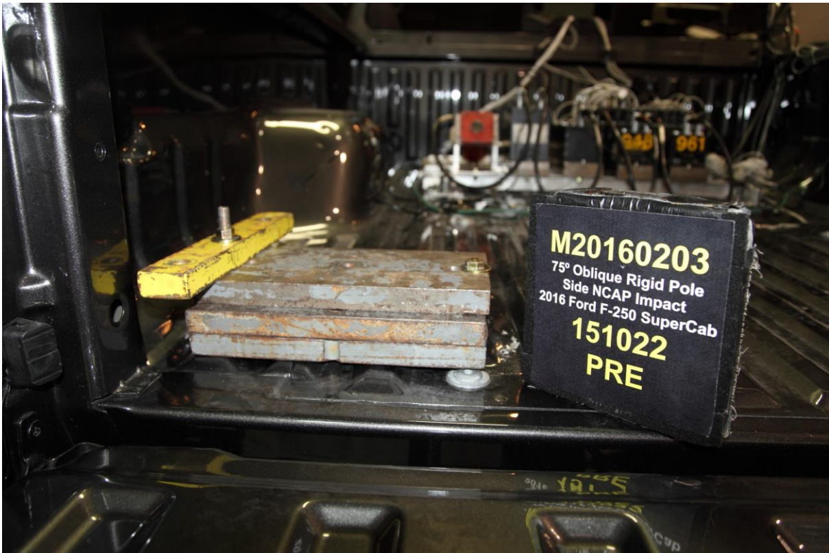
061a Pre Test Ballast View
