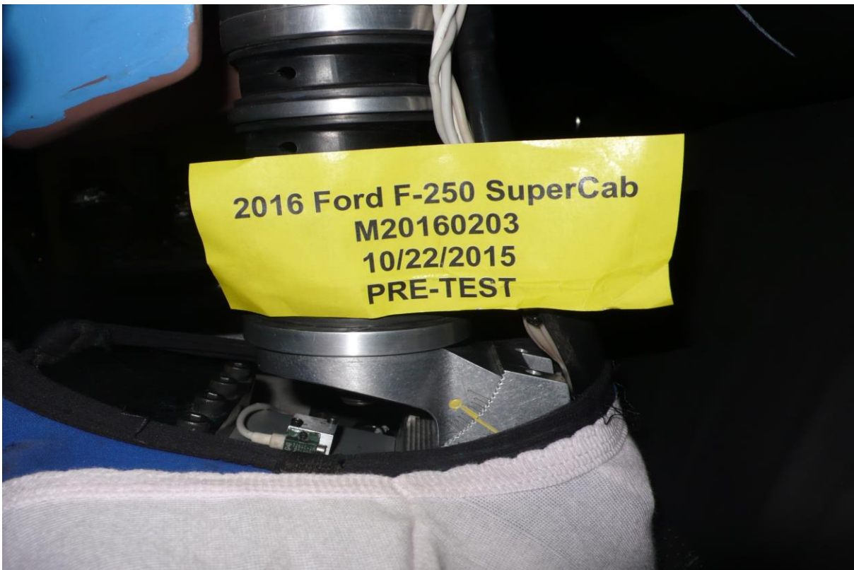
030 Pre-Test Left Side View of Dummy Neck Showing Position of Adjustable Neck Bracket
