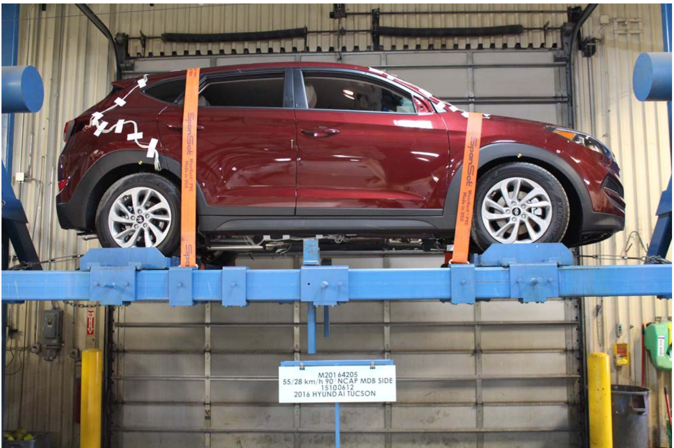
Photo No. 100 - FMVSS No. 301 Static Rollover 360 Degrees
