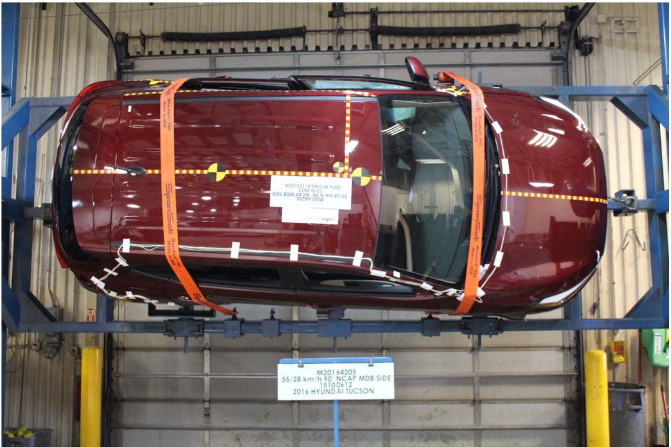
Photo No. 099 - FMVSS No. 301 Static Rollover 270 Degrees
