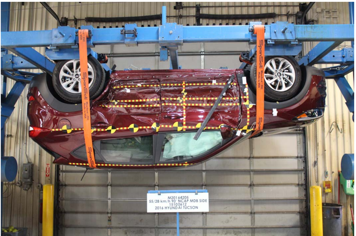
Photo No. 098 - FMVSS No. 301 Static Rollover 180 Degrees
