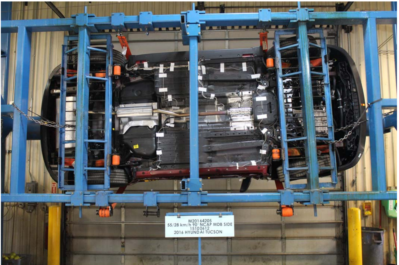
Photo No. 097 - FMVSS No. 301 Static Rollover 90 Degrees
