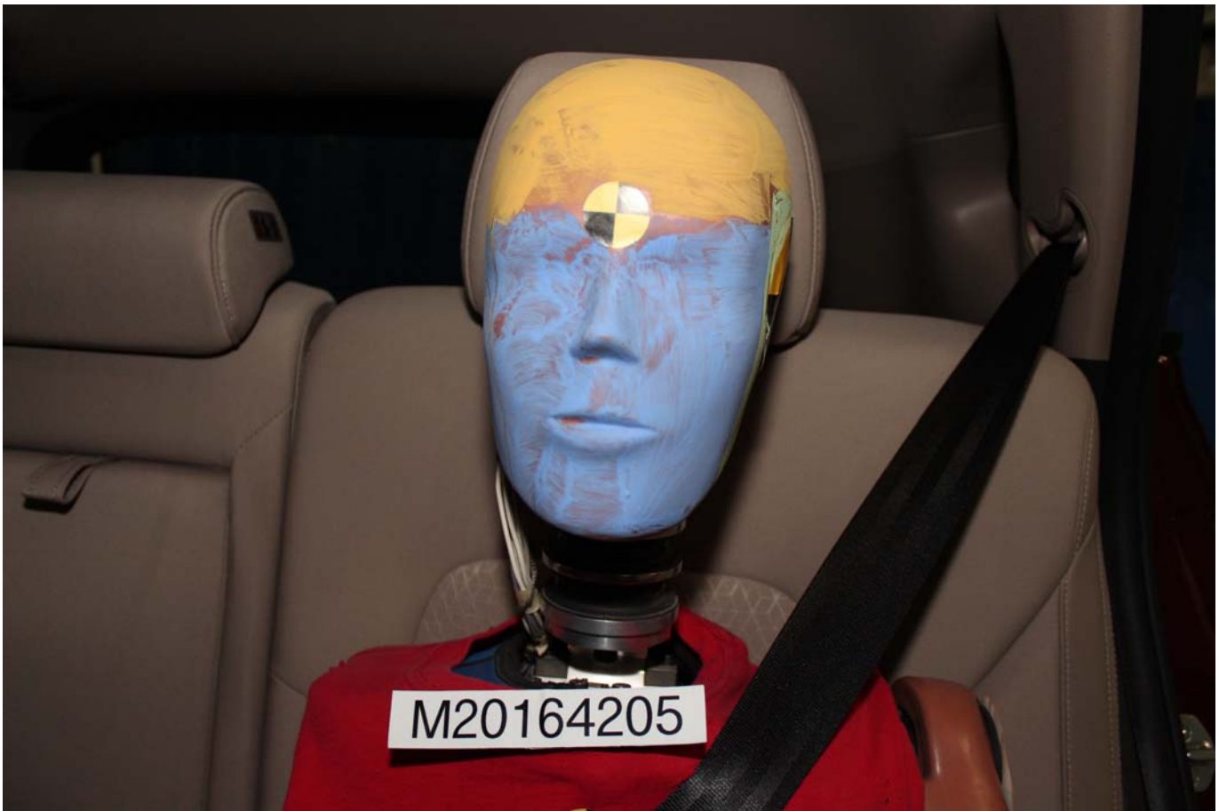
Photo No. 059 - Pre-Test Frontal View of Rear Passenger Dummy Head and Shoulders in Relation to Head Rest
