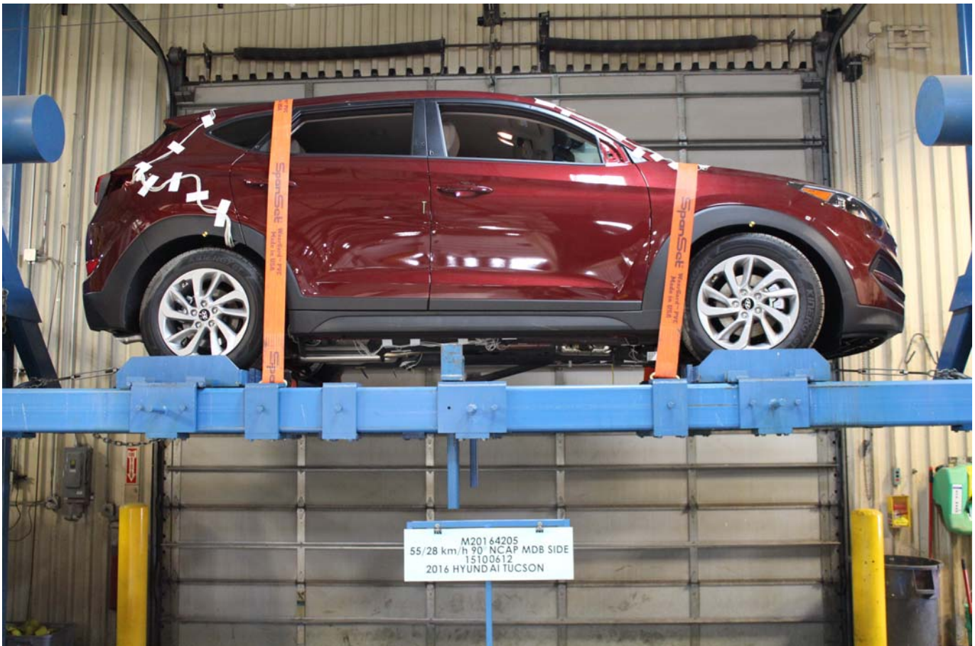
Photo No. 096 - FMVSS No. 301 Static Rollover 0 Degrees
