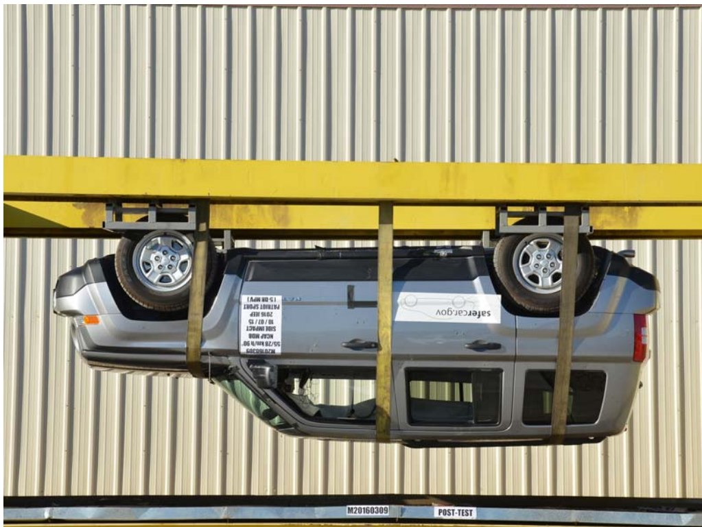
FIGURE 98. FMVSS No. 301 Static Rollover 180 Degrees
