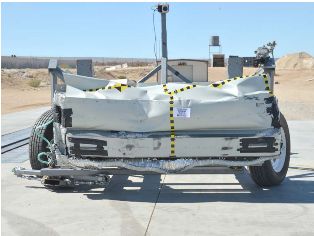
FIGURE 85. Post-Test Front View of MDB Impactor Face
