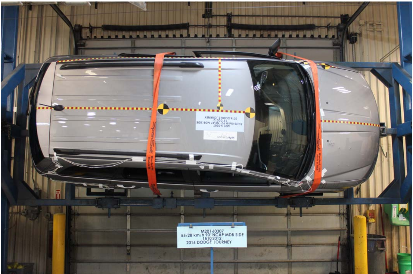
Photo No. 099 - FMVSS No. 301 Static Rollover 270 Degrees
