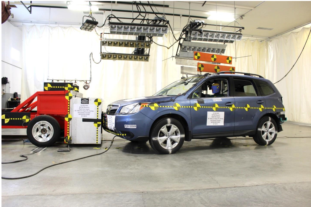
No. 183: Pre-Test OMDB & Vehicle, Right Side
