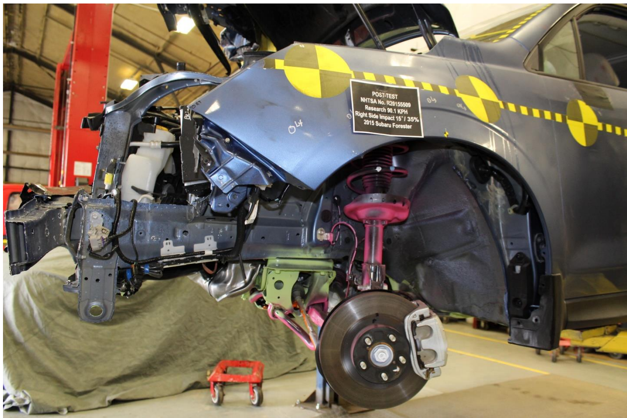
No. 148: Post-Test \frac{3}{4} View of Front Driver Wheel Well w/ Tire Removed
