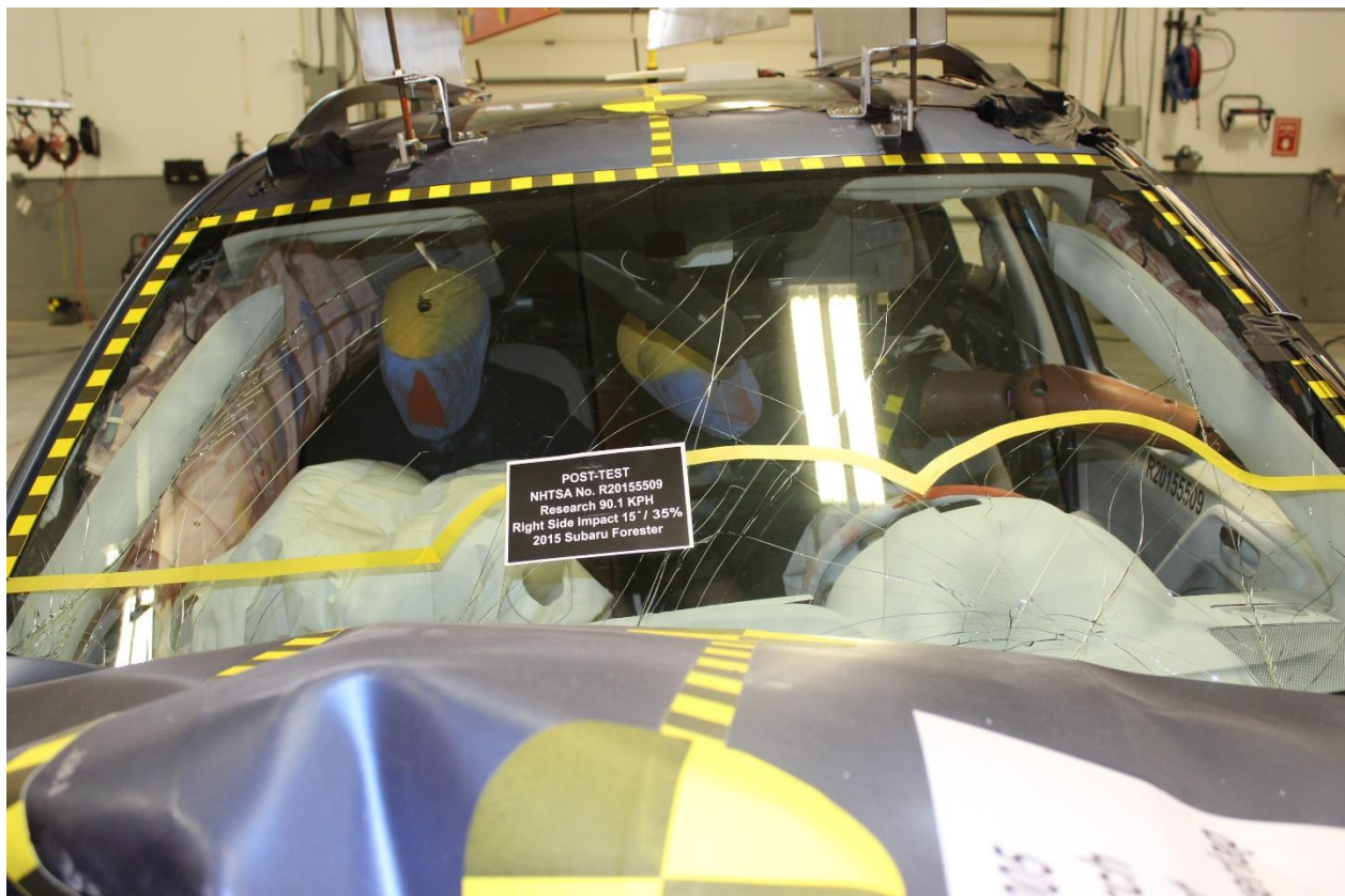
No. 166: Post-Test View of Windshield Separation
