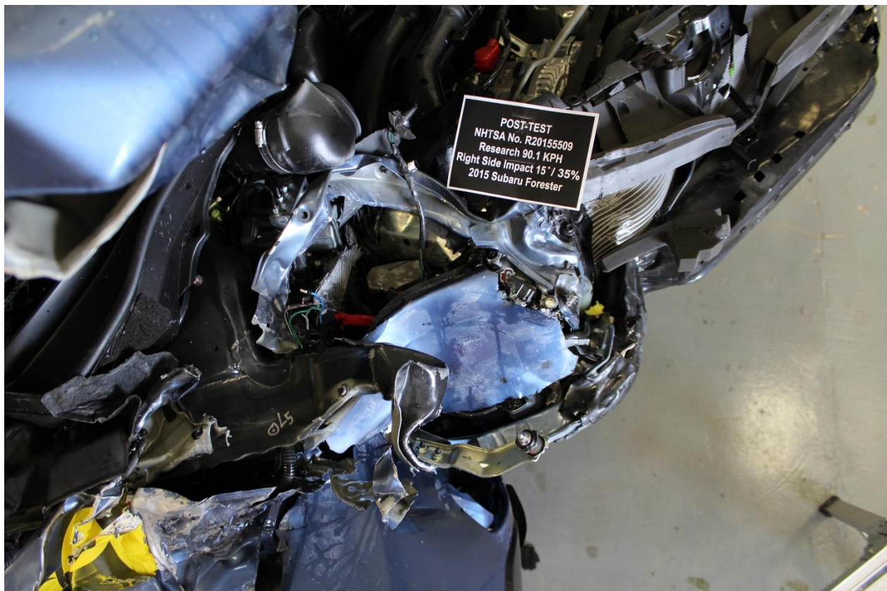
No. 131: Post-Test Right Side Engine Compartment View
