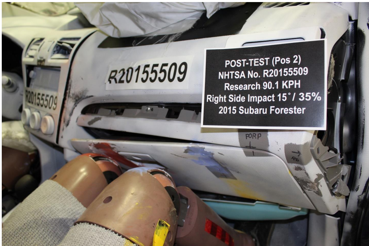
No. 123: Post-Test Passenger Contact With Glovebox
