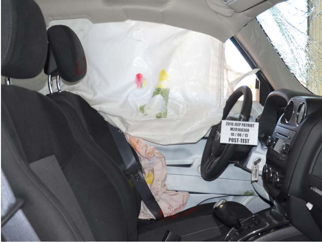
FIGURE 45. Post-Test Inner Door Panel View Showing Dummy Contact Locations
