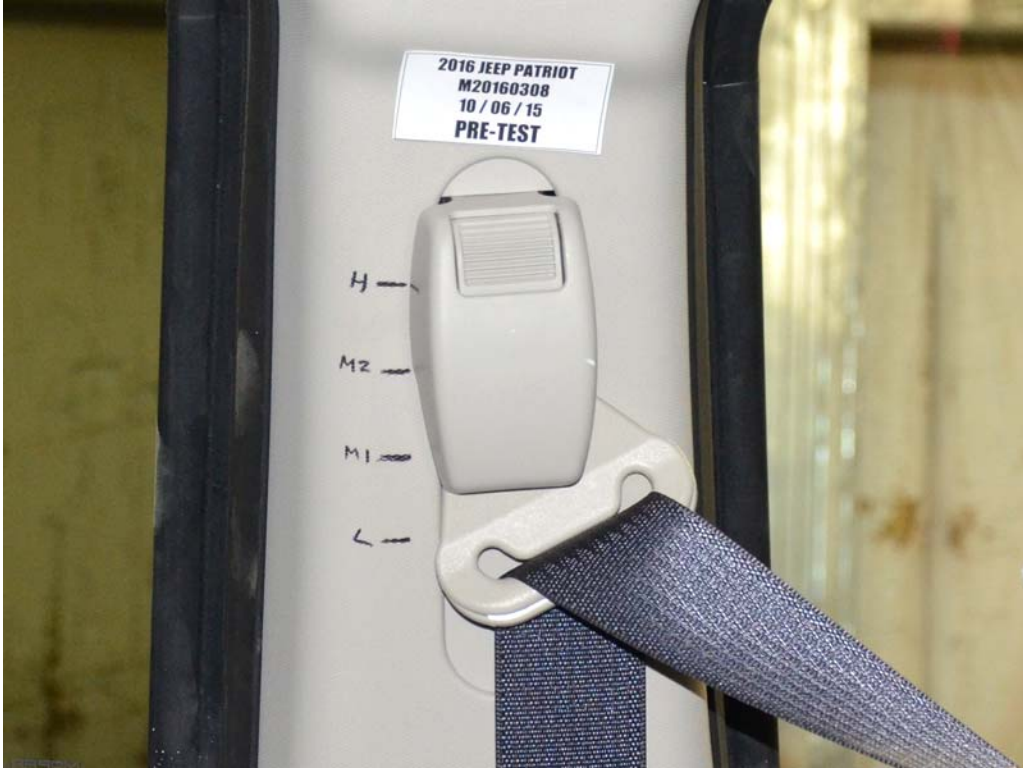
FIGURE 33. Pre-Test View of Belt Anchorage for Dummy
