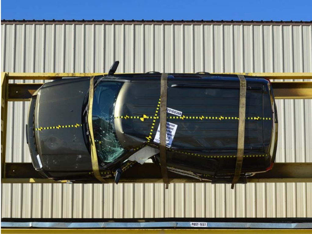
FIGURE 64. FMVSS No. 301 Static Rollover 90 Degrees
