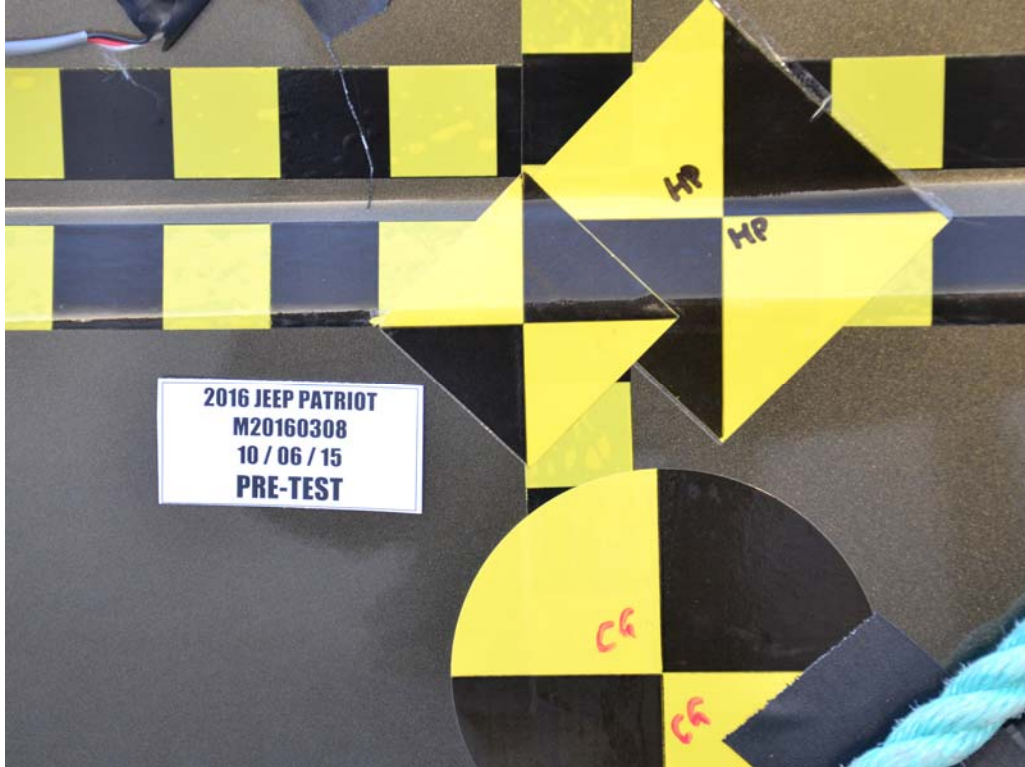
FIGURE 19. Pre-Test Close-Up View of Impact Point Target
