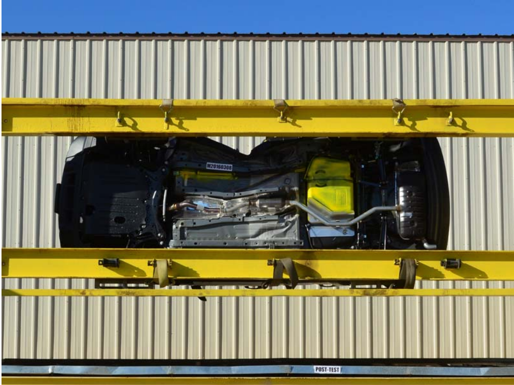
FIGURE 66. FMVSS No. 301 Static Rollover 270 Degrees
