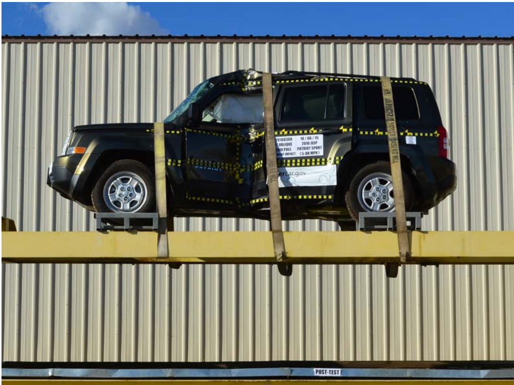
FIGURE 67. FMVSS No. 301 Static Rollover 360 Degrees
