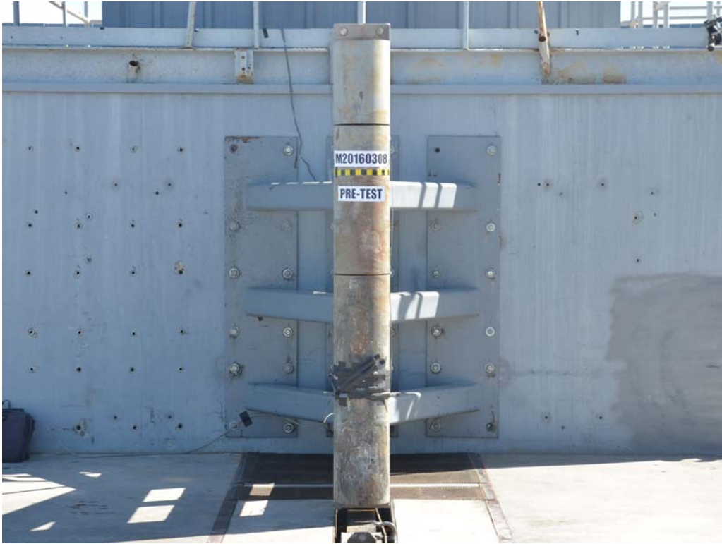
FIGURE 57. Pre-Test Pole Barrier Front View
