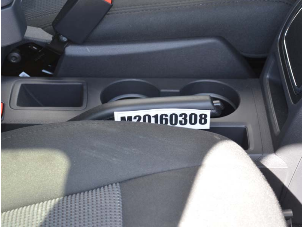
FIGURE 35. View of Disengaged Parking Brake
