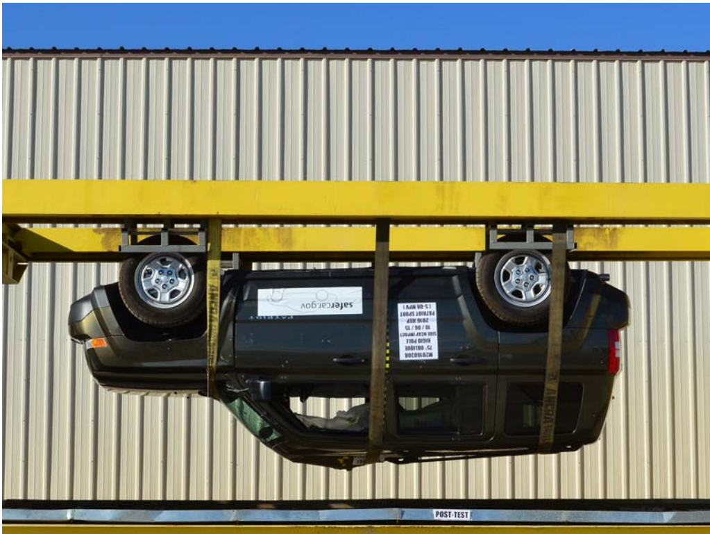
FIGURE 65. FMVSS No. 301 Static Rollover 180 Degrees
