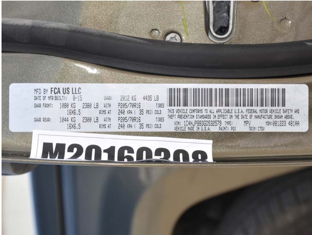
FIGURE 55. Close-Up View of Vehicle's Certification Label
