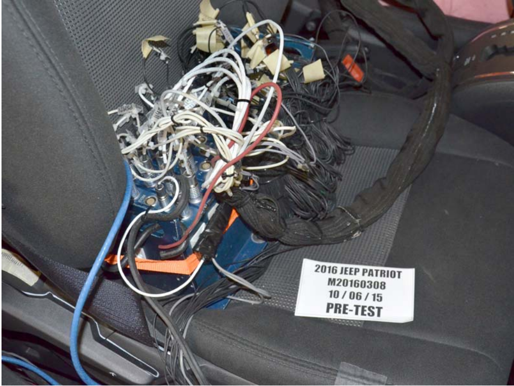
FIGURE 61. Pre-Test Ballast View
