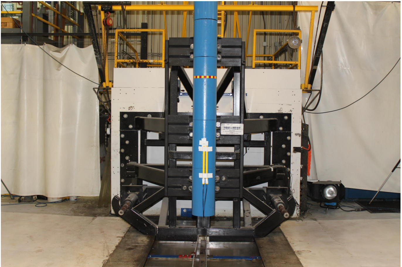
Photo No. 057 - Pre-Test Pole Barrier Front View
