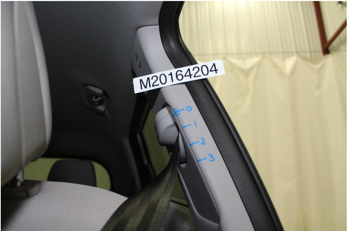
Photo No. 033 - Pre-Test View of Belt Anchorage for Dummy
