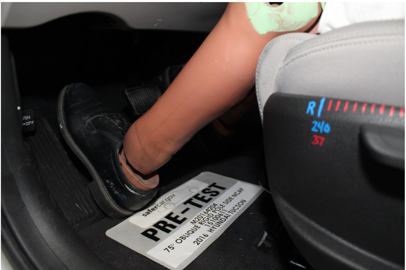
Photo No. 032 - Pre-Test Placement of Dummy's Feet
