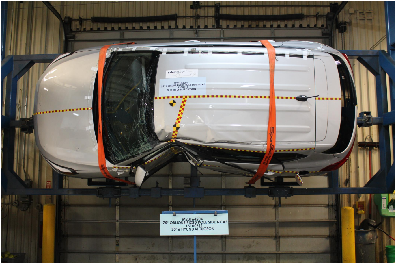
Photo No. 064 - FMVSS No. 301 Static Rollover 90 Degrees
