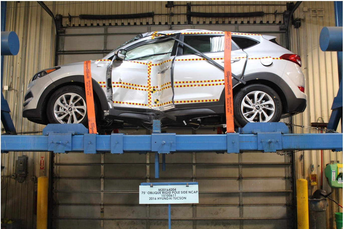
Photo No. 067 - FMVSS No. 301 Static Rollover 360 Degrees
