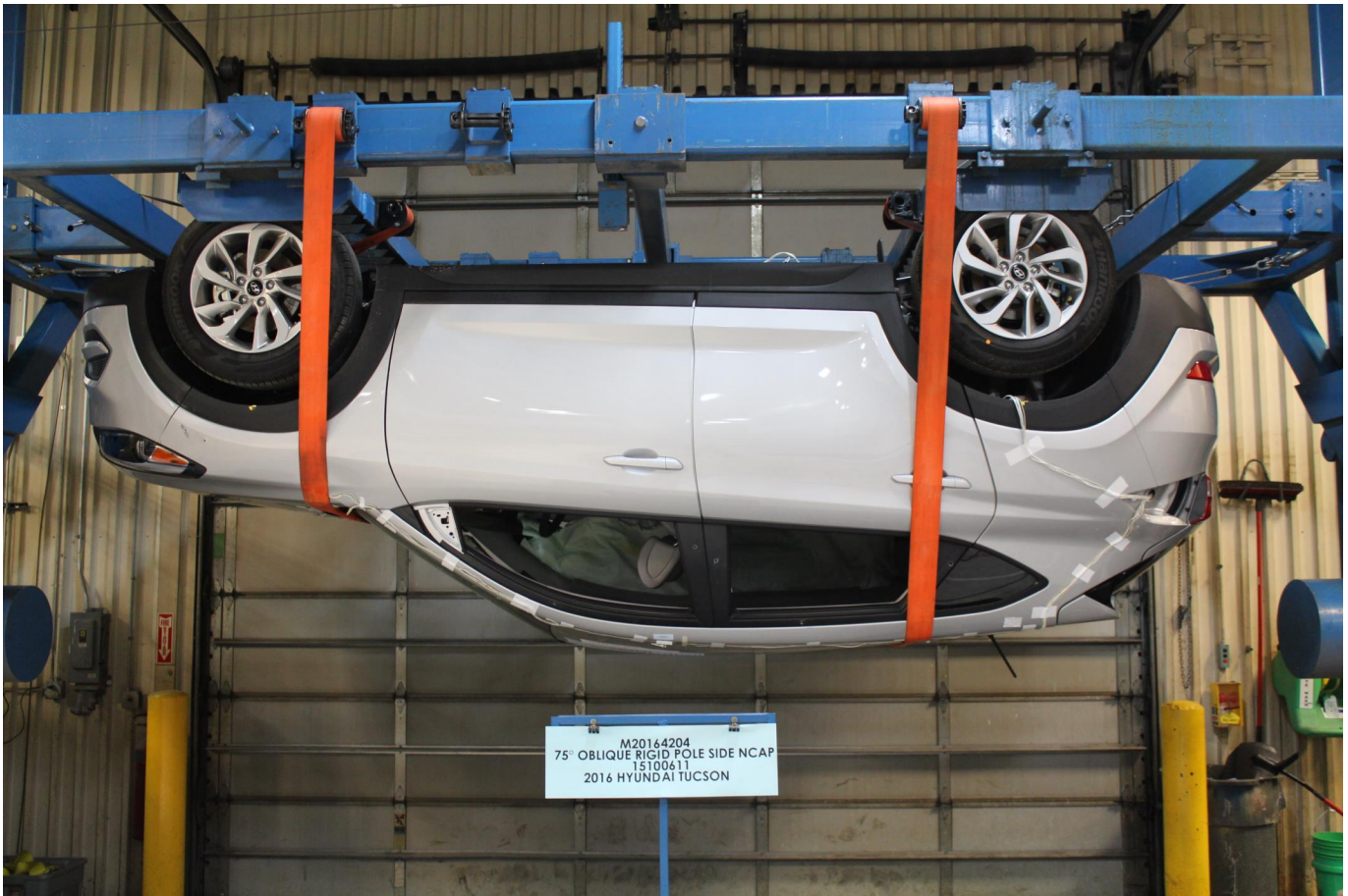
Photo No. 065 - FMVSS No. 301 Static Rollover 180 Degrees
