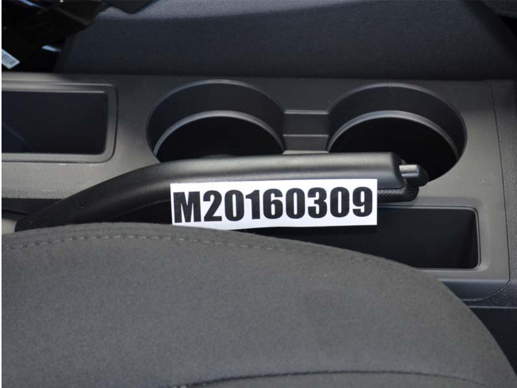
FIGURE 37. View of Disengaged Parking Brake
