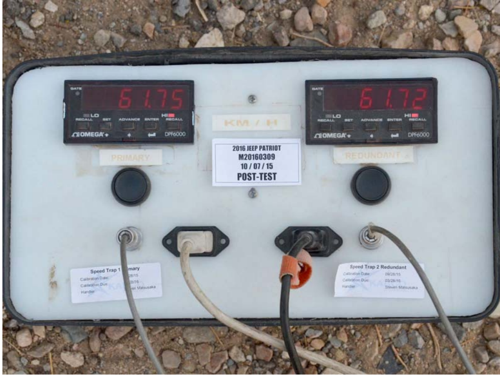
FIGURE 95. Post-Test Primary and Redundant Speed Trap Read-Out
