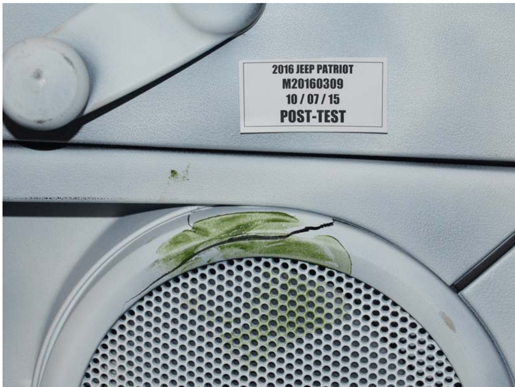
FIGURE 54. Post-Test Driver Dummy Close-Up Knee Contact View
