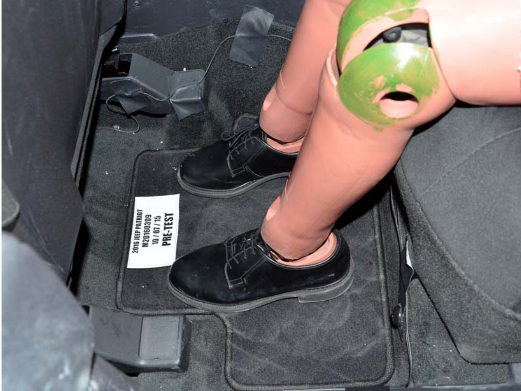
FIGURE 64. Pre-Test Placement of Rear Passenger Dummy's Feet
