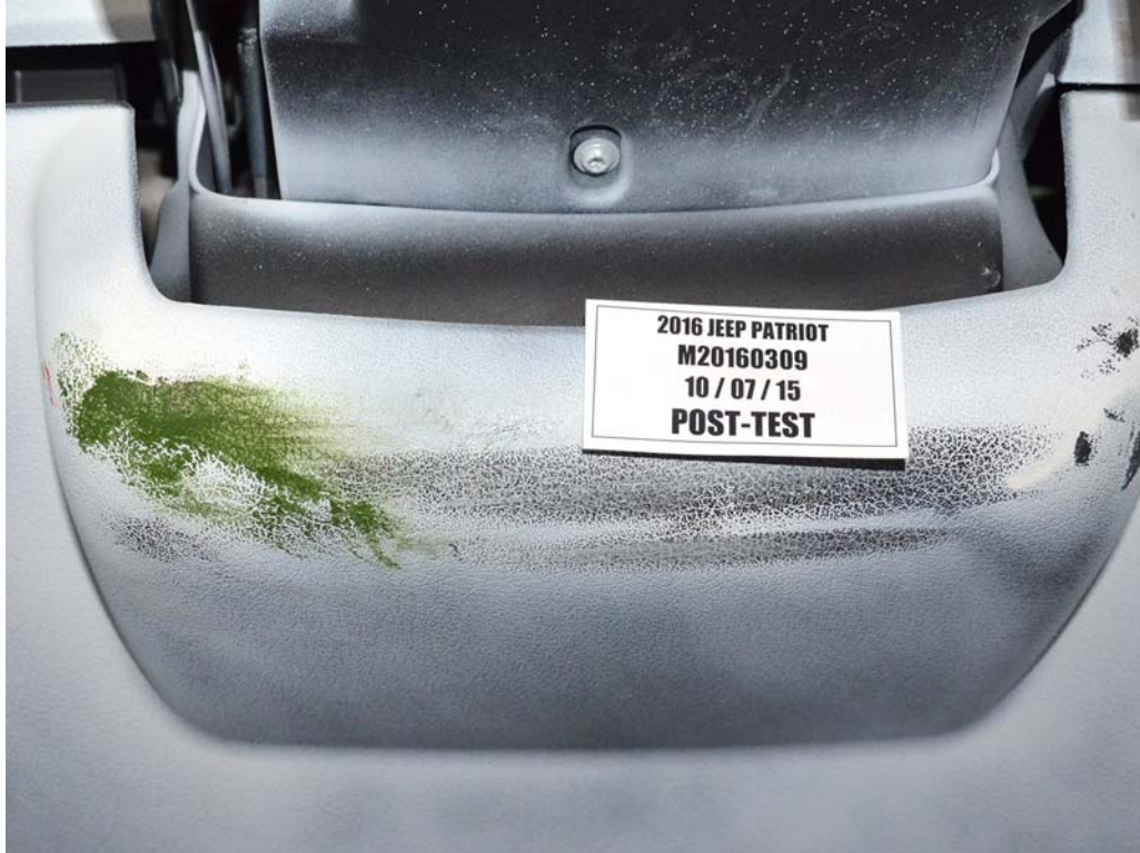
FIGURE 54a. Post-Test Driver Dummy Close-Up Knee Contact View
