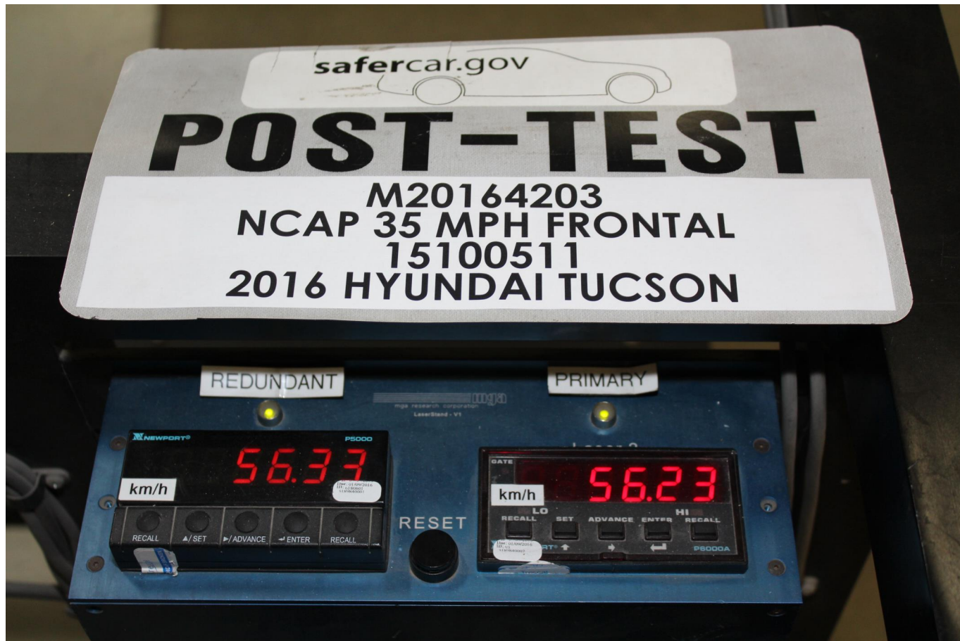
Photo No. 071 - Post-Test Speed Trap Read-Out
