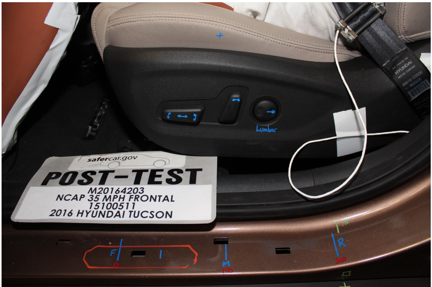
Photo No. 036 - Post-Test Driver's Seat Fore-Aft Markings
