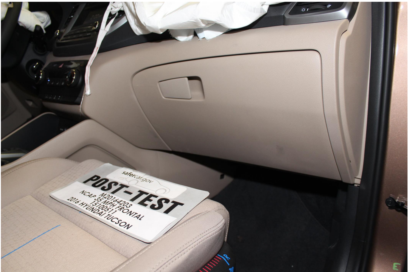
Photo No. 063 - Post-Test Passenger Side Knee Bolster (without dummy)
