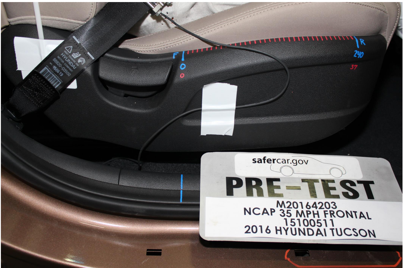
Photo No. 056 - Pre-Test Passenger's Seat Fore-Aft Markings
