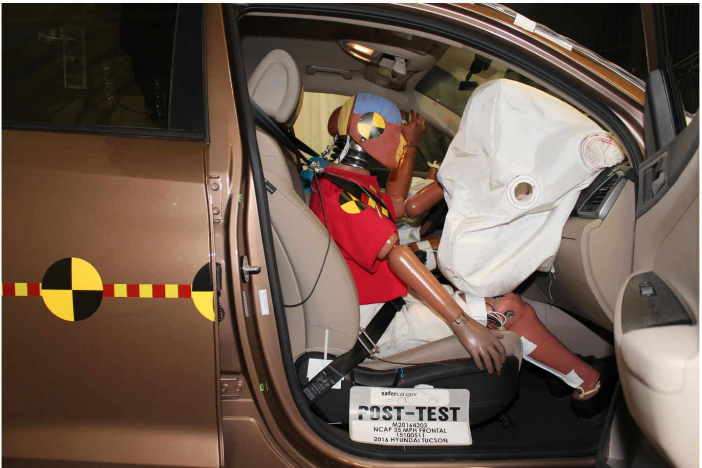
Photo No. 055 - Post-Test Passenger Dummy and Vehicle Interior (Door Open)
