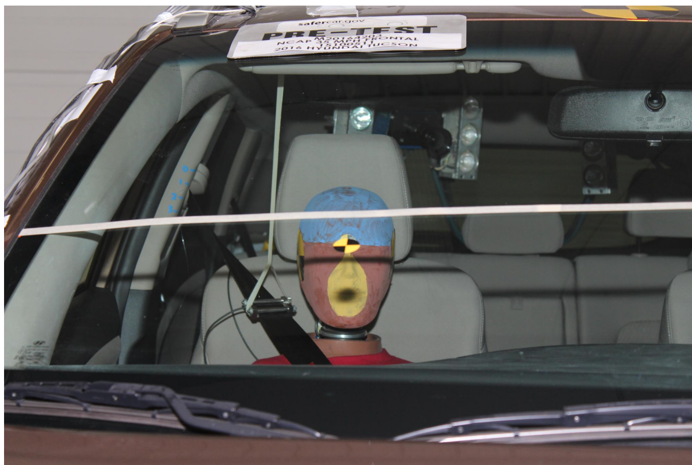
Photo No. 050 - Pre-Test Passenger Dummy Front View
