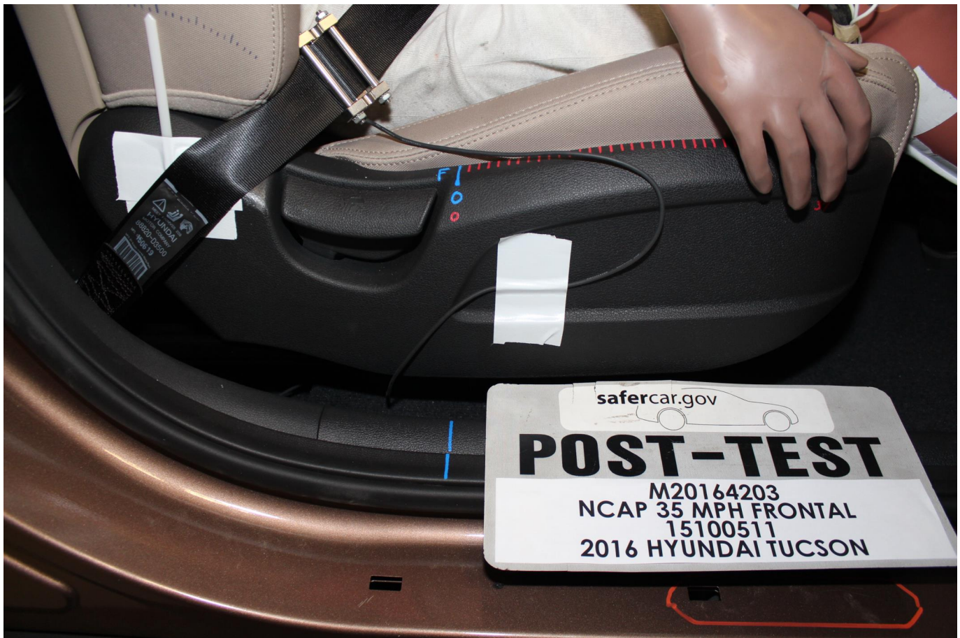
Photo No. 057 - Post-Test Passenger's Seat Fore-Aft Markings
