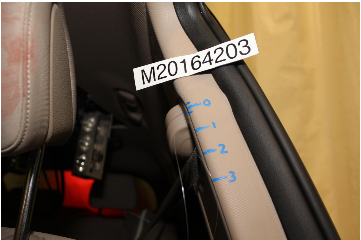
Photo No. 038 - Post-Test View of Belt Anchorage for Driver Dummy
