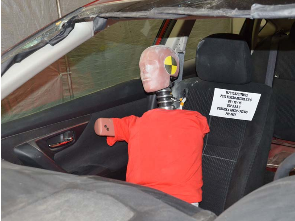
FIGURE 9. Pre-Test Dummy Position, ¾ View
