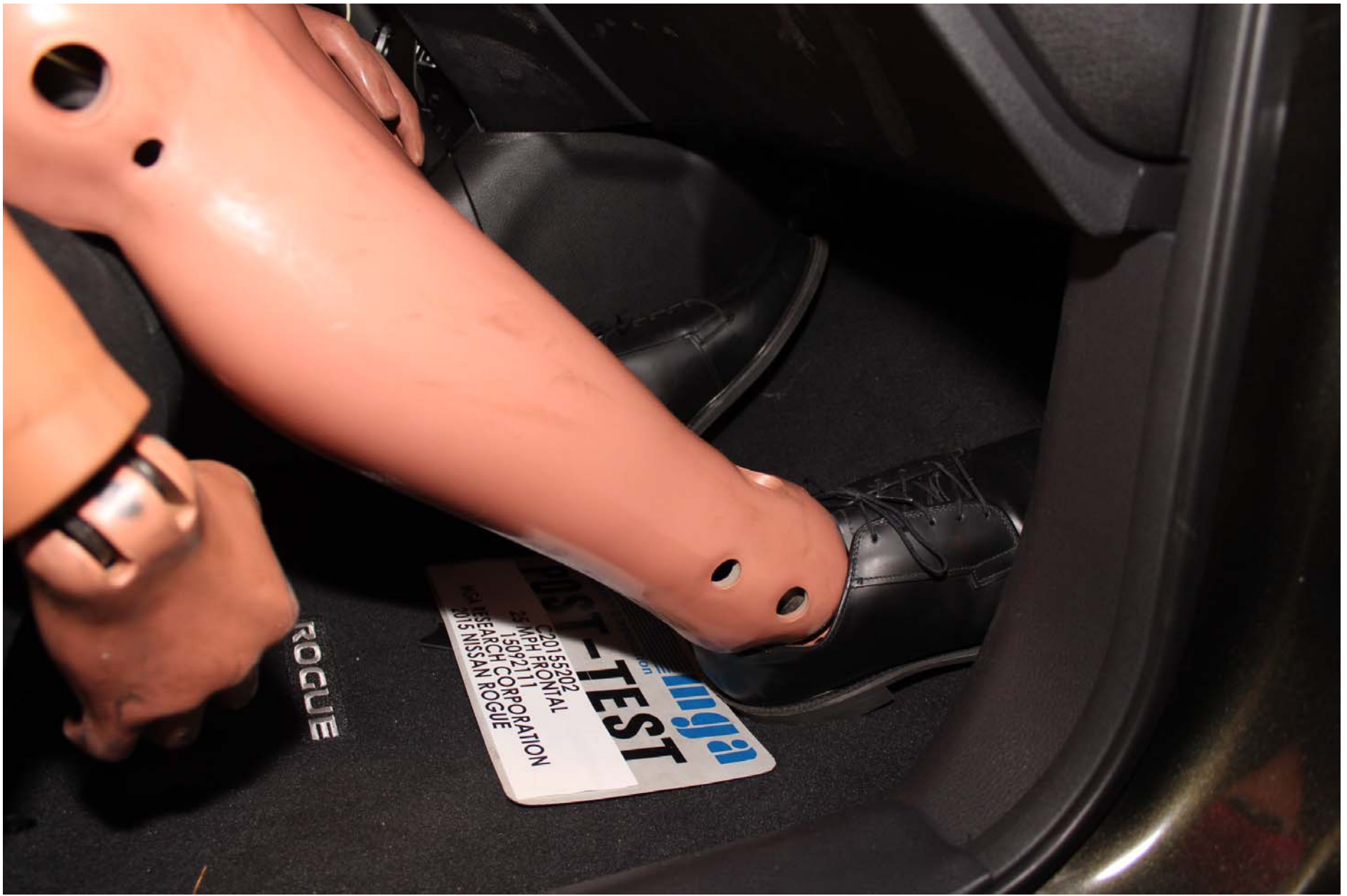
Photo No. 57 - Post-Test Passenger Dummy Feet Position
