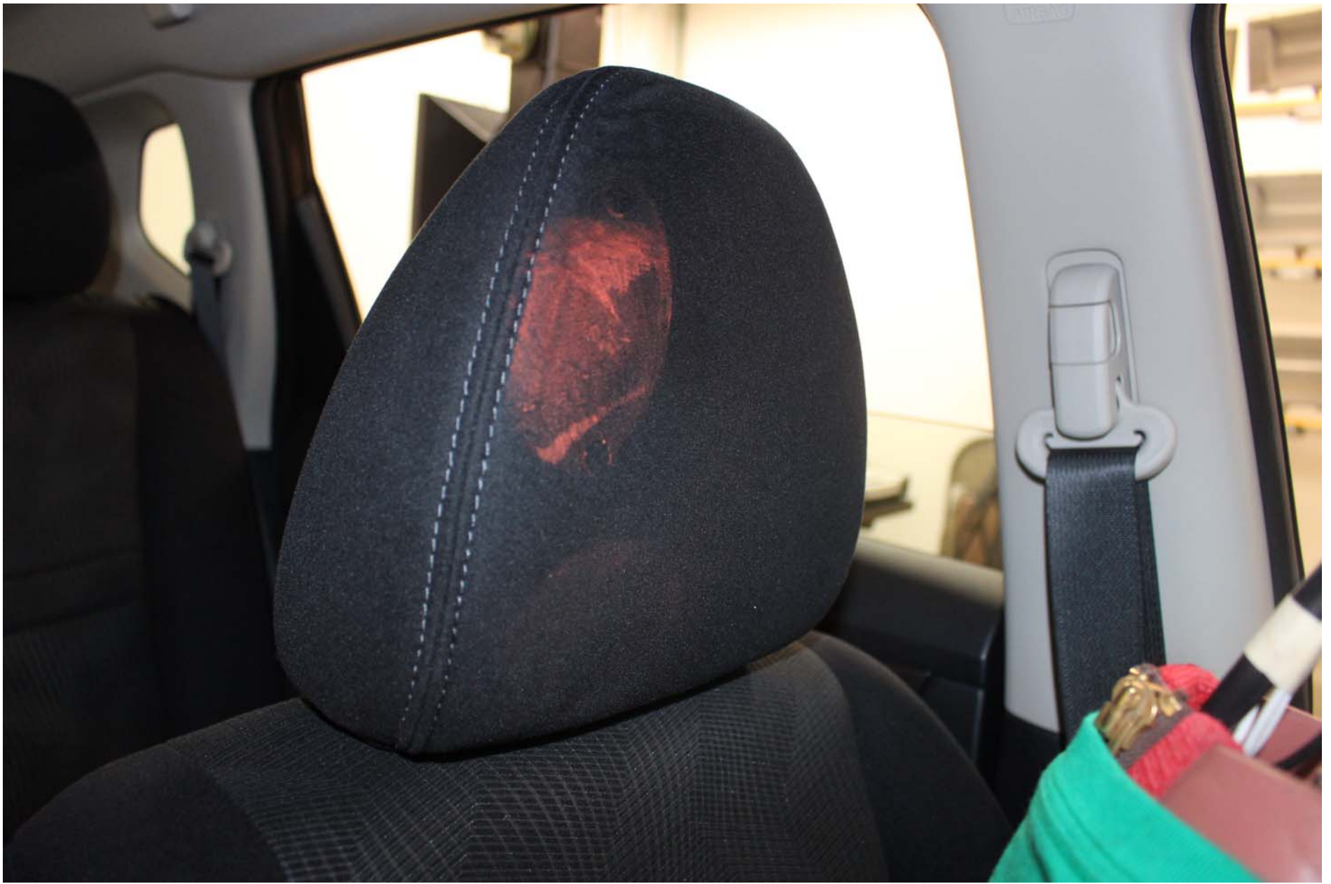
Photo No. 14 - Post-Test 5th Fem. P2 Driver Dummy Head Contact (headrest)
