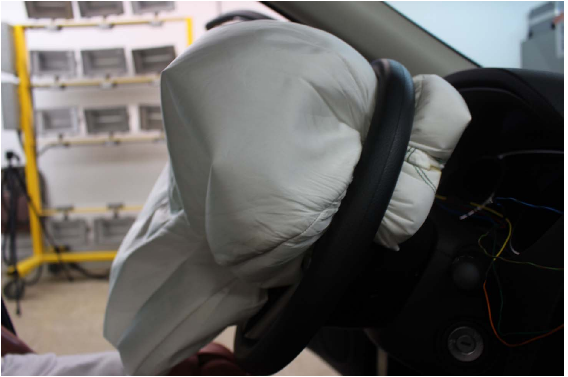
Photo No. 13 - Post-Test 5th Fem. P2 Driver Dummy Airbag Right Side View
