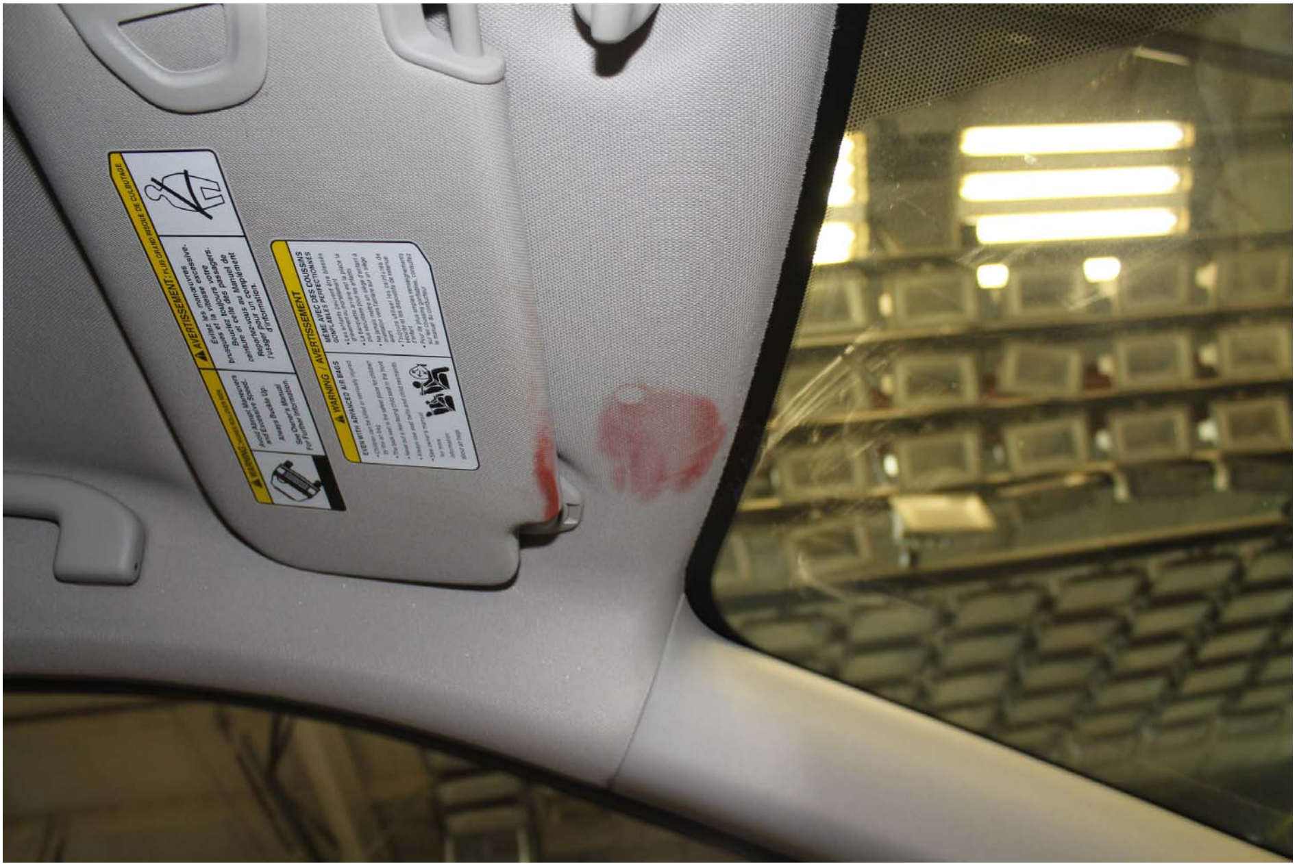
Photo No. 46 - Post-Test Driver Dummy Head Contact (visor)
