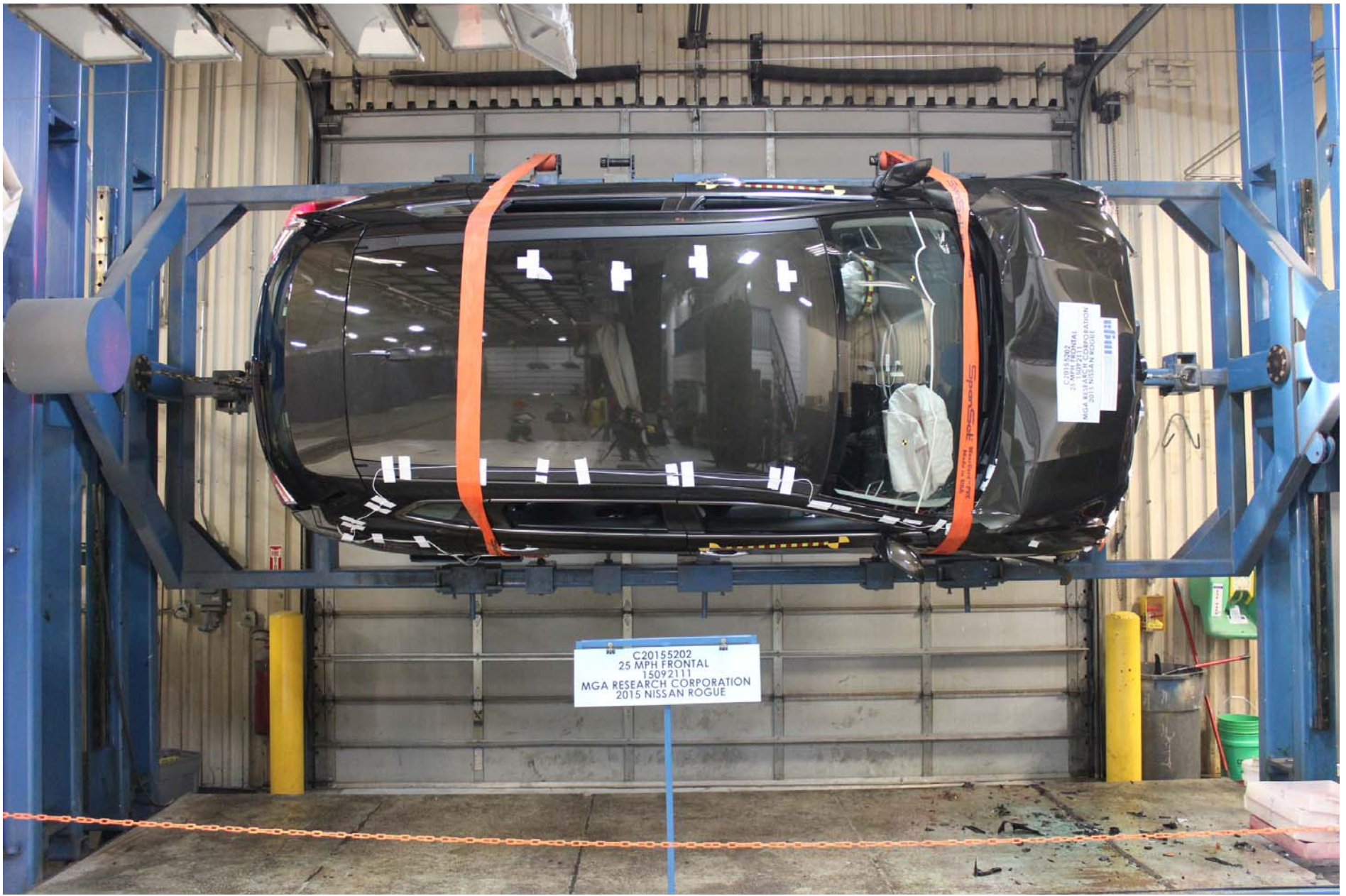
Photo No. 62 - Rollover 90 Degrees
