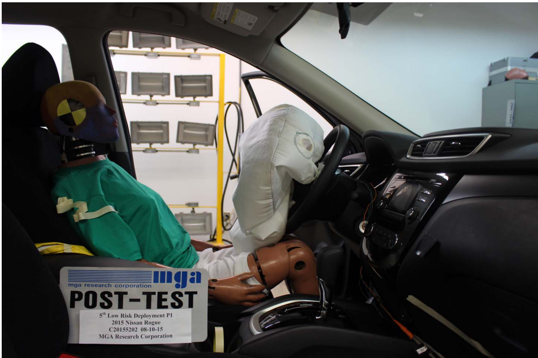
Photo No. 4 - Post-Test 5th Fem. P1 Driver Dummy Right Side View
