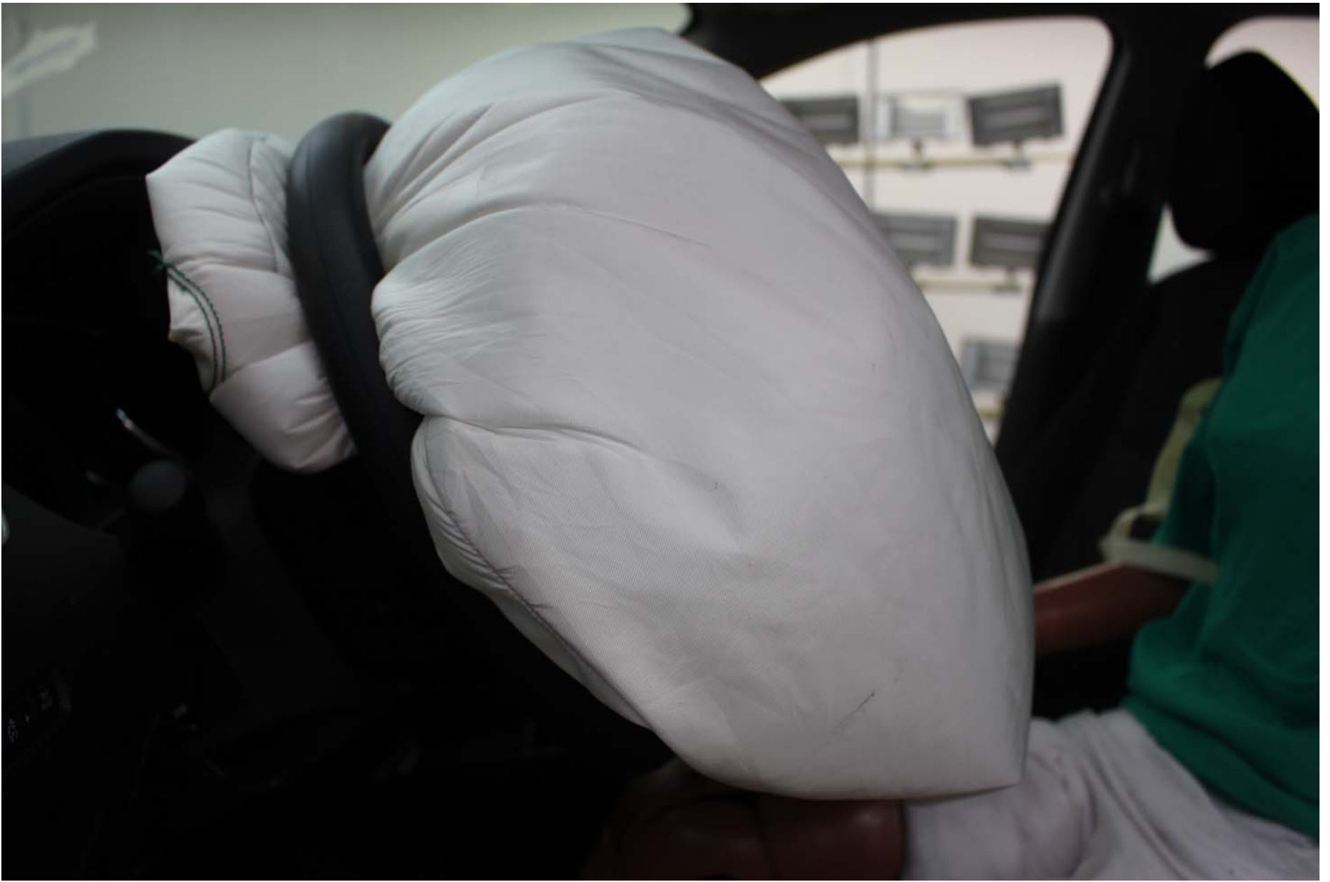
Photo No. 12 - Post-Test 5th Fem. P2 Driver Dummy Airbag Left Side View
