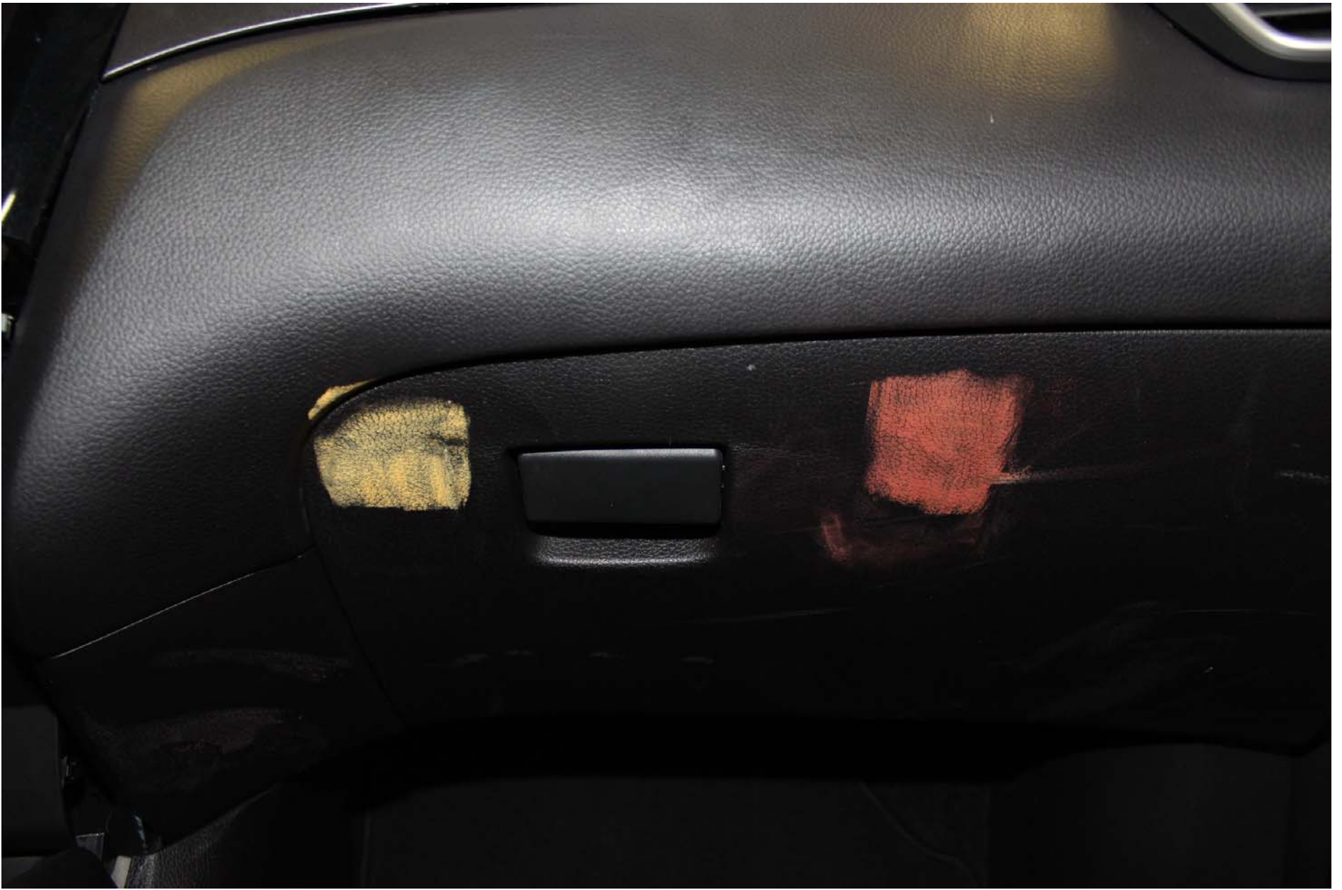
Photo No. 61 - Post-Test Passenger Dummy Knee Contact
