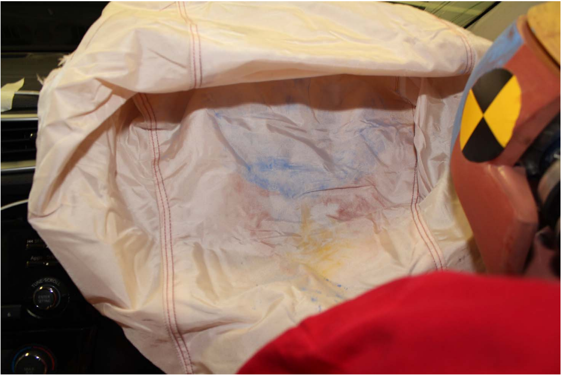
Photo No. 60 - Post-Test Passenger Dummy Airbag Contact
