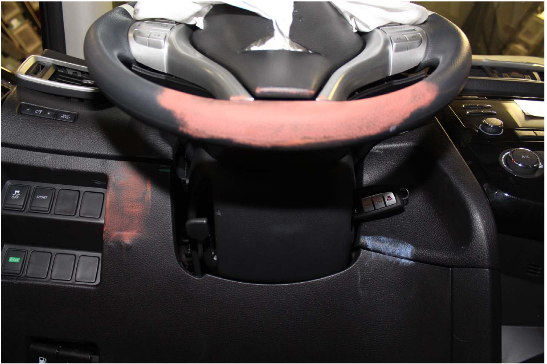
Photo No. 47 - Post-Test Driver Dummy Knee Contact
