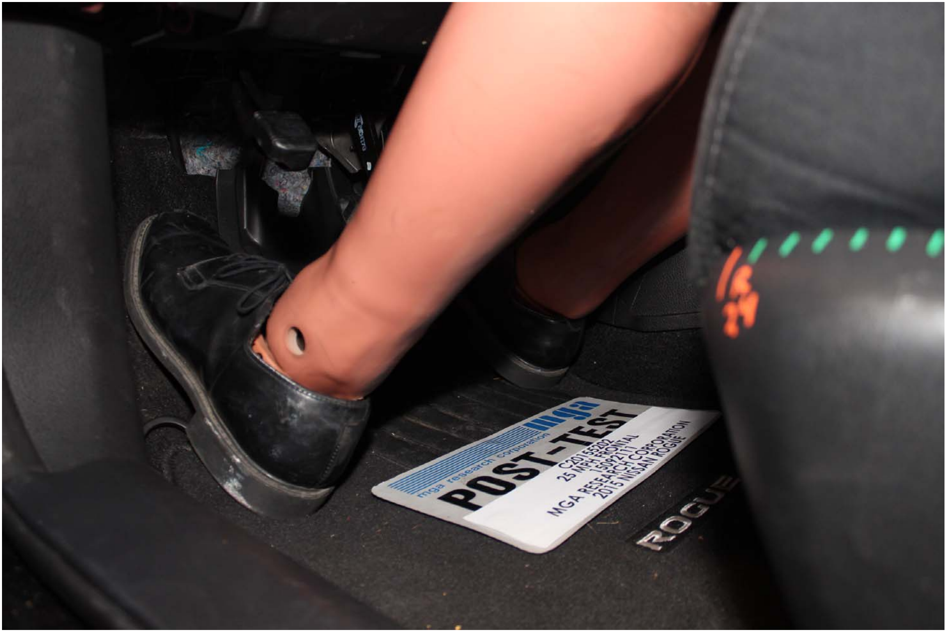
Photo No. 42 - Post-Test Driver Dummy Feet Position
