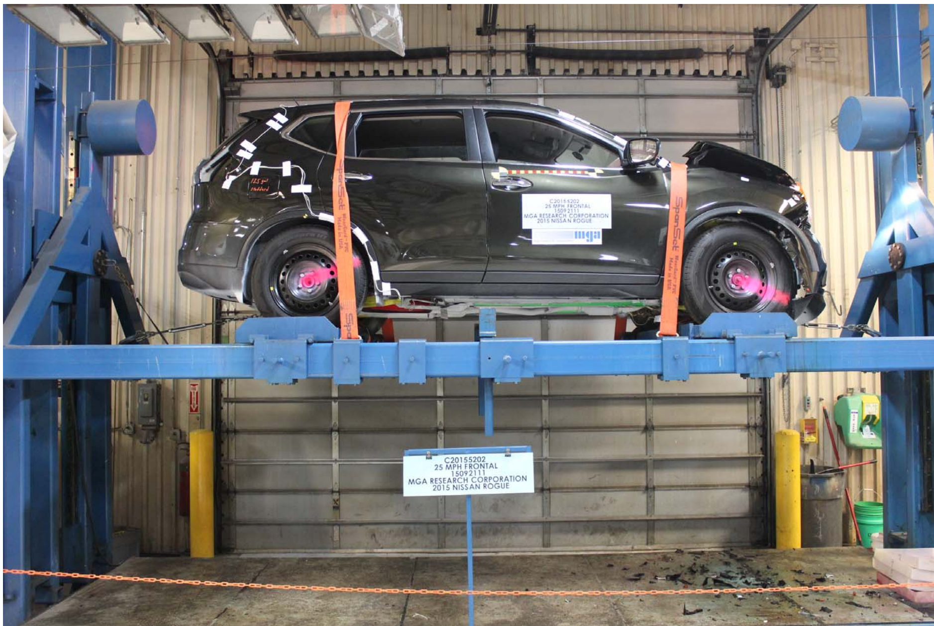
Photo No. 65 - Rollover 360 Degrees
