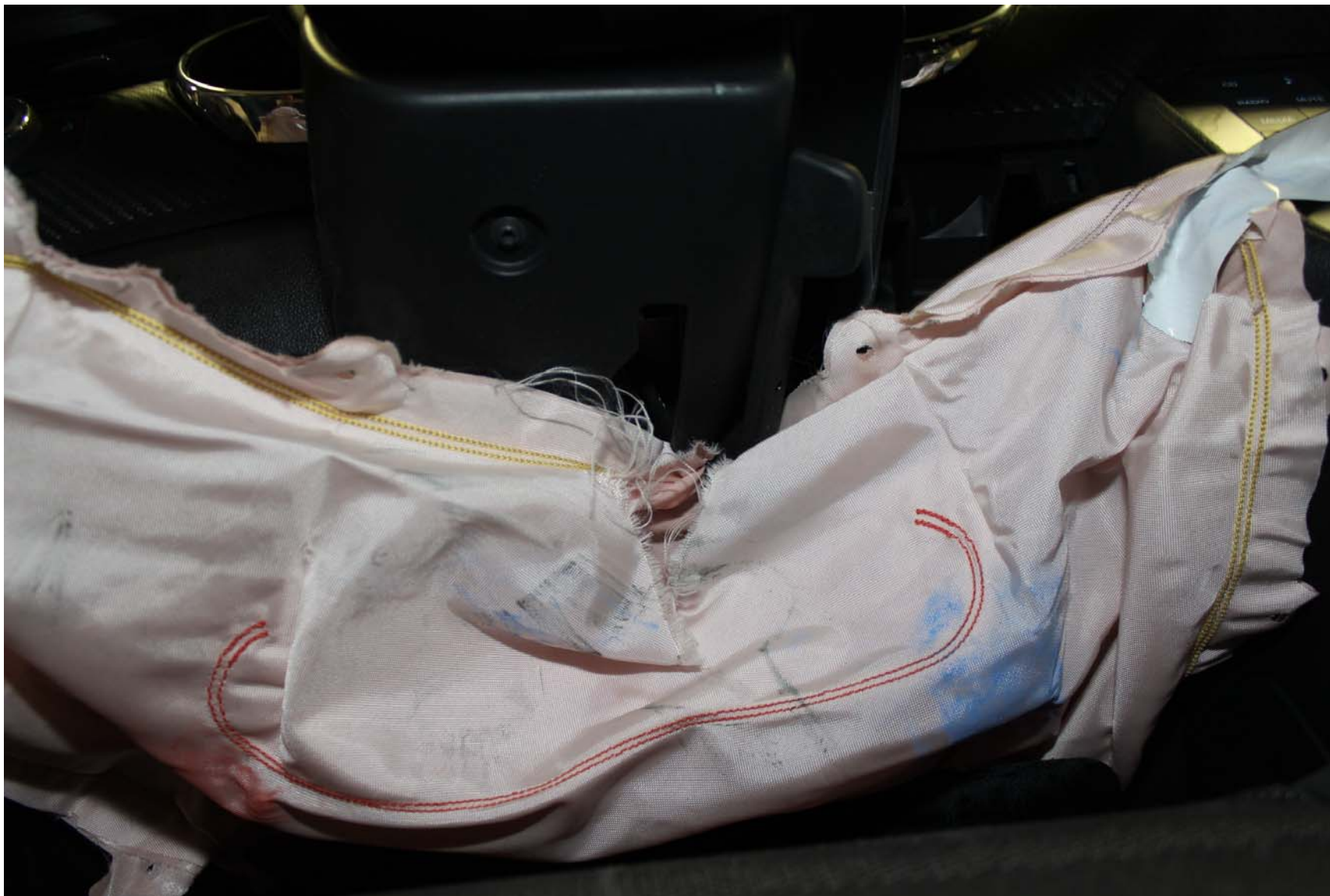
Photo No. 47 - Post-Test Driver Dummy Knee Contact
