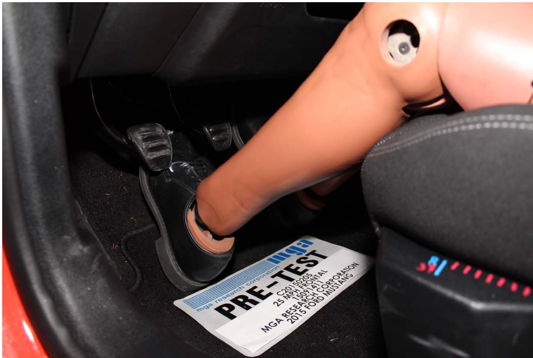
Photo No. 41 - Pre-Test Driver Dummy Feet Position
