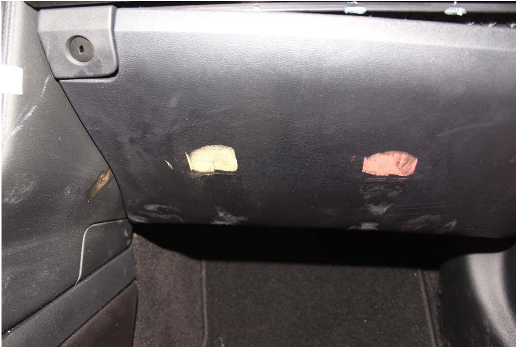
Photo No. 62 - Post-Test Passenger Dummy Knee Contact
