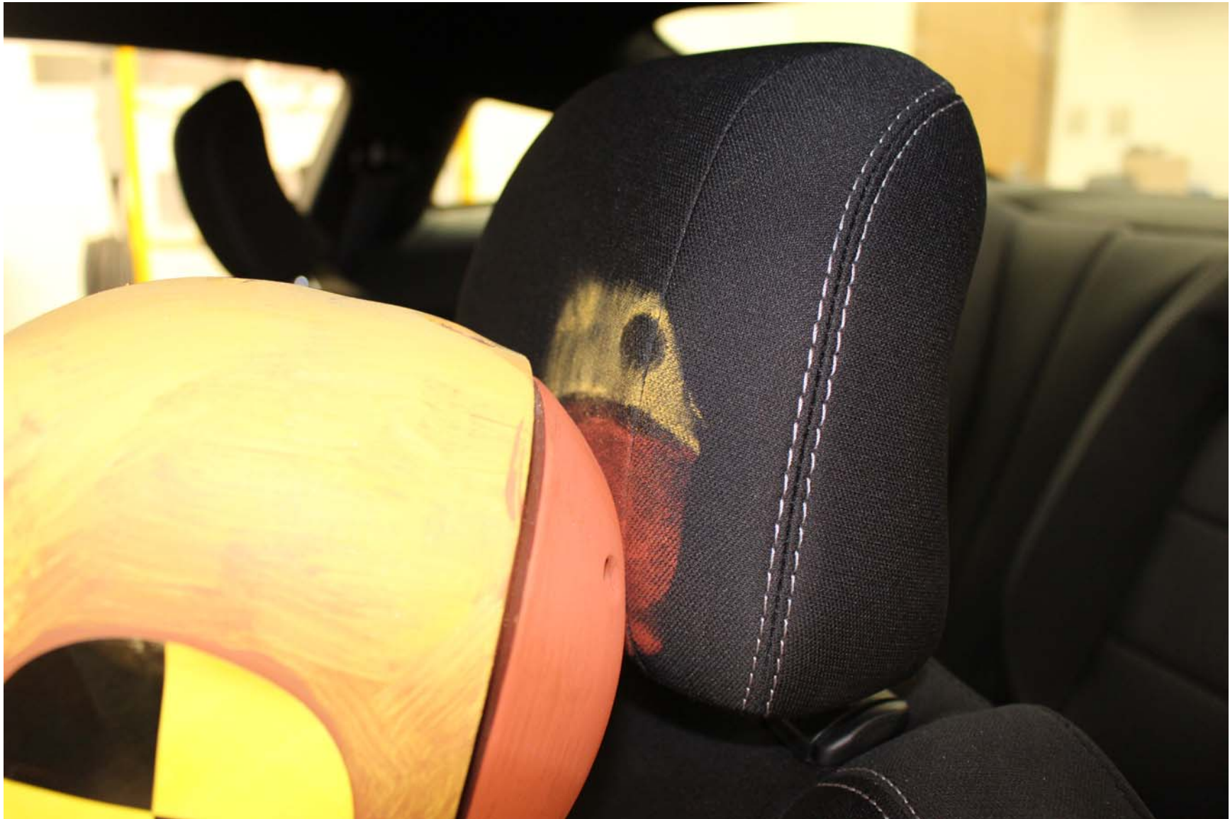
Photo No. 7 - Post-Test 5th Fem. P1 Driver Dummy Head Contact (headrest)
