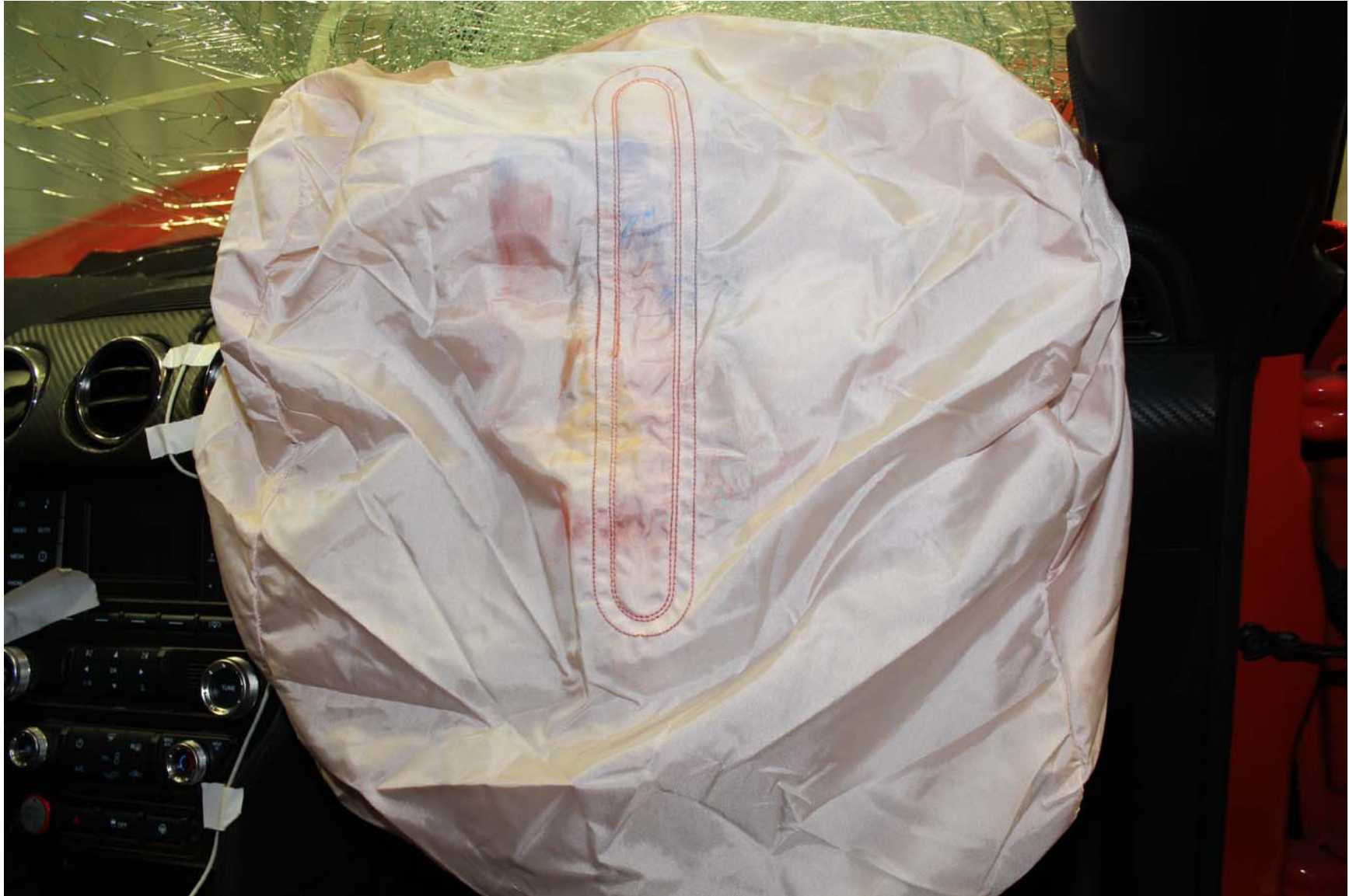
Photo No. 60 - Post-Test Passenger Dummy Airbag Contact
