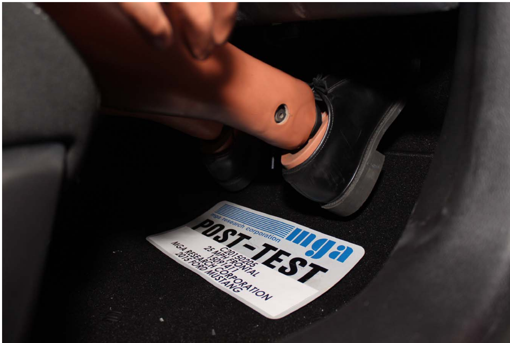
Photo No. 57 - Post-Test Passenger Dummy Feet Position
