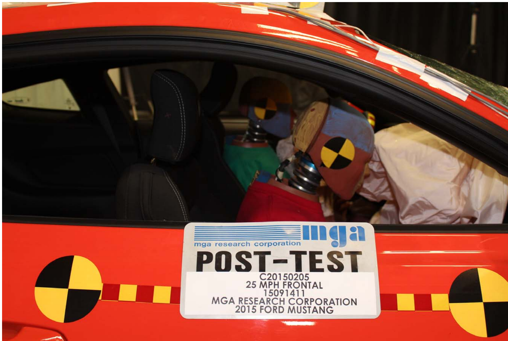
Photo No. 51 - Post-Test Passenger Dummy Position Right Side View
