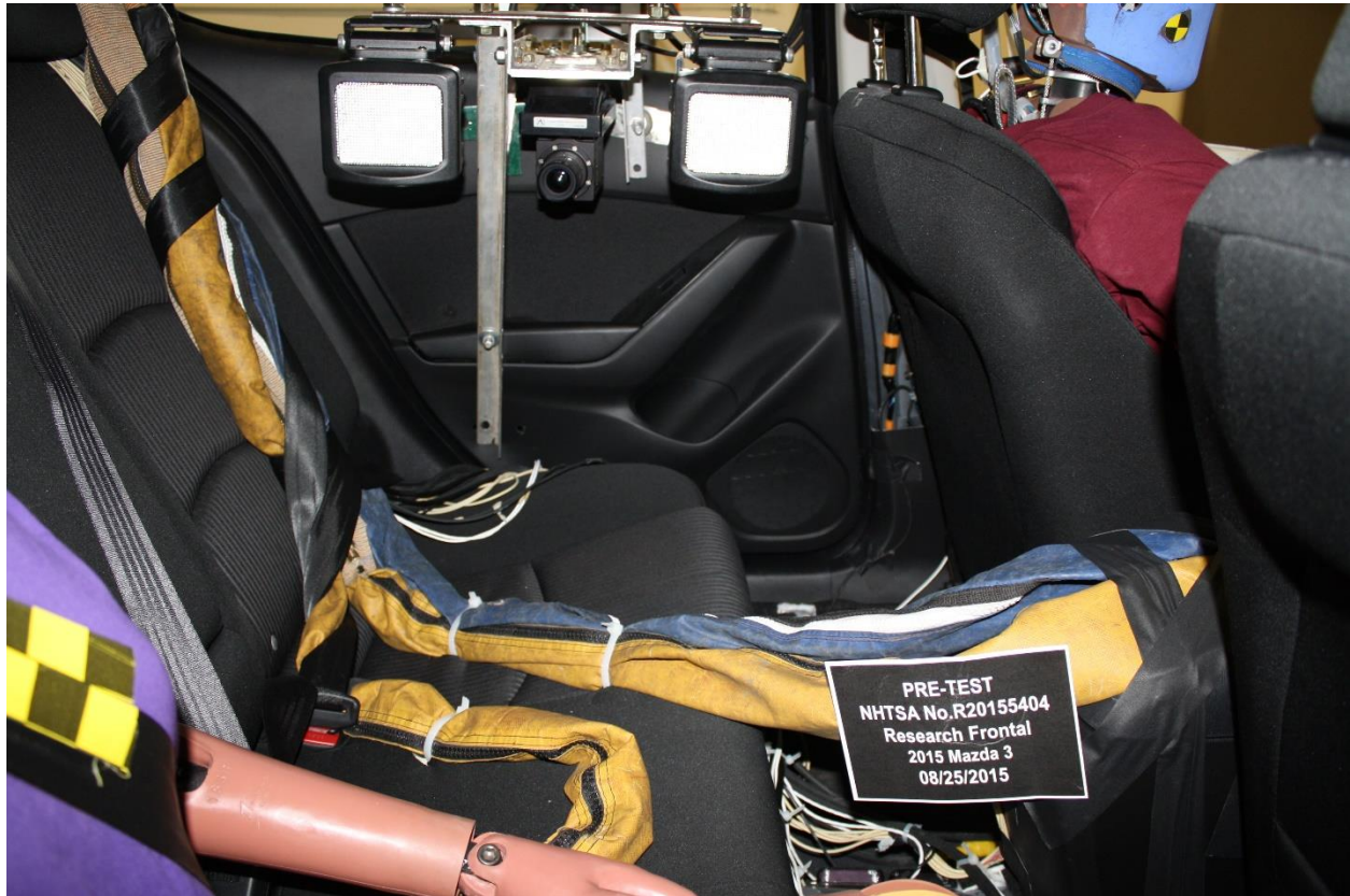
Figure A-27: Pre-Test Dummy Cable Routing
