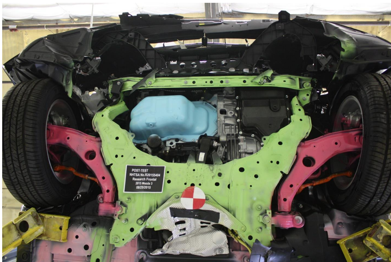
Figure A-24: Post-Test Front Underbody View
