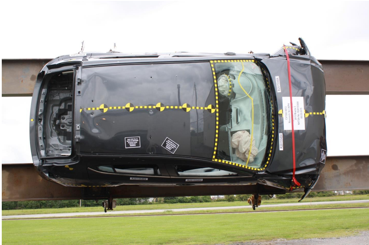
Figure A-75: Vehicle at 270° on Static Rollover Device
