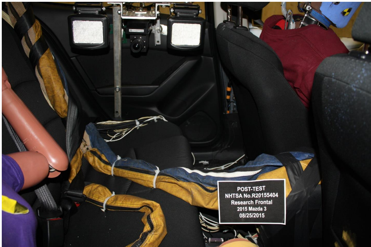
Figure A-28: Post-Test Dummy Cable Routing
