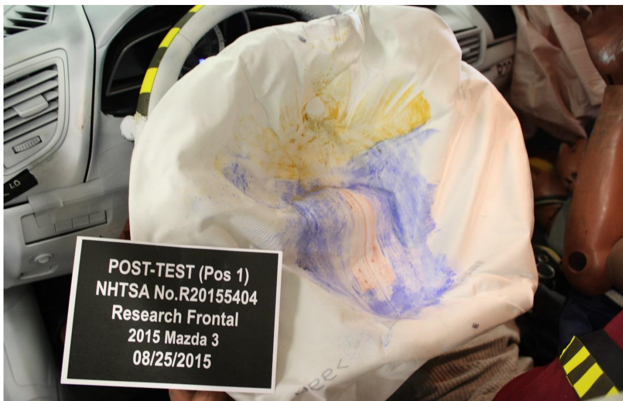
Figure A-46: Post-Test Driver Dummy Contact With Airbag
