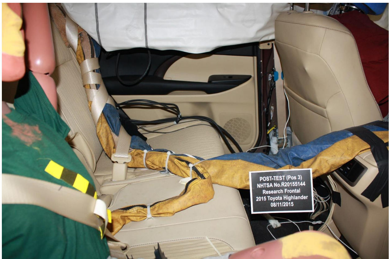
Figure A-28: Post-Test Dummy Cable Routing
