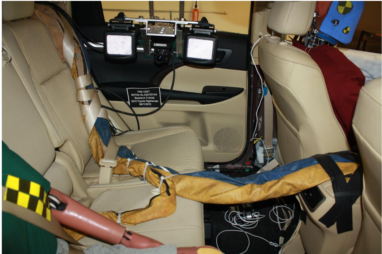
Figure A-27: Pre-Test Dummy Cable Routing
