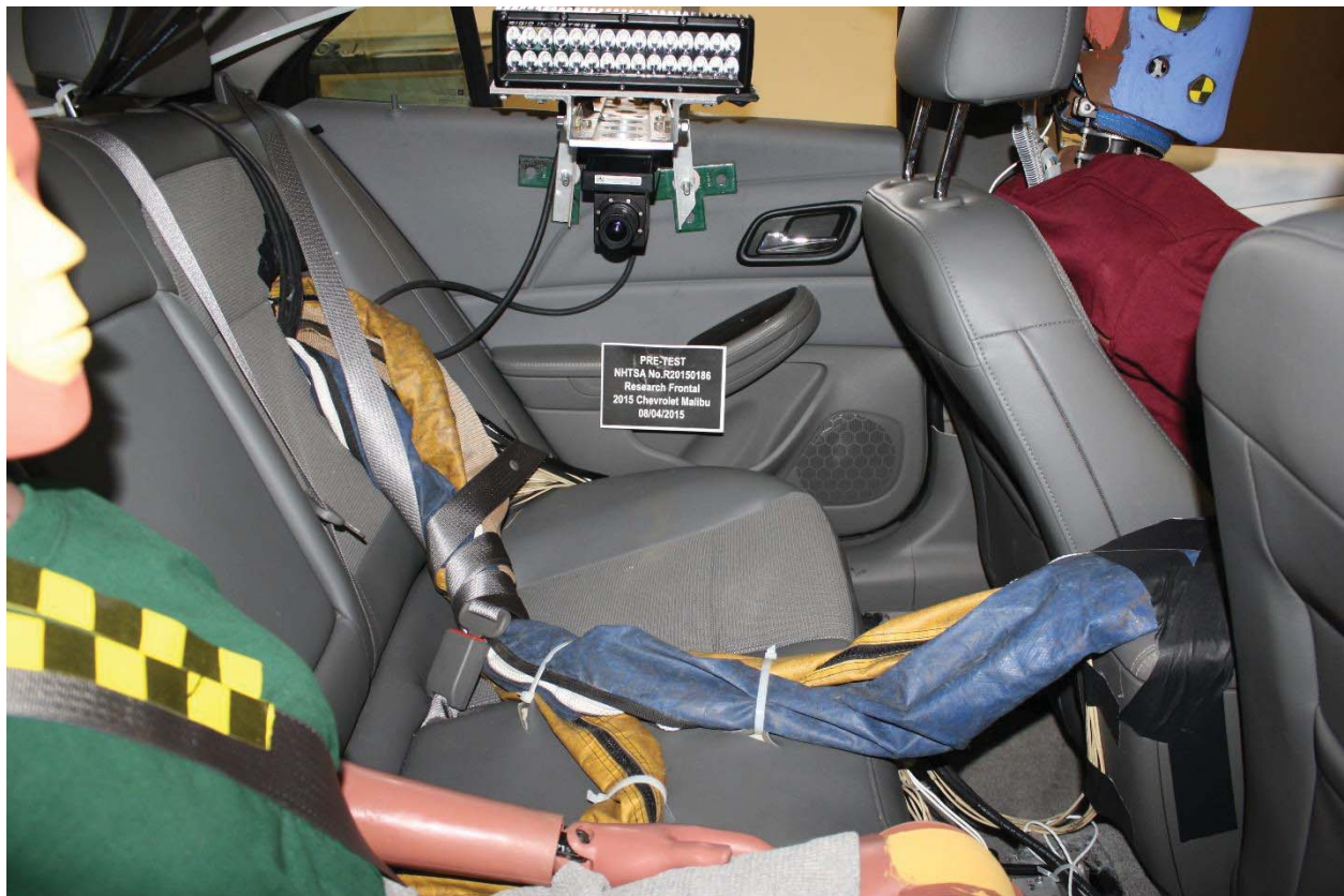
Figure A-27: Pre-Test Dummy Cable Routing
