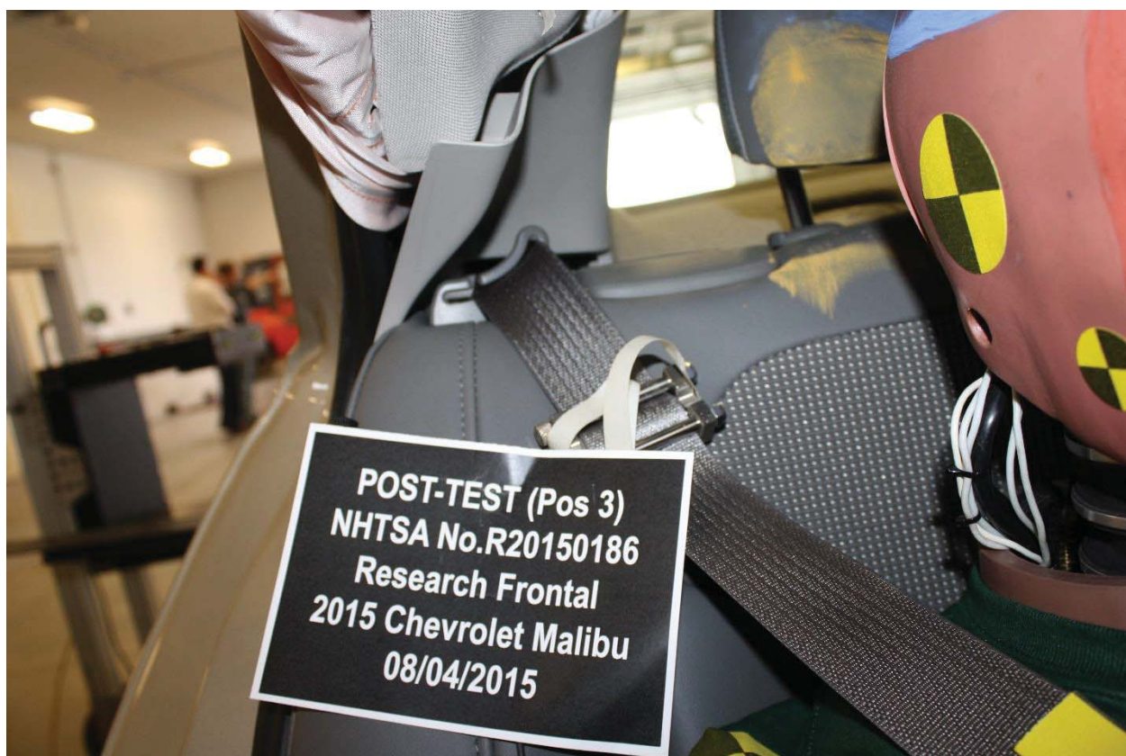
Figure A-88: Post-Test View of Belt Anchorage for Rear Passenger Dummy
