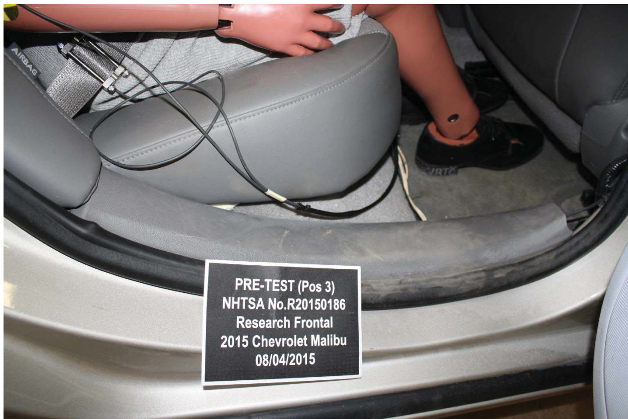
Figure A-85: Pre-Test Rear Passenger Seat Fore-Aft Markings
