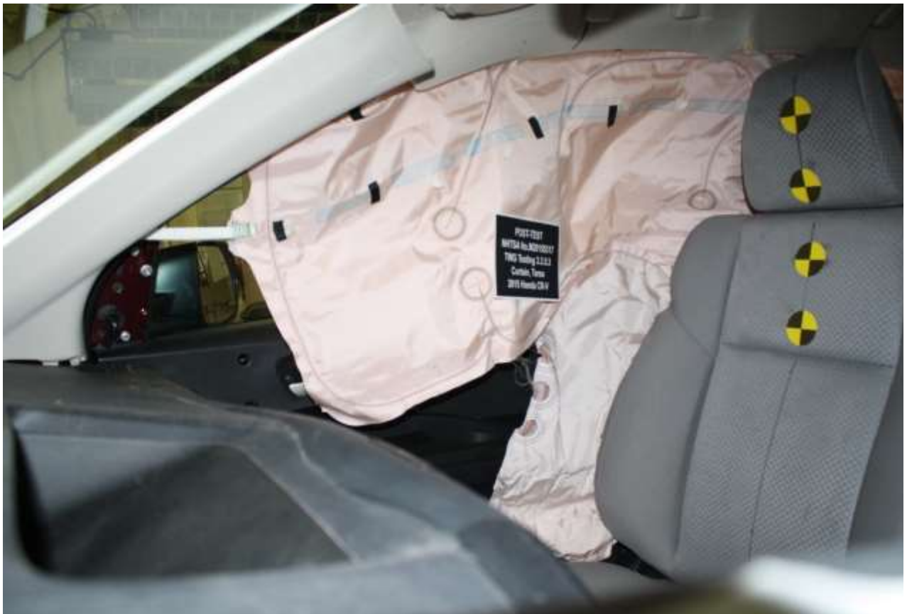
Figure A-20: Post-Test Curtain Airbag Left \frac{3}{4} Front View
