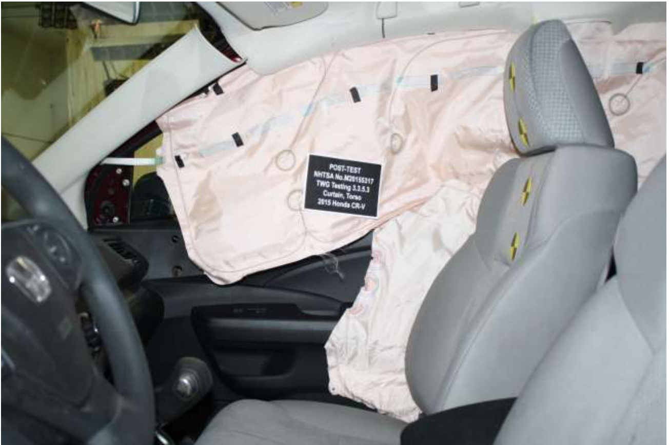
Figure A-19: Post-Test Curtain Airbag Left Side View
