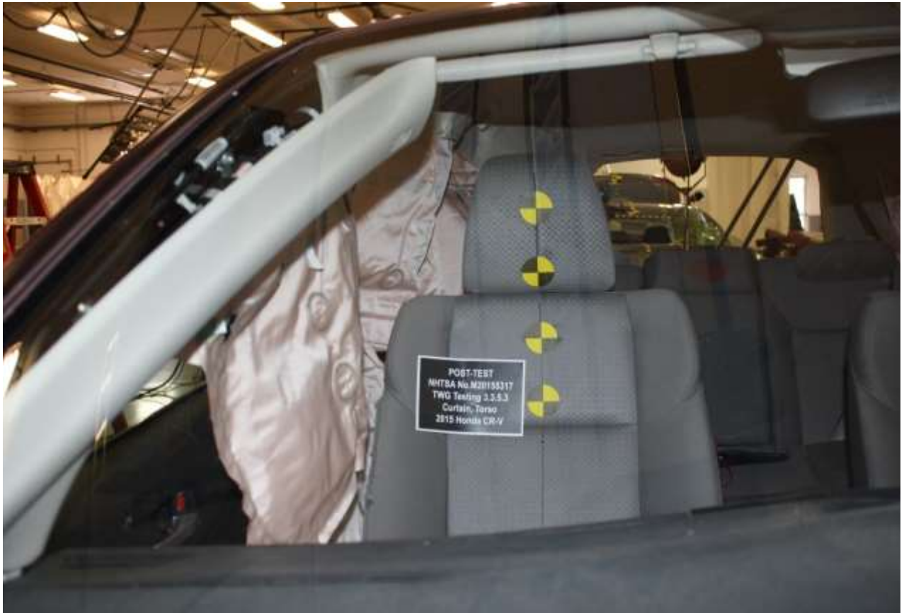
Figure A-21: Post-Test Curtain Airbag Front View
