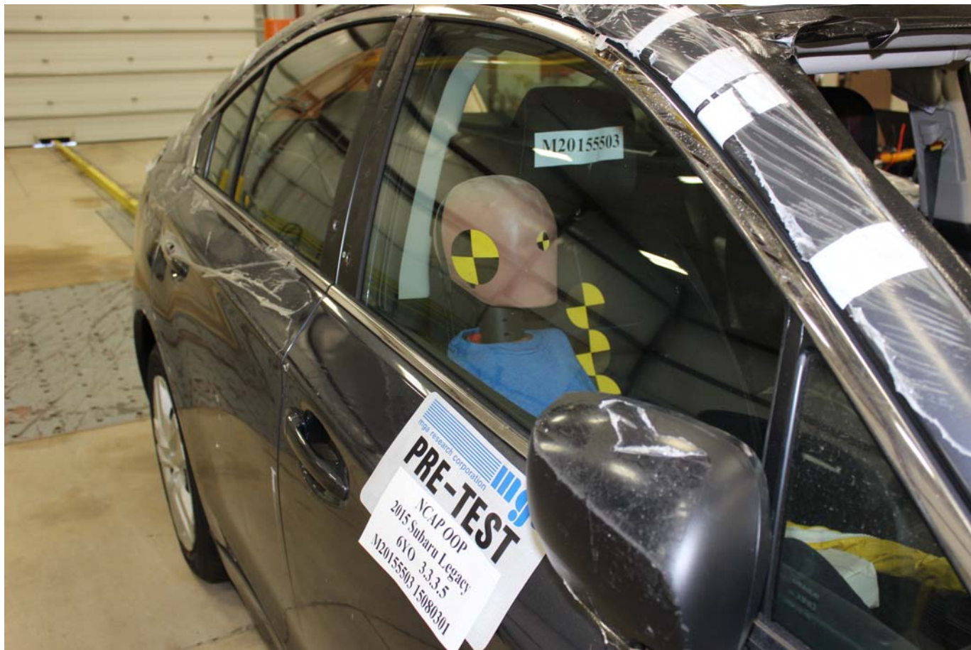
Photo No. 17 - Pre-Test 6-Year-Old Child Dummy Right ¾ Front View
