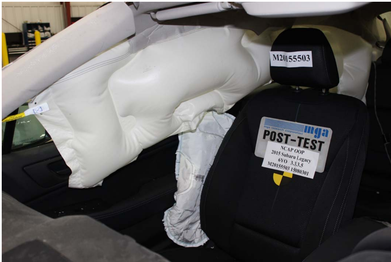
Photo No. 23 - Post-Test Curtain Airbag Left ¾ Front View
