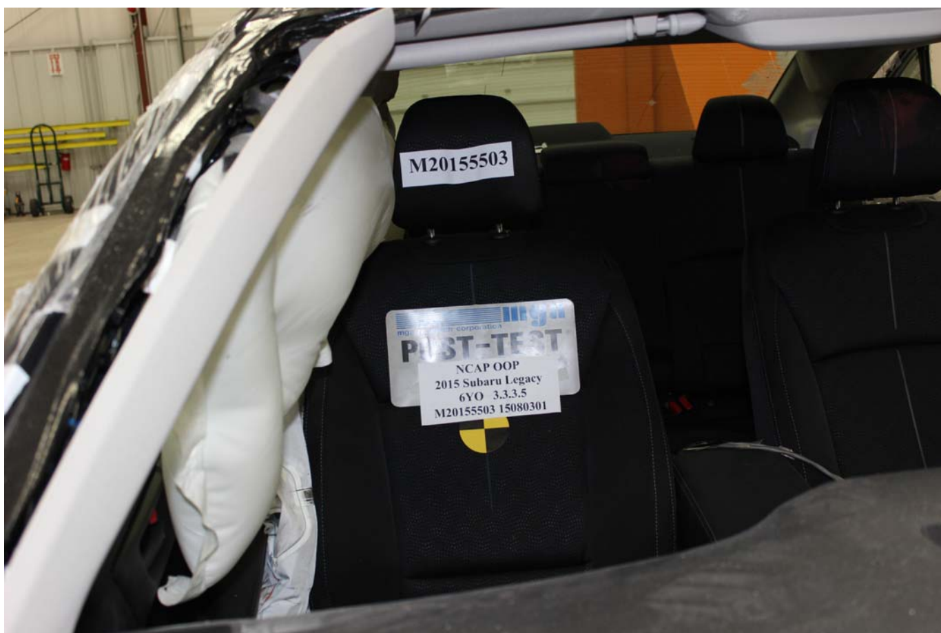
Photo No. 24 - Post-Test Curtain Airbag Front View
