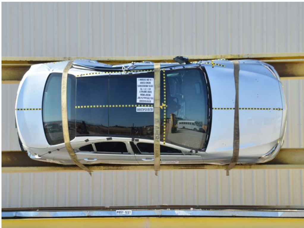
FIGURE 97. FMVSS No. 301 Static Rollover 90 Degrees
