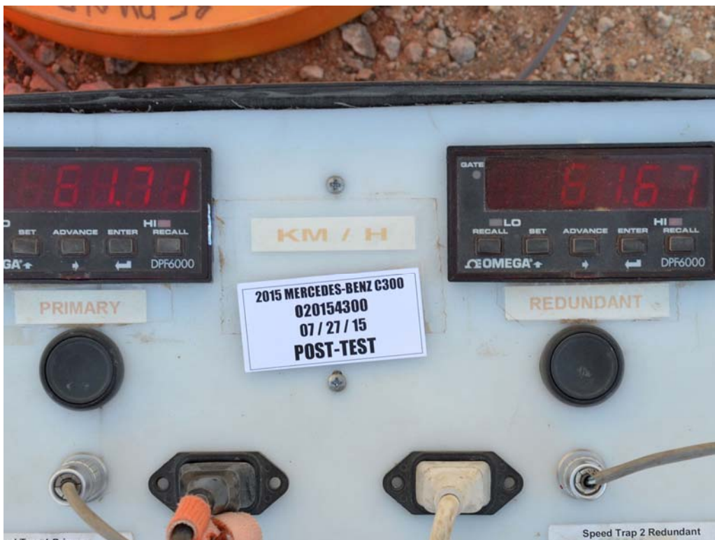
FIGURE 95. Post-Test Primary and Redundant Speed Trap Read-Out
