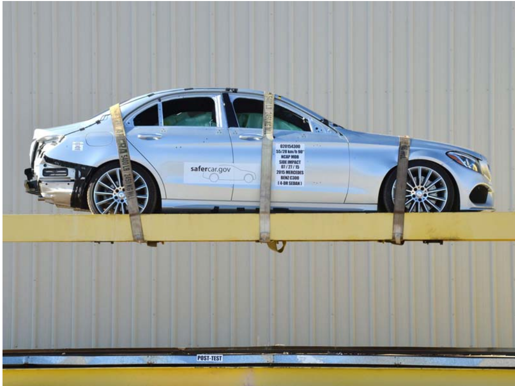
FIGURE 100. FMVSS No. 301 Static Rollover 360 Degrees
