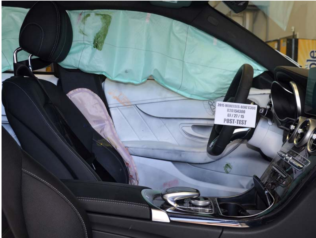
FIGURE 47. Post-Test Driver Inner Door Panel View Showing Driver Dummy Contact Locations
