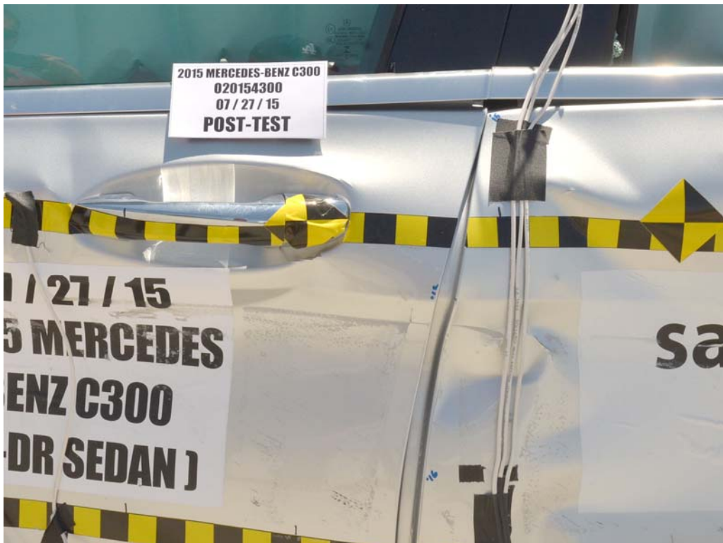
FIGURE 22. Post-Test Left Front Door Latch Close-Up
