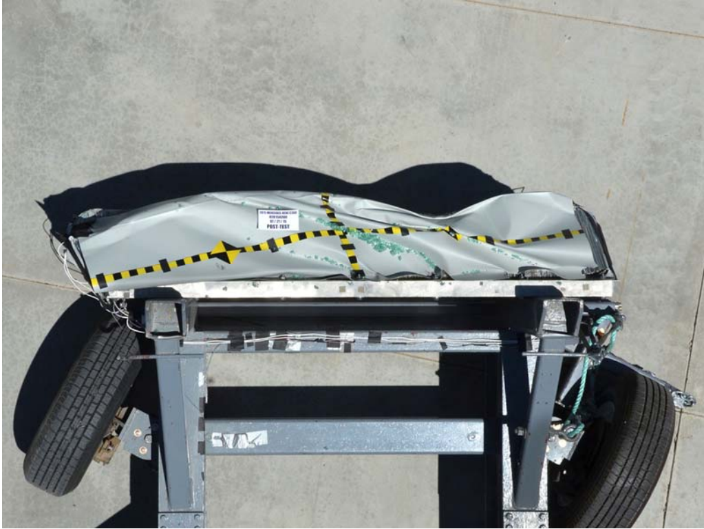
FIGURE 87. Post-Test Top View of MDB Impactor Face
