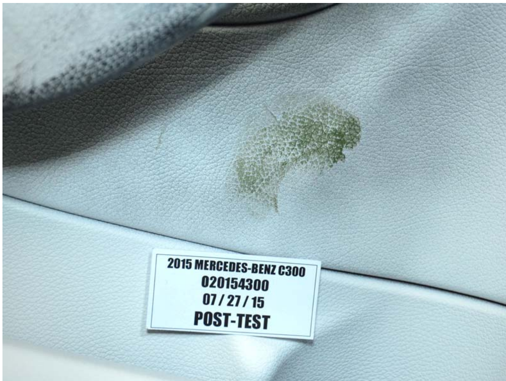
FIGURE 54. Post-Test Driver Dummy Close-Up Knee Contact View
