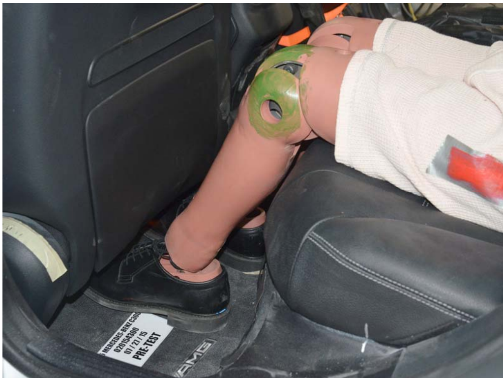
FIGURE 64. Pre-Test Placement of Rear Passenger Dummy's Feet
