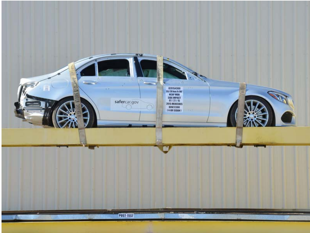
FIGURE 96. FMVSS No. 301 Static Rollover 0 Degrees
