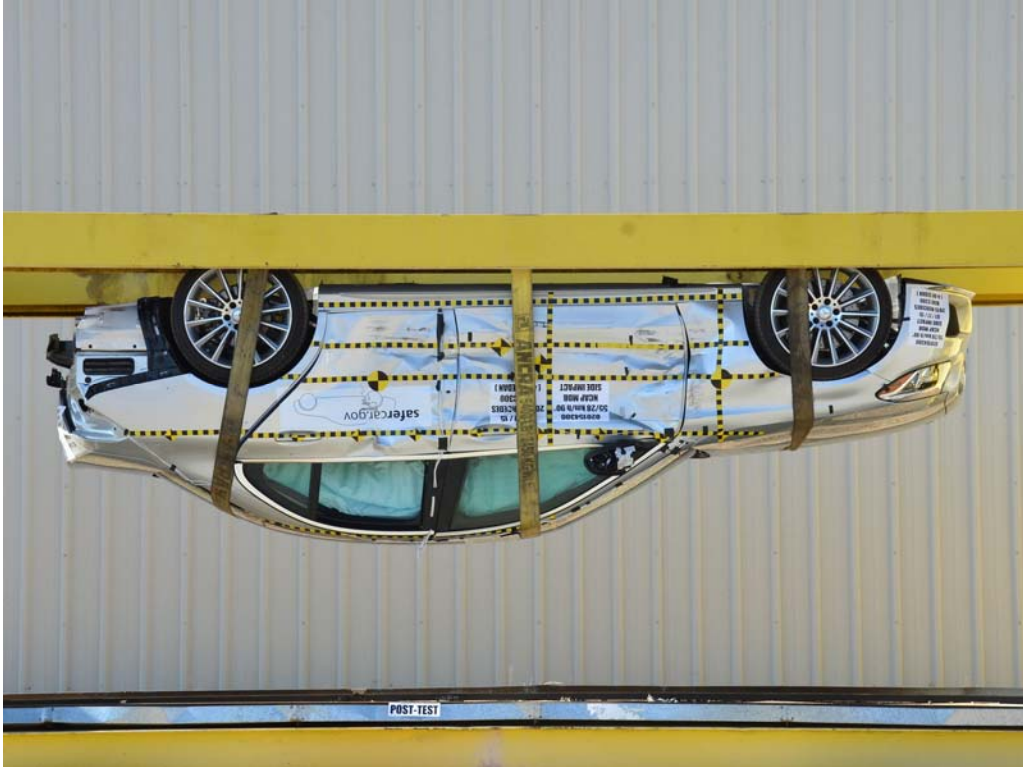
FIGURE 98. FMVSS No. 301 Static Rollover 180 Degrees
