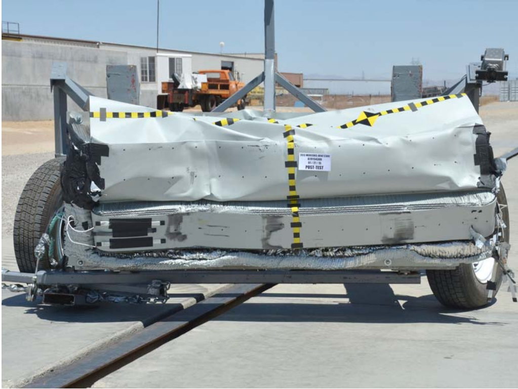
FIGURE 85. Post-Test Front View of MDB Impactor Face
