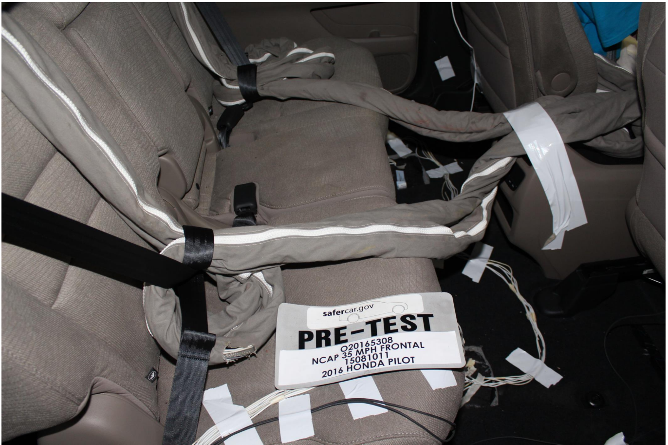
Photo No. 027 - Pre-Test Dummy Cable Routing
