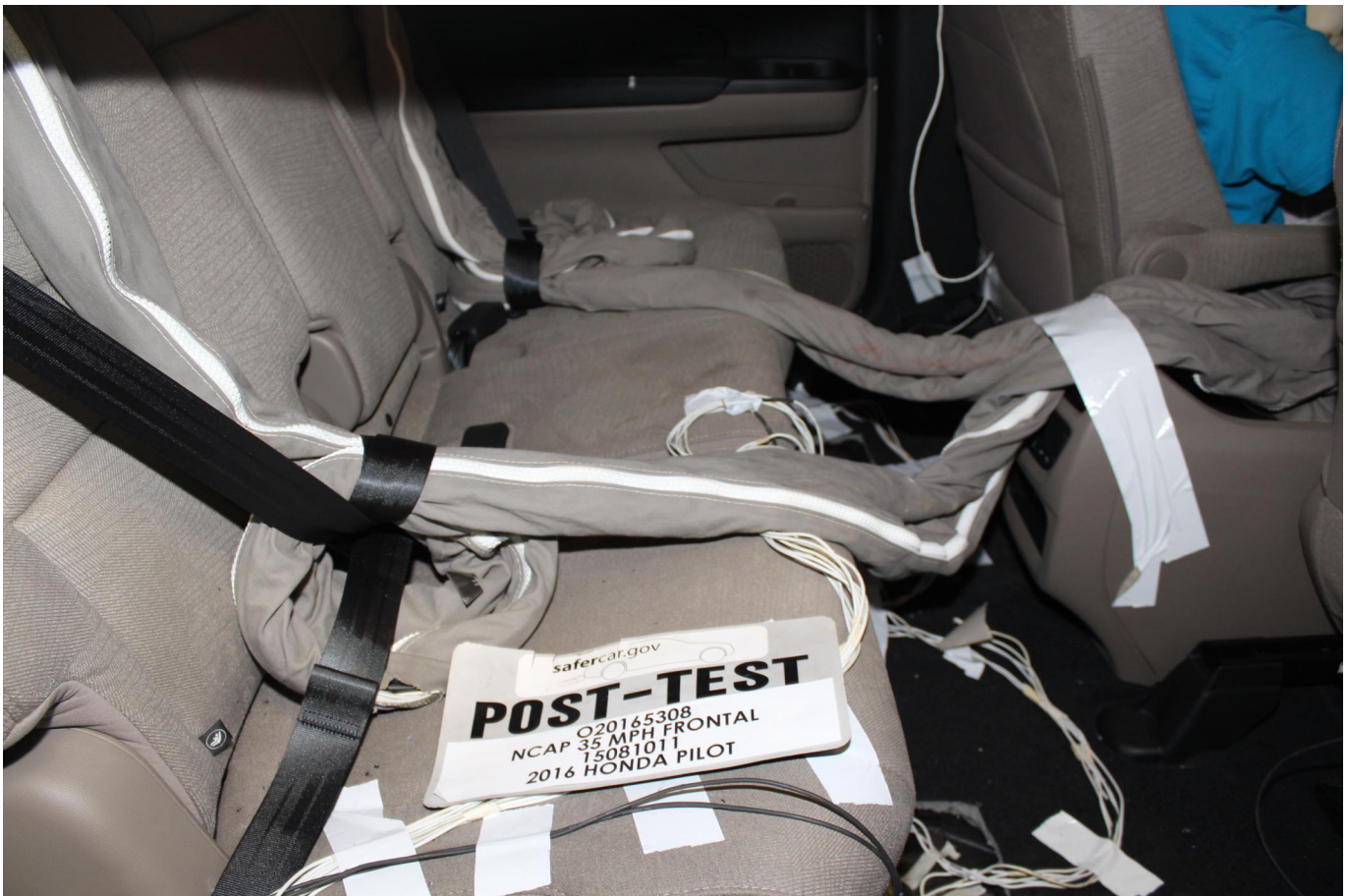
Photo No. 028 - Post-Test Dummy Cable Routing
