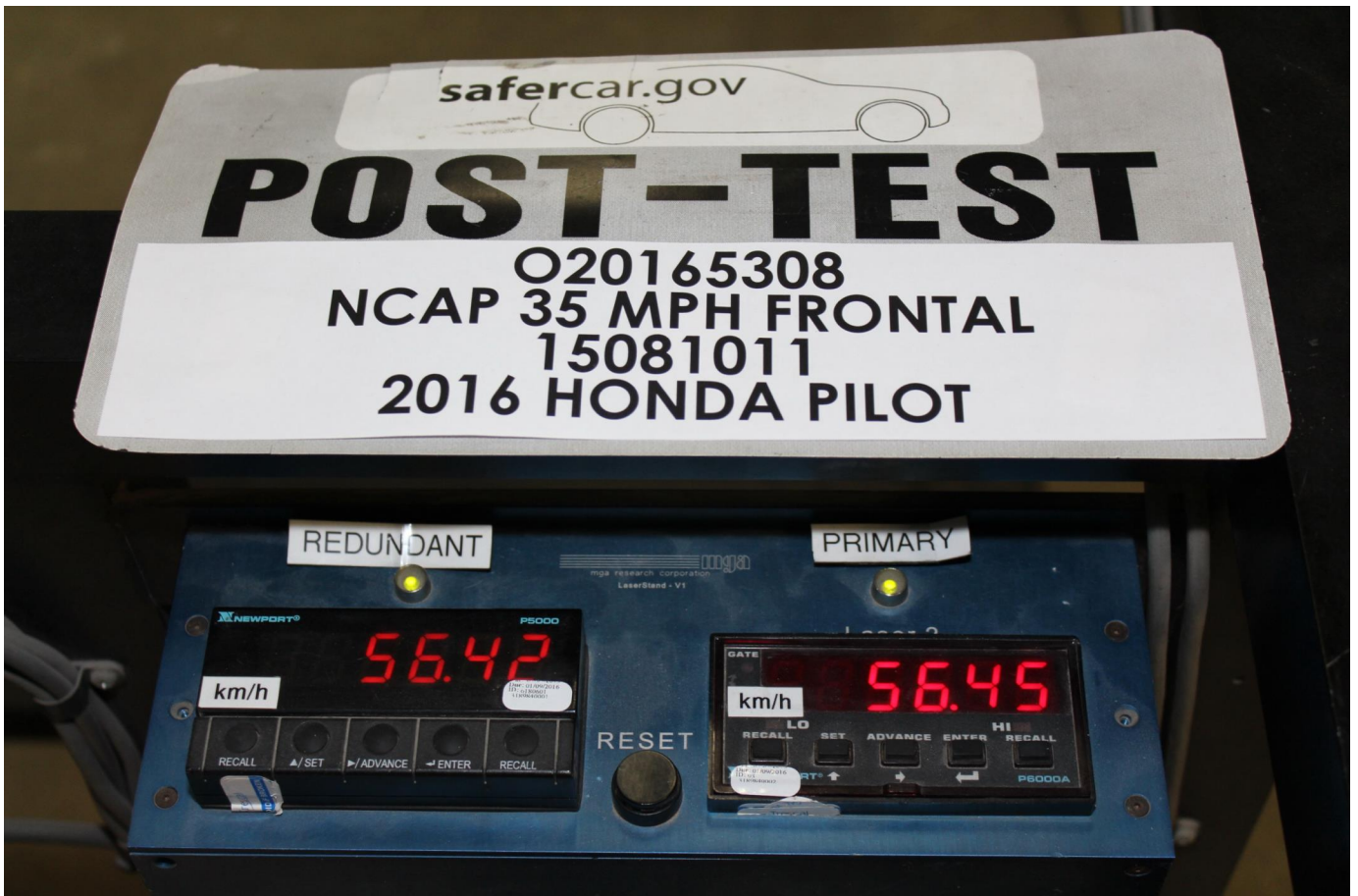
Photo No. 071 - Post-Test Speed Trap Read-Out
