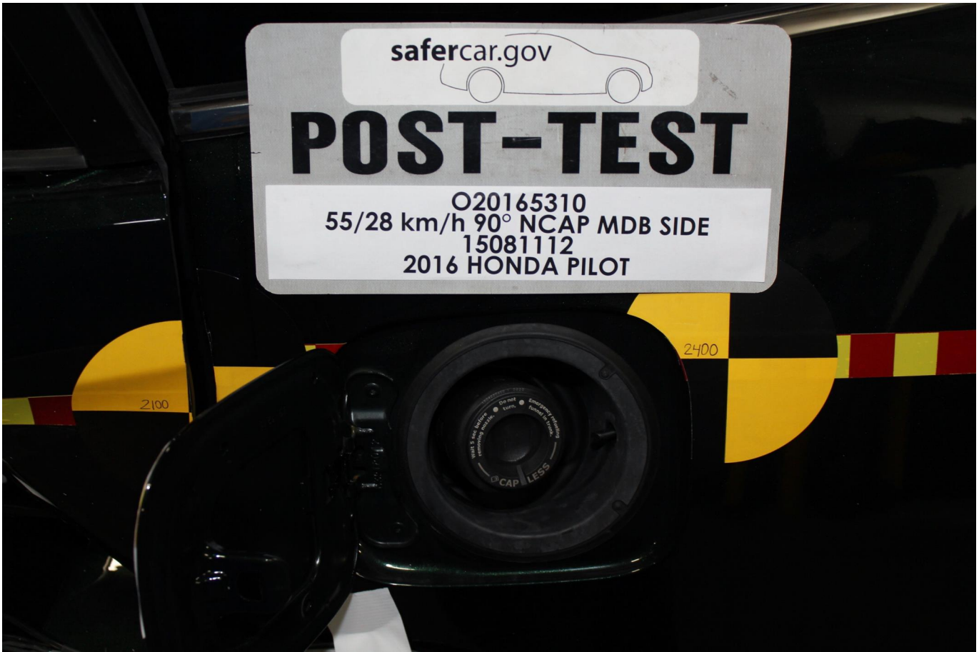
Photo No. 083 - Post-Test View of Fuel Filler Cap or Fuel Filler Neck
