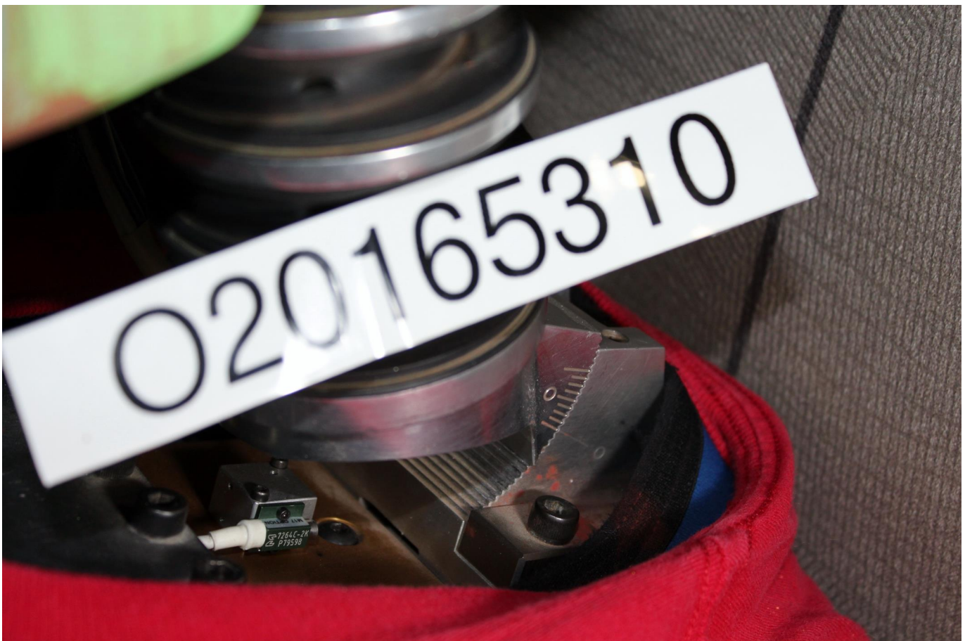
Photo No. 062 - Pre-Test View of Rear Passenger Dummy's Neck Showing Position of Adjustable Neck
