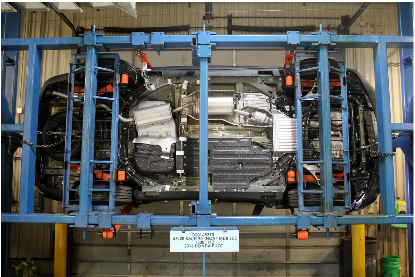
Photo No. 097 - FMVSS No. 301 Static Rollover 90 Degrees
