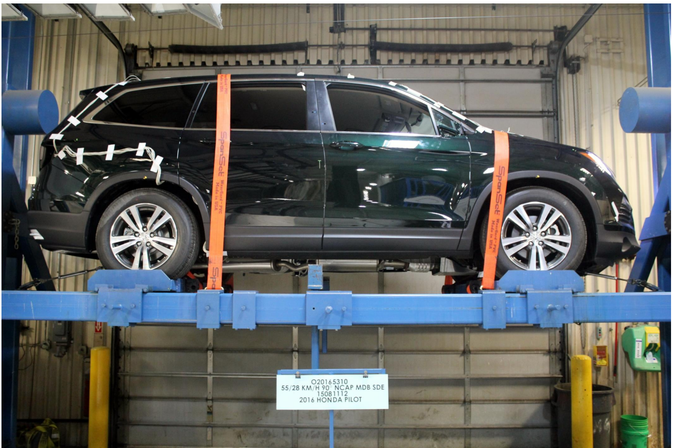
Photo No. 096 - FMVSS No. 301 Static Rollover 0 Degrees
