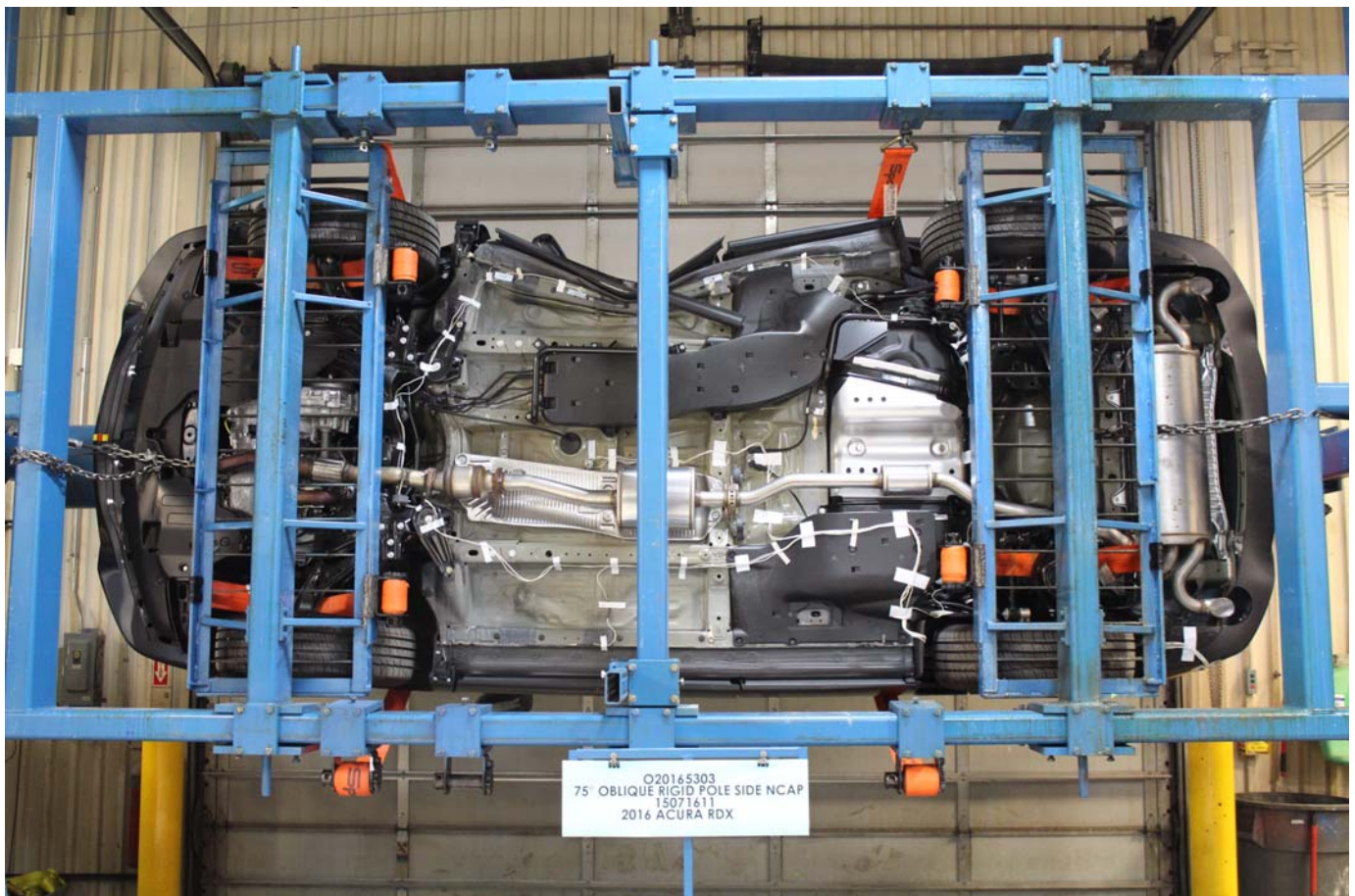
Photo No. 066 - FMVSS No. 301 Static Rollover 270 Degrees
