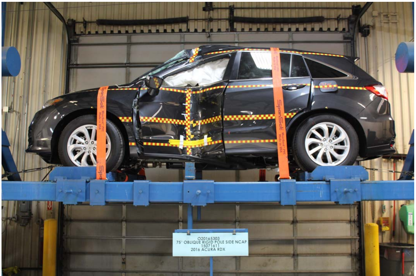
Photo No. 063 - FMVSS No. 301 Static Rollover 0 Degrees
