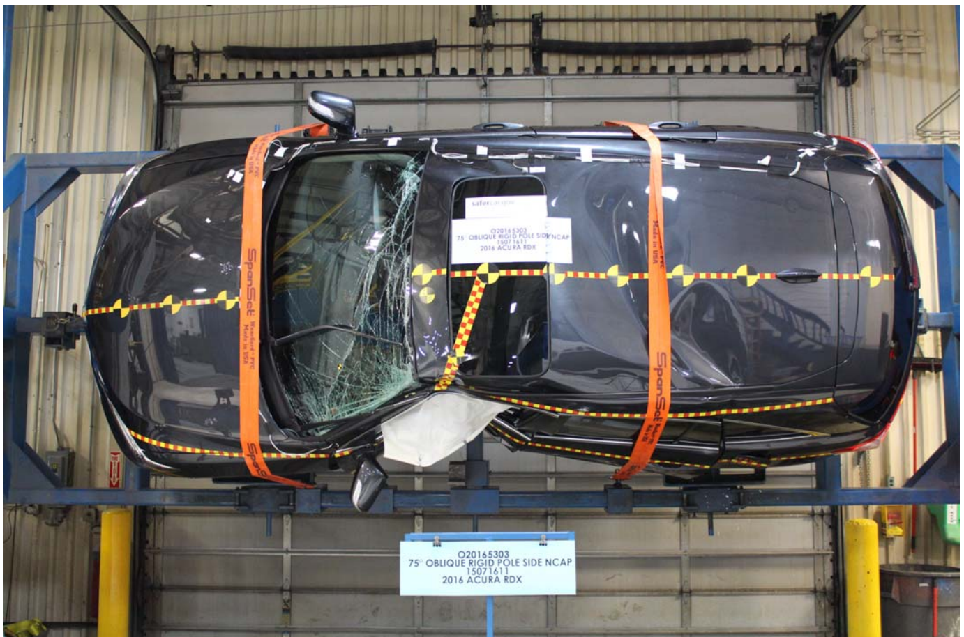
Photo No. 064 - FMVSS No. 301 Static Rollover 90 Degrees
