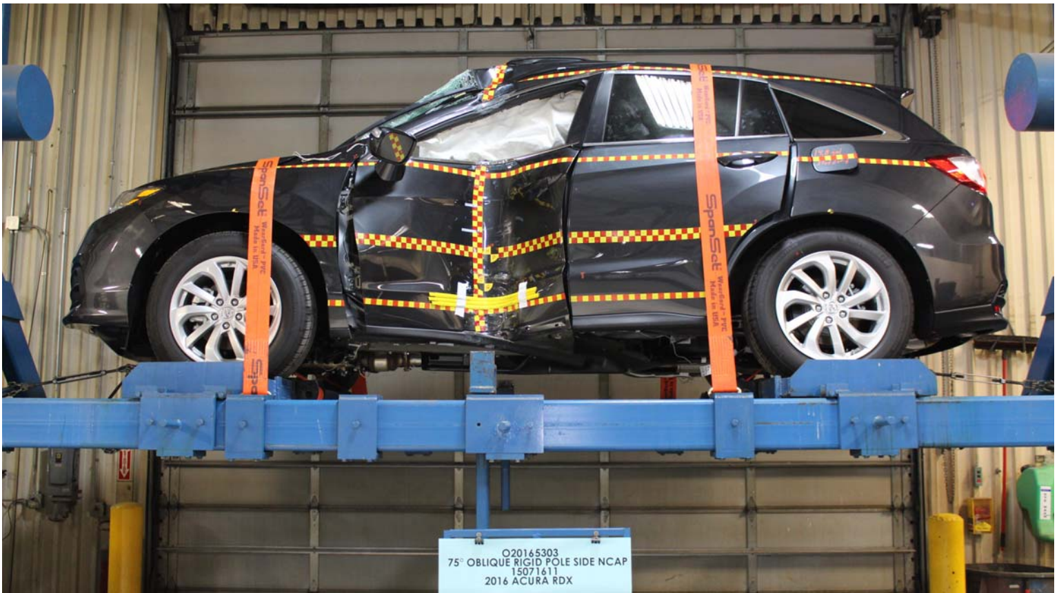
Photo No. 067 - FMVSS No. 301 Static Rollover 360 Degrees
