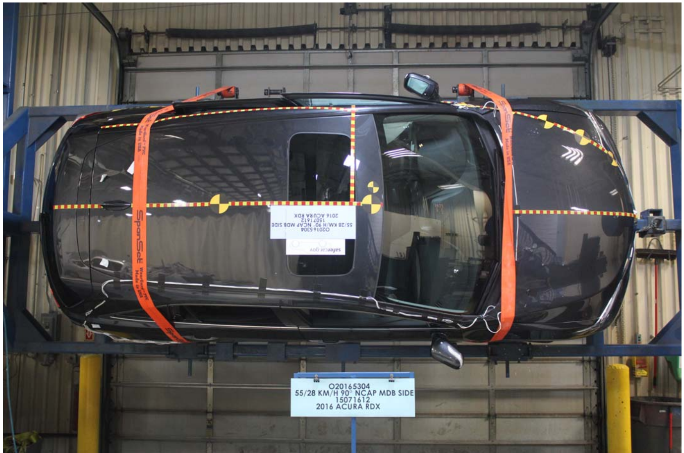
Photo No. 099 - FMVSS No. 301 Static Rollover 270 Degrees
