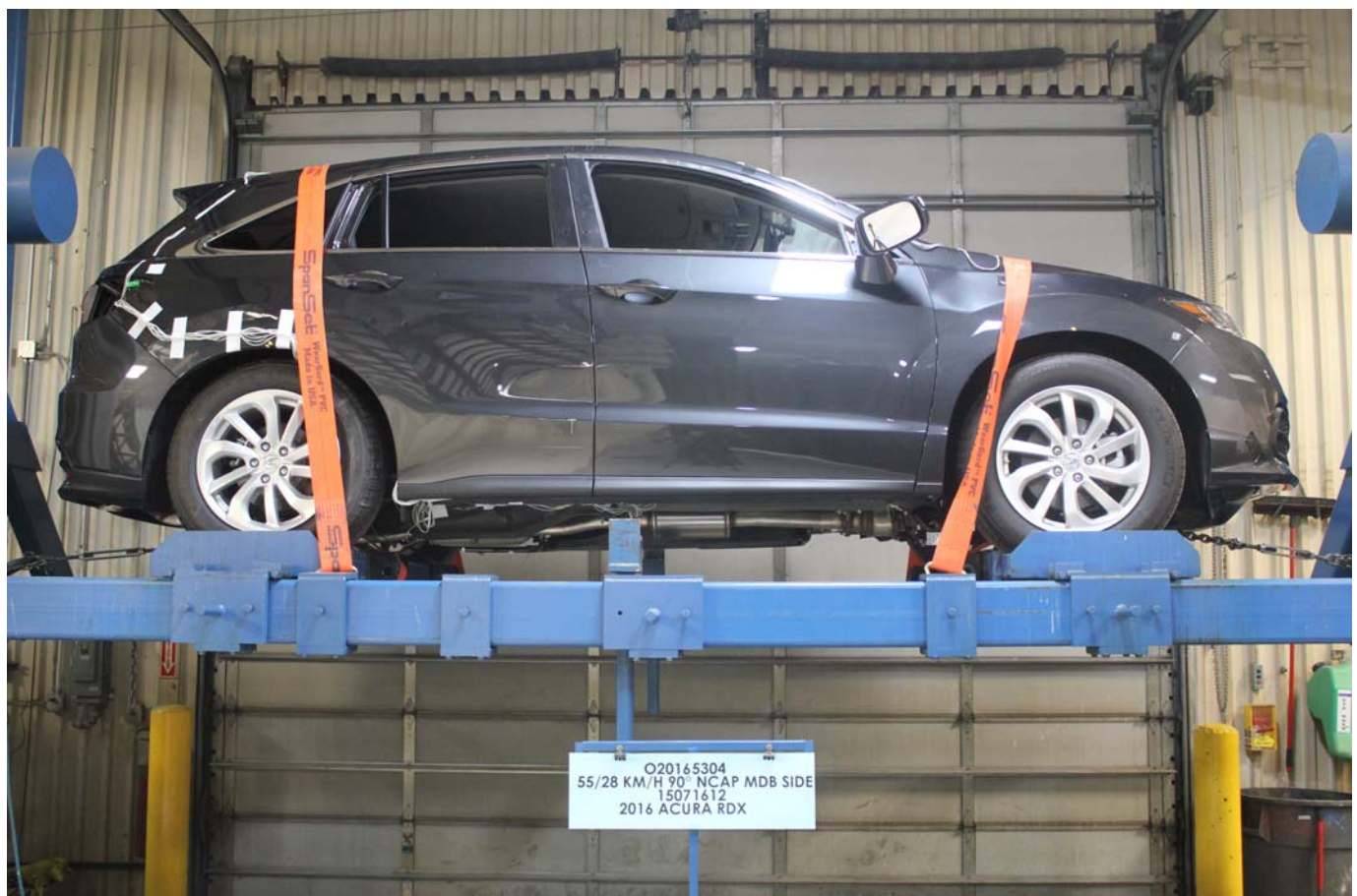
Photo No. 096 - FMVSS No. 301 Static Rollover 0 Degrees
