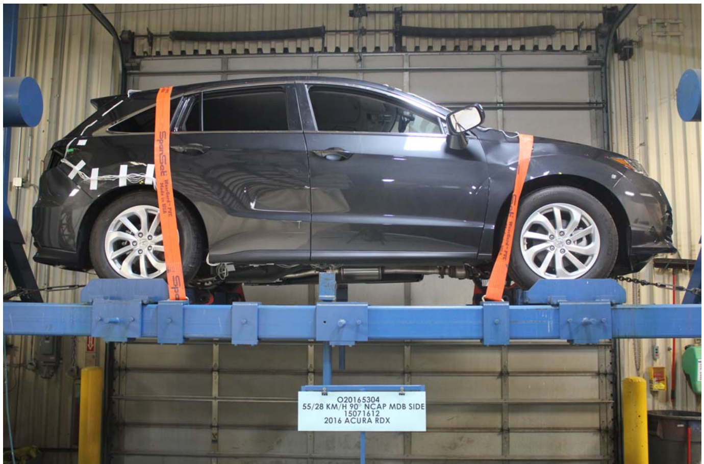
Photo No. 100 - FMVSS No. 301 Static Rollover 360 Degrees
