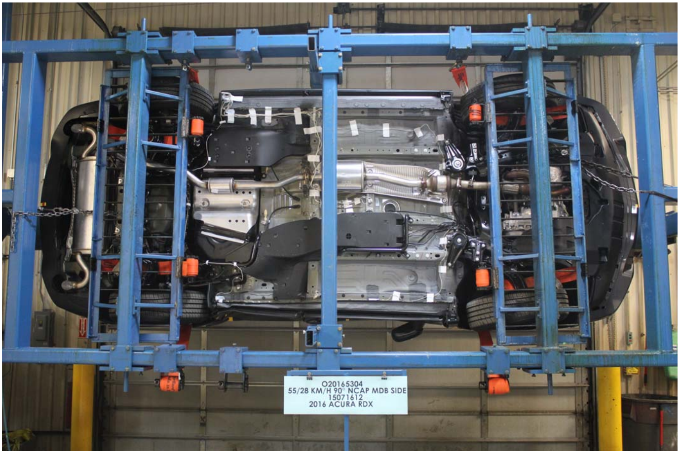
Photo No. 097 - FMVSS No. 301 Static Rollover 90 Degrees
