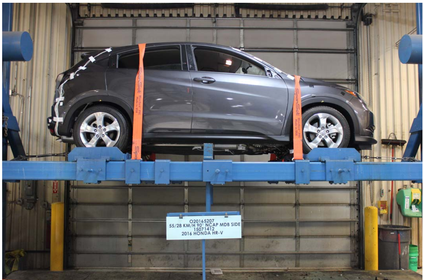
Photo No. 096 - FMVSS No. 301 Static Rollover 0 Degrees
