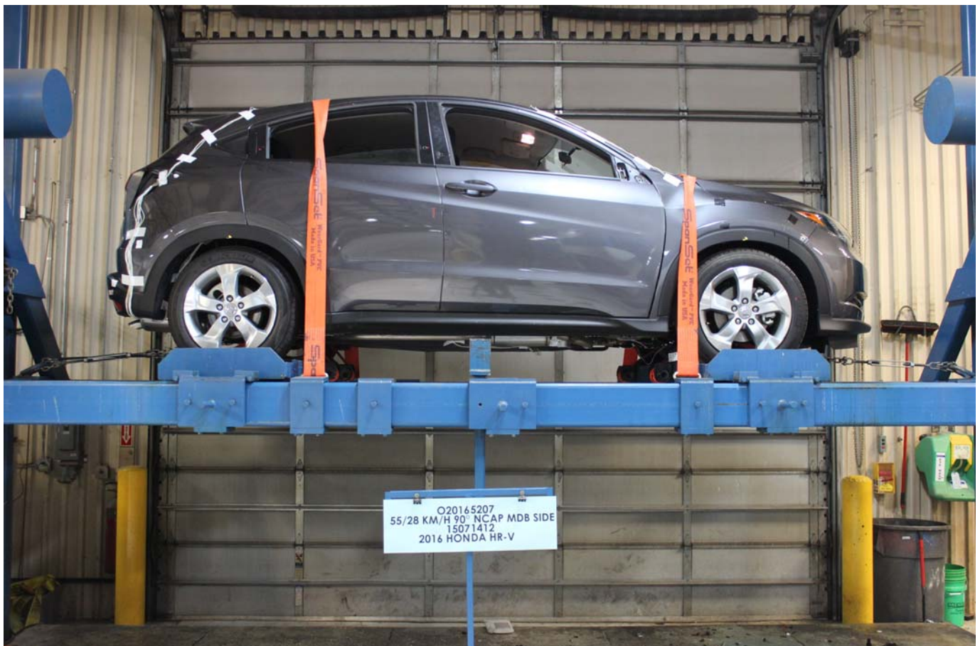
Photo No. 100 - FMVSS No. 301 Static Rollover 360 Degrees
