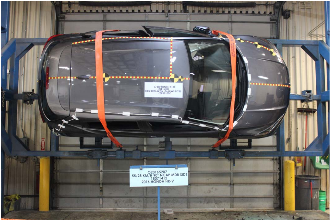
Photo No. 099 - FMVSS No. 301 Static Rollover 270 Degrees
