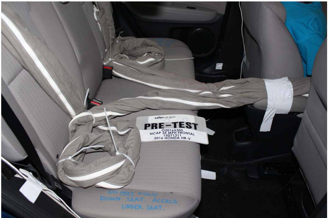
Photo No. 027 - Pre-Test Dummy Cable Routing
