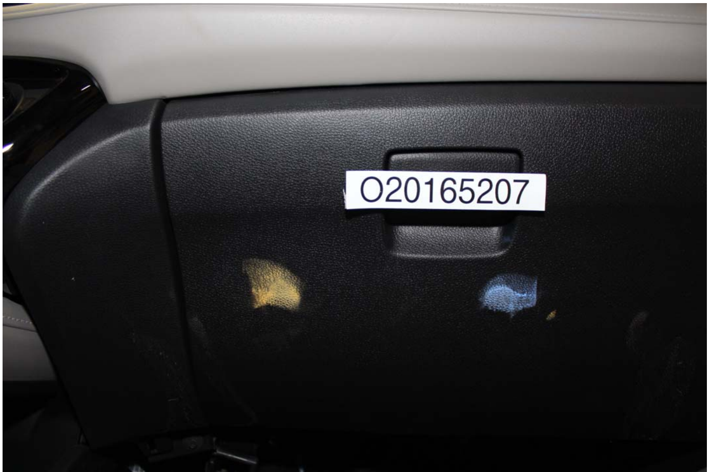
Photo No. 068a - Post-Test Passenger Dummy Contact with Glovebox
