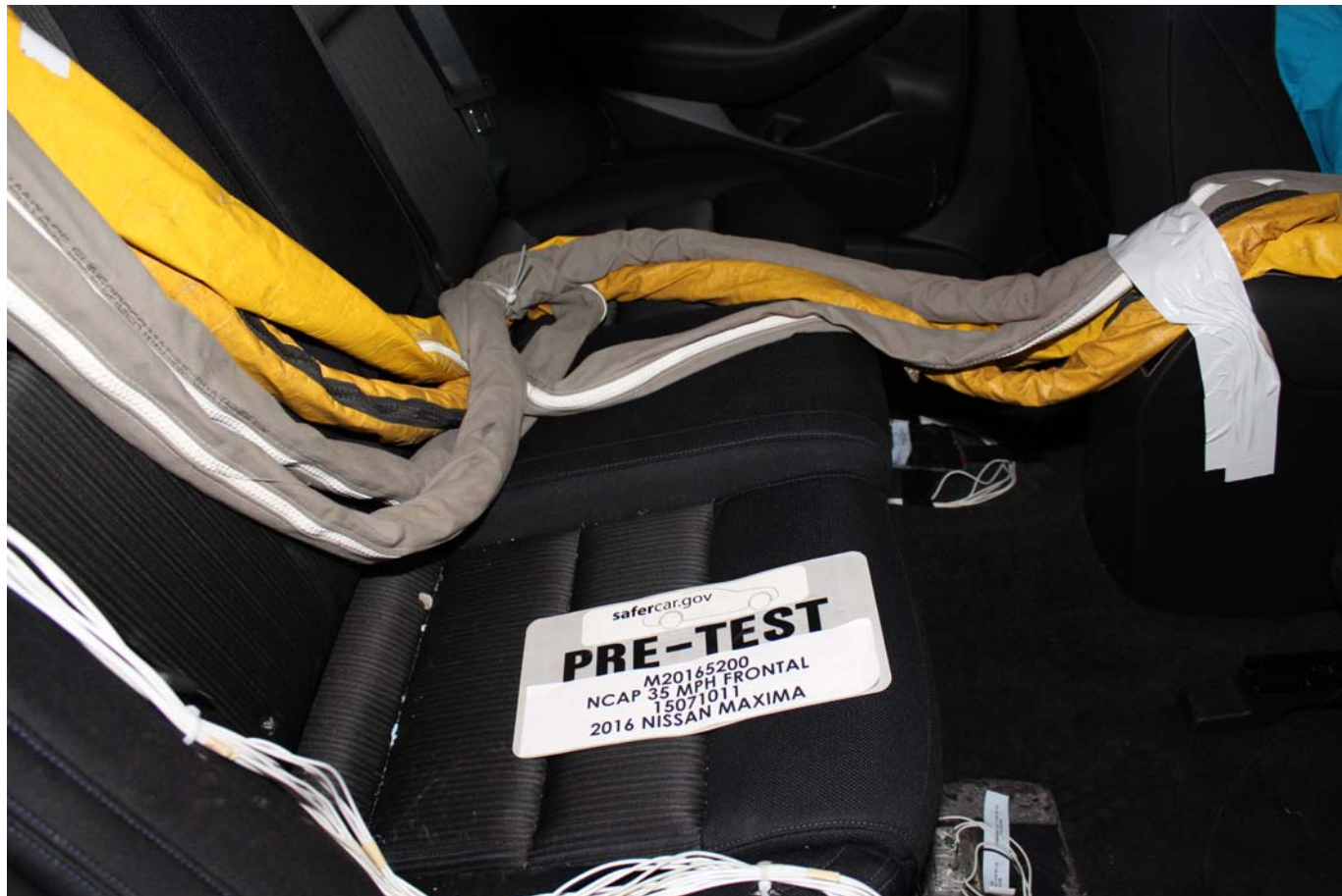
Photo No. 027 - Pre-Test Dummy Cable Routing
