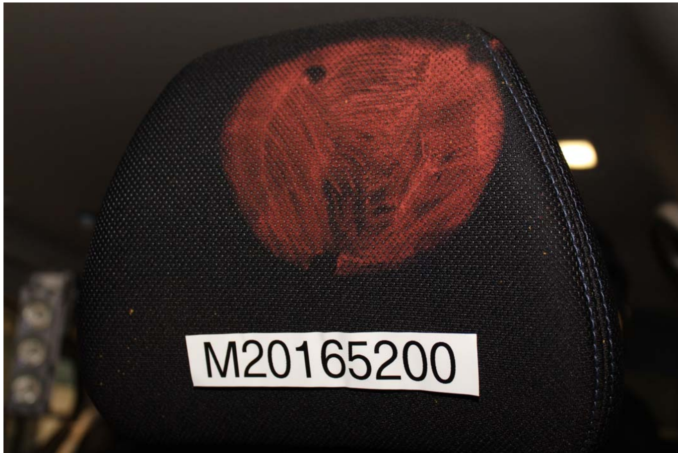
Photo No. 047 - Post-Test Driver Dummy Contact with Headrest
