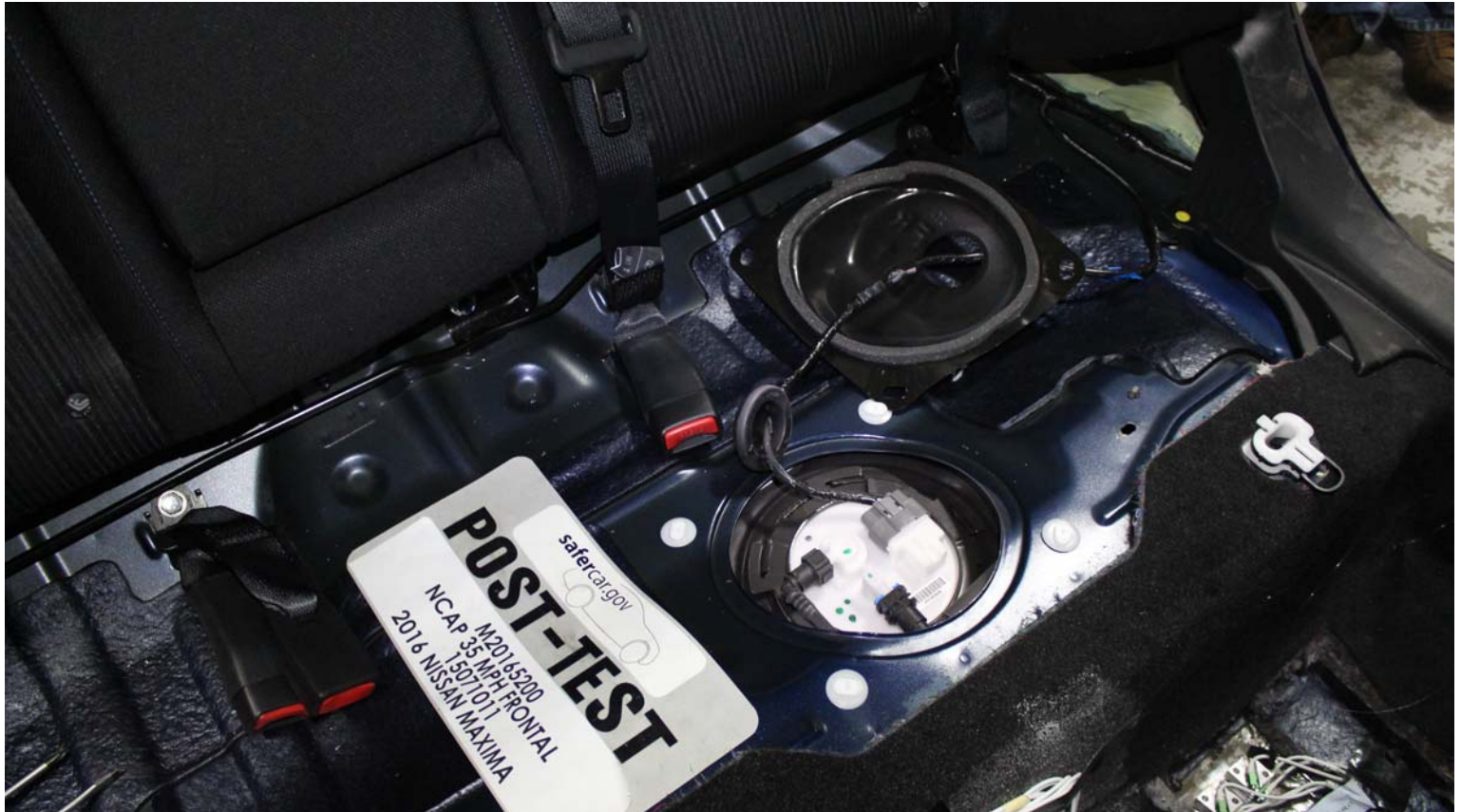
Photo No. 070 - Post-Test Stoddard Solvent Spillage Location View
