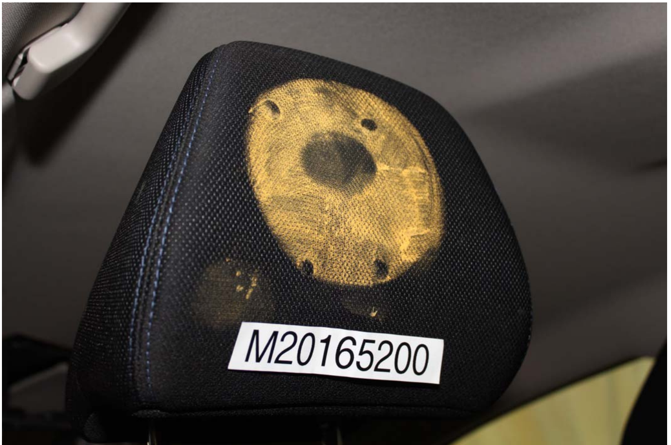
Photo No. 068 - Post-Test Passenger Dummy Contact with Headrest
