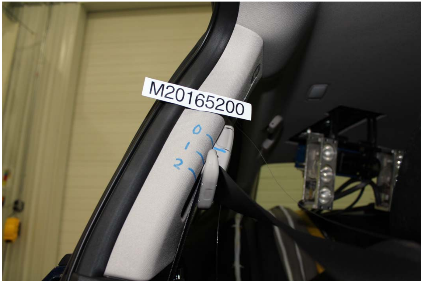
Photo No. 058 - Pre-Test View of Belt Anchorage for Passenger Dummy
