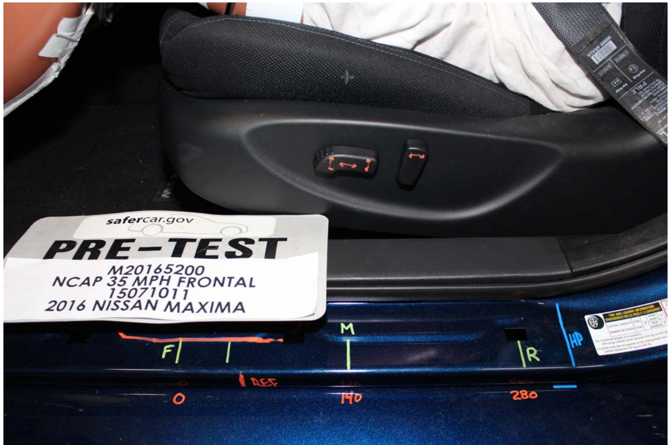
Photo No. 035 - Pre-Test Driver's Seat Fore-Aft Markings
