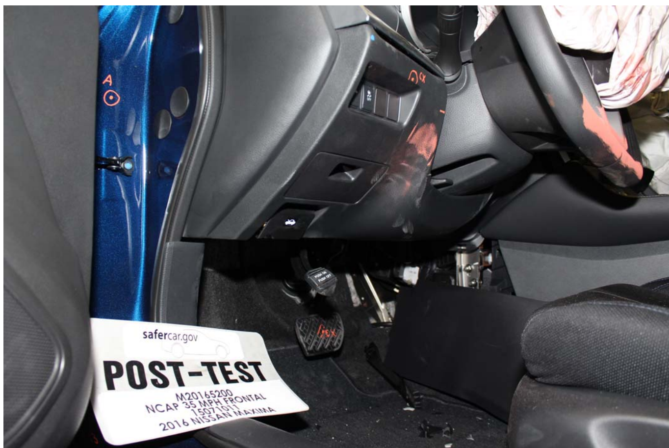
Photo No. 042 - Post-Test Driver's Side Knee Bolster (without dummy)
