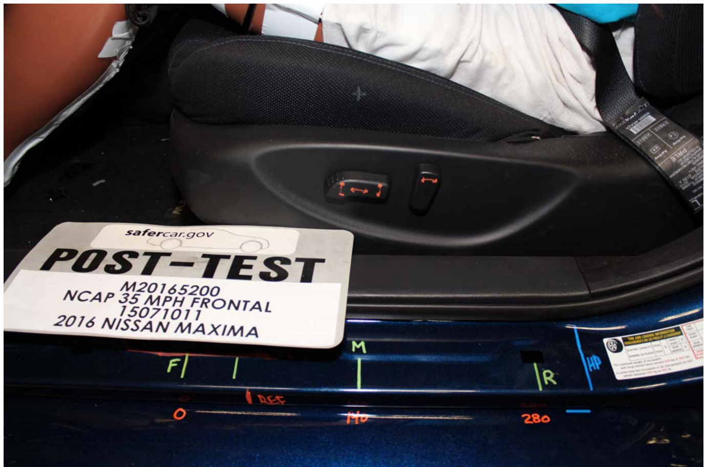
Photo No. 036 - Post-Test Driver's Seat Fore-Aft Markings
