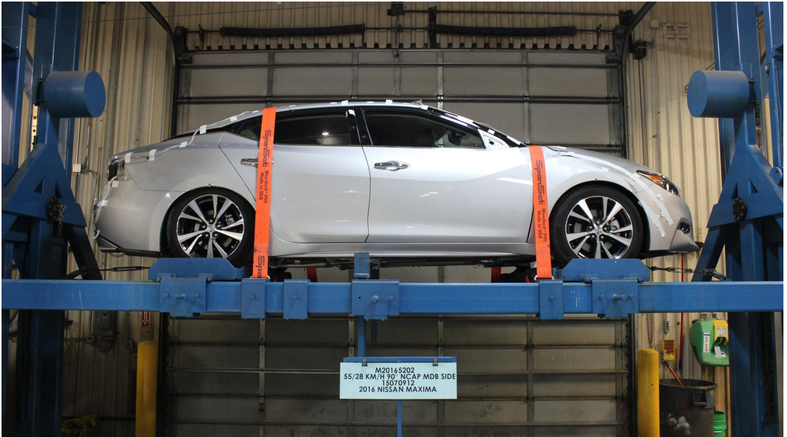
Photo No. 100 - FMVSS No. 301 Static Rollover 360 Degrees
