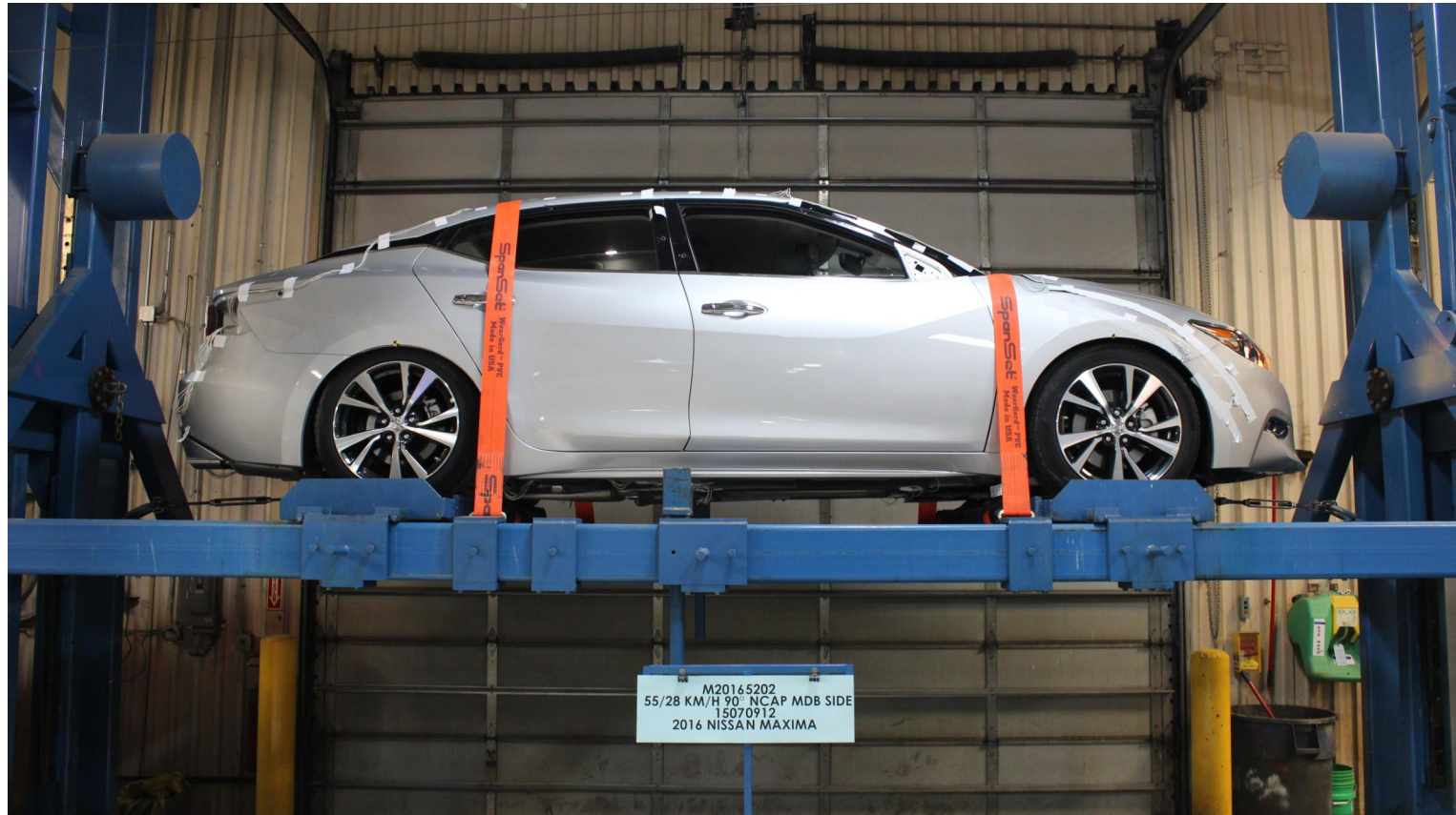
Photo No. 096 - FMVSS No. 301 Static Rollover 0 Degrees
