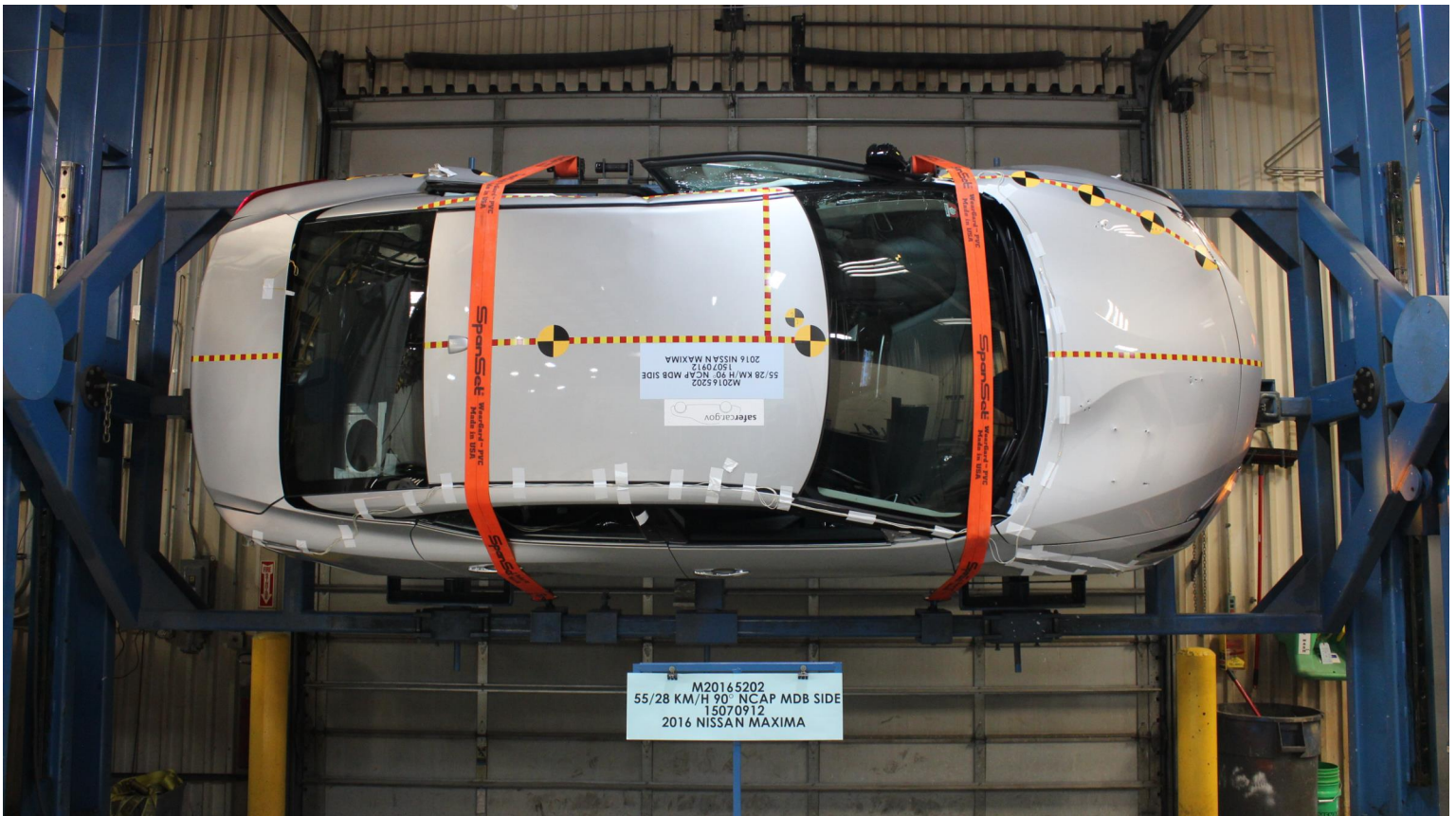
Photo No. 099 - FMVSS No. 301 Static Rollover 270 Degrees
