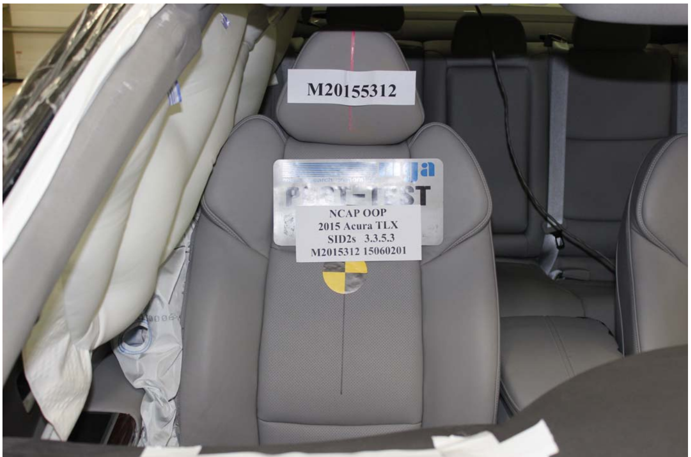
Photo No. 24 - Post-Test Curtain Airbag Front View
