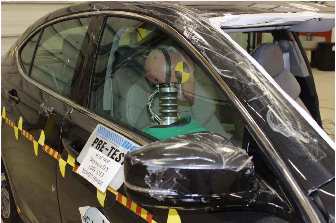
Photo No. 17 - Pre-Test SID-IIs Dummy Right \frac{3}{4} Front View
