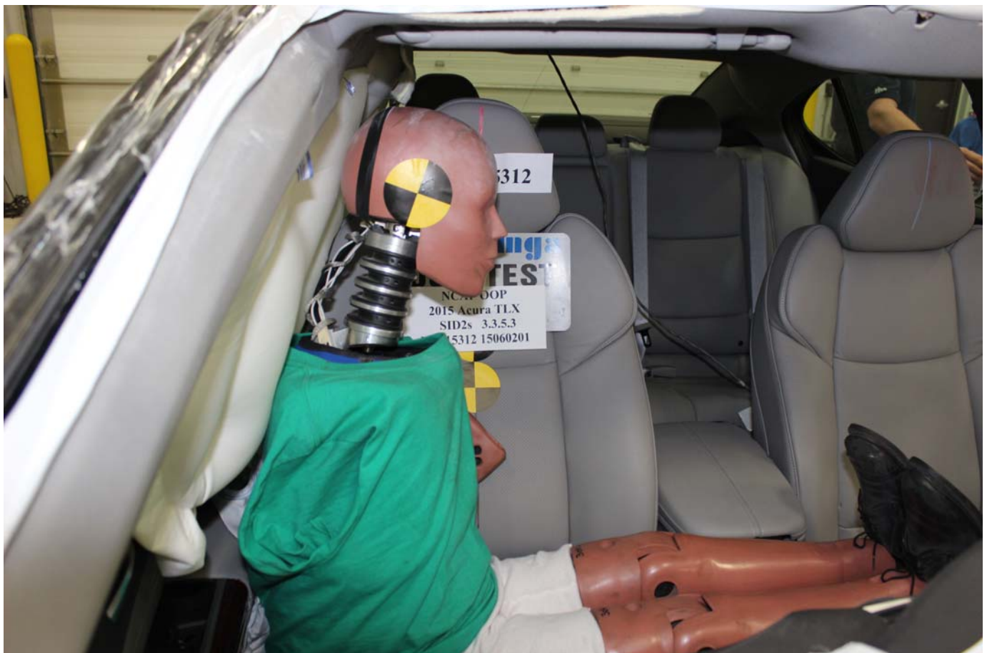
Photo No. 14 - Post-Test SID-IIs Dummy Front View
