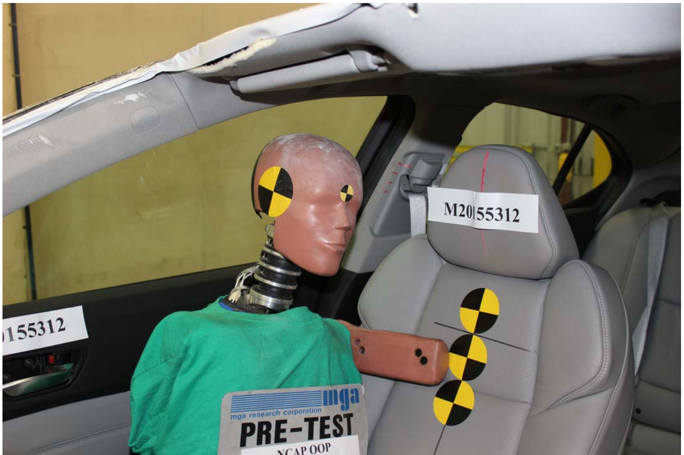
Photo No. 11 - Pre-Test SID-11s Dummy Left 3/4 Front Closeup View
