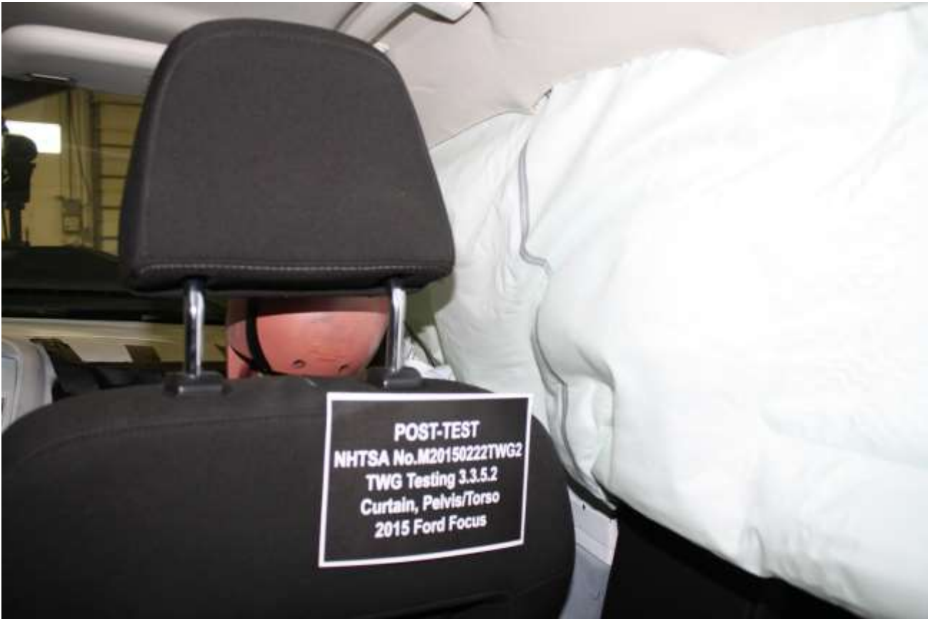
Figure A-23: Post-Test Curtain Airbag Rear Right Side View
