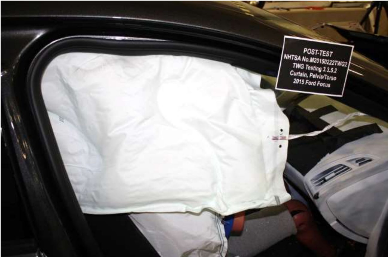
Figure A-22: Post-Test Curtain Airbag Right Side View
