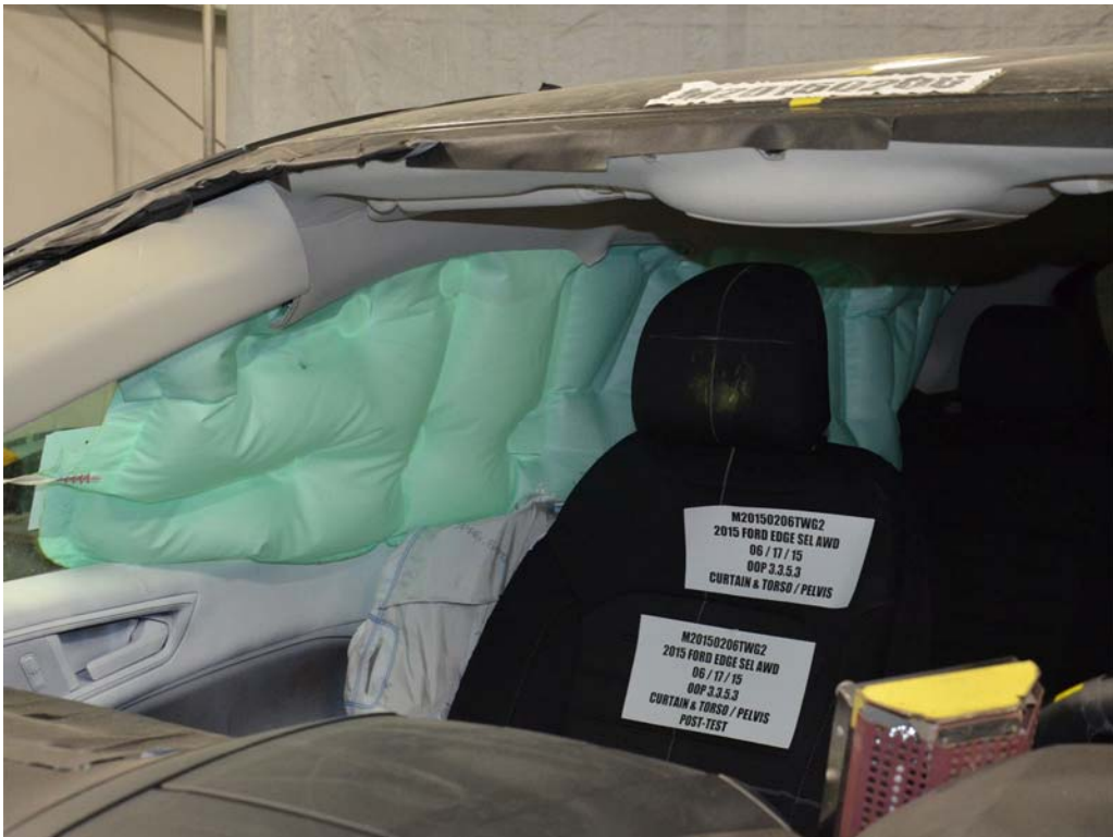
FIGURE 16. Post-Test Airbags, Left Front ¾ View
