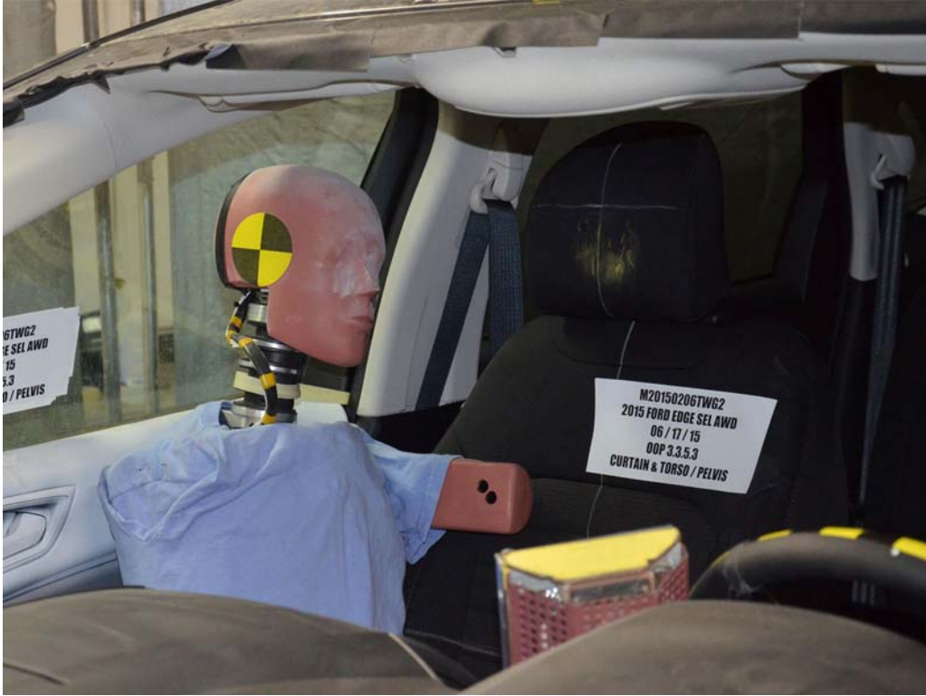
FIGURE 9. Pre-Test Dummy Position, \frac{3}{4} View
