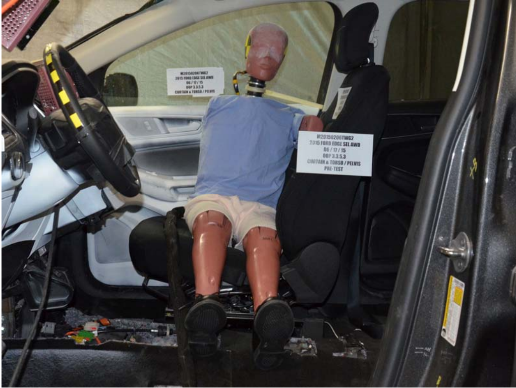
FIGURE 7. Pre-Test Dummy Position, Left Side View
