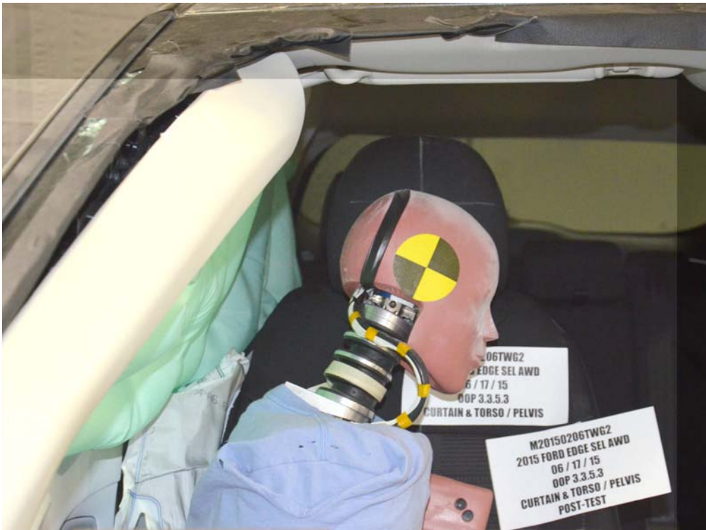
FIGURE 12. Post-Test Dummy Position, Front View
