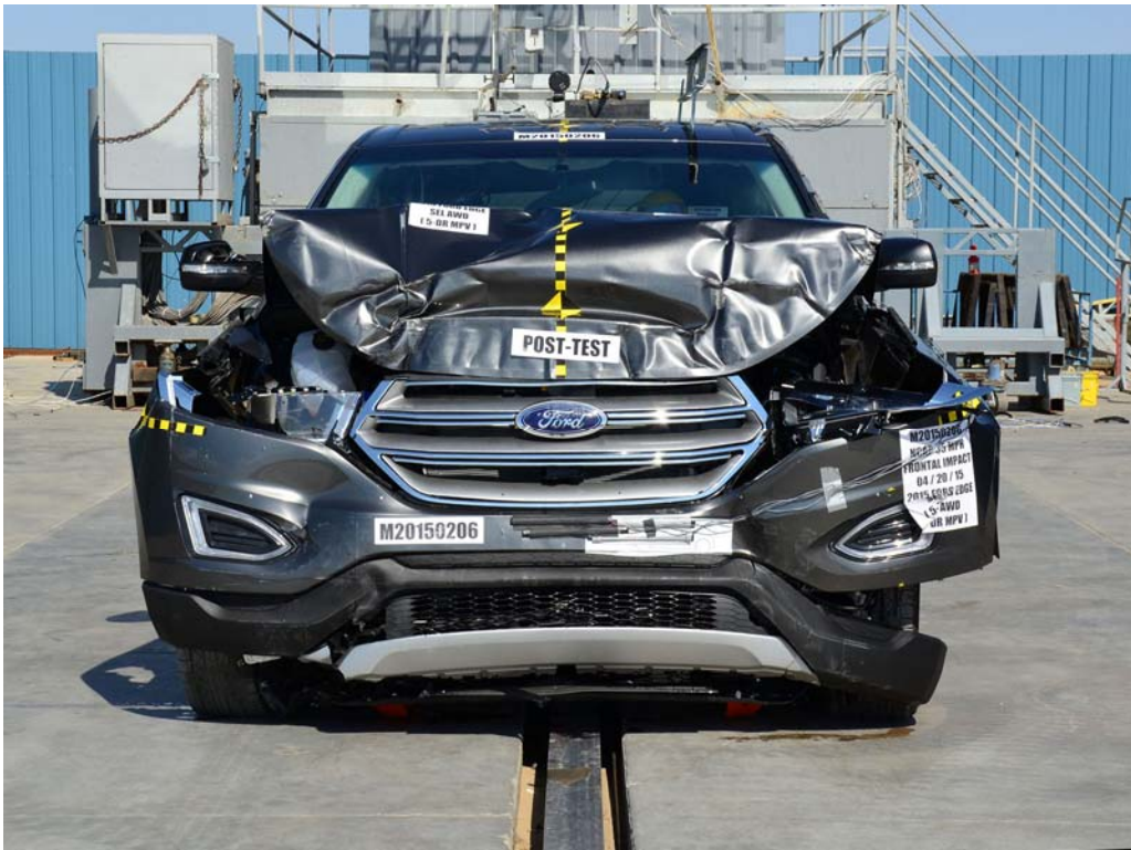
FIGURE 4. Post-Test Front View of NCAP Frontal Impact Test
