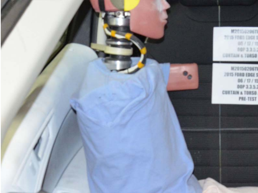
FIGURE 13. Pre-Test Dummy Position, Close-Up Front View
