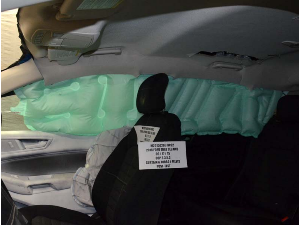
FIGURE 15. Post-Test Airbags, Left Side View
