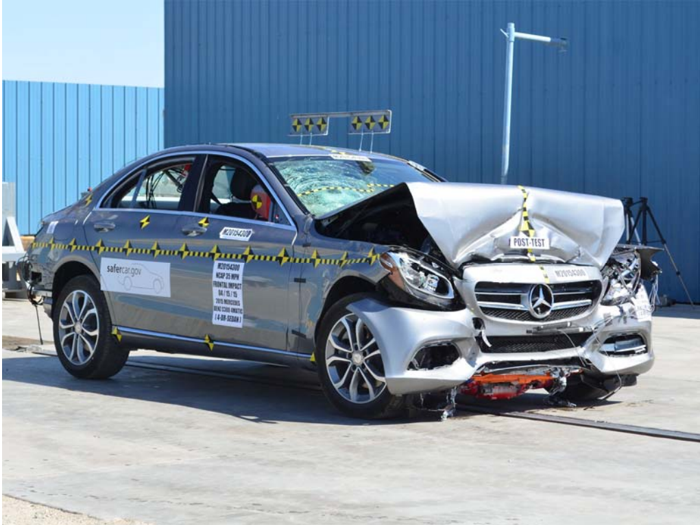
FIGURE 3. Post-Test Right Front ¾ View of NCAP Frontal Impact Test
