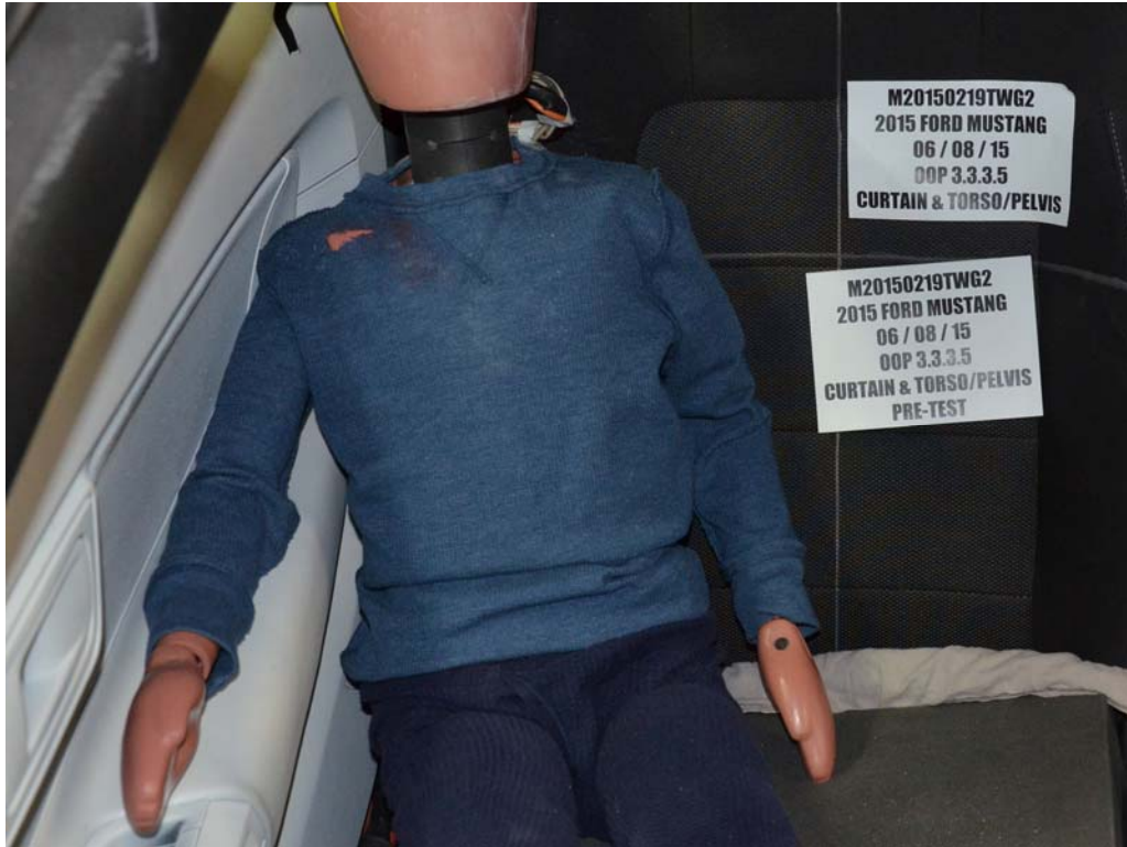
FIGURE 13. Pre-Test Dummy Position, Close-Up Front View
