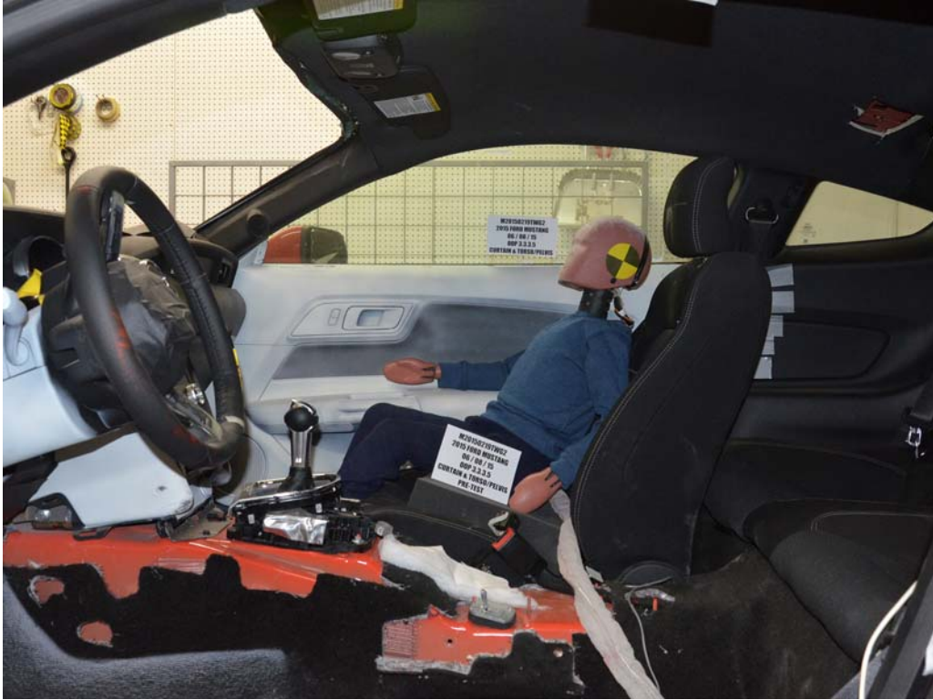
FIGURE 7. Pre-Test Dummy Position, Left Side View
