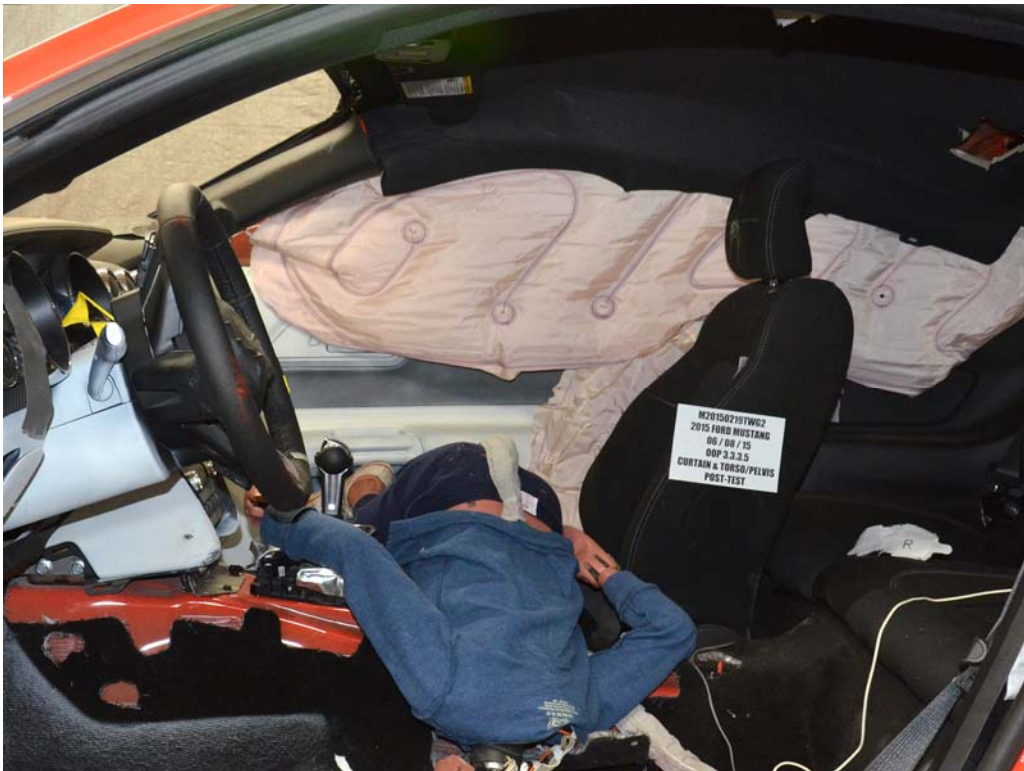
FIGURE 8. Post-Test Dummy Position, Left Side View
