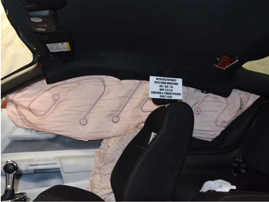
FIGURE 15. Post-Test Airbags, Left Side View
