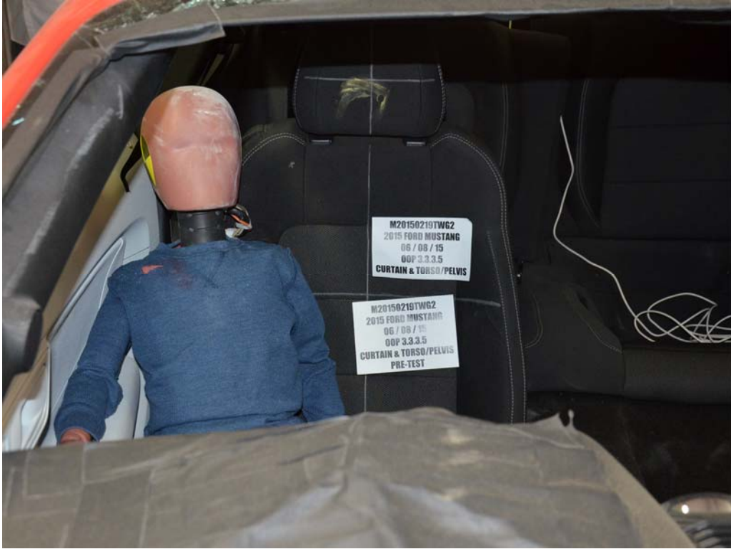
FIGURE 11. Pre-Test Dummy Position, Front View
