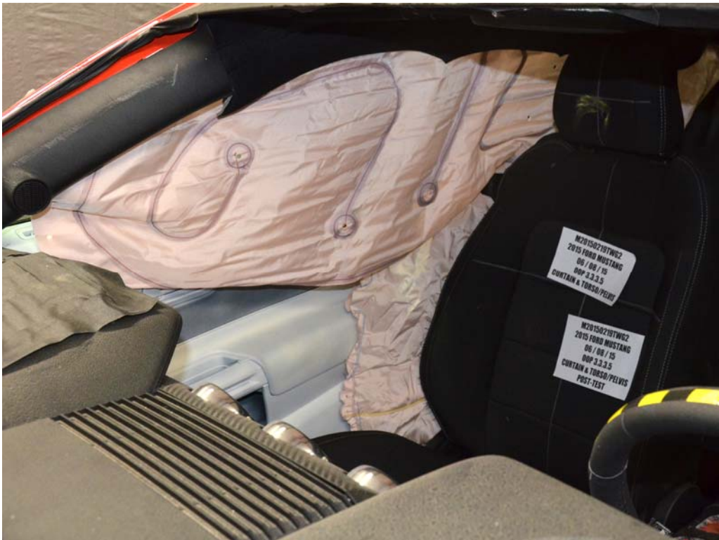
FIGURE 16. Post-Test Airbags, Left Front ¾ View
