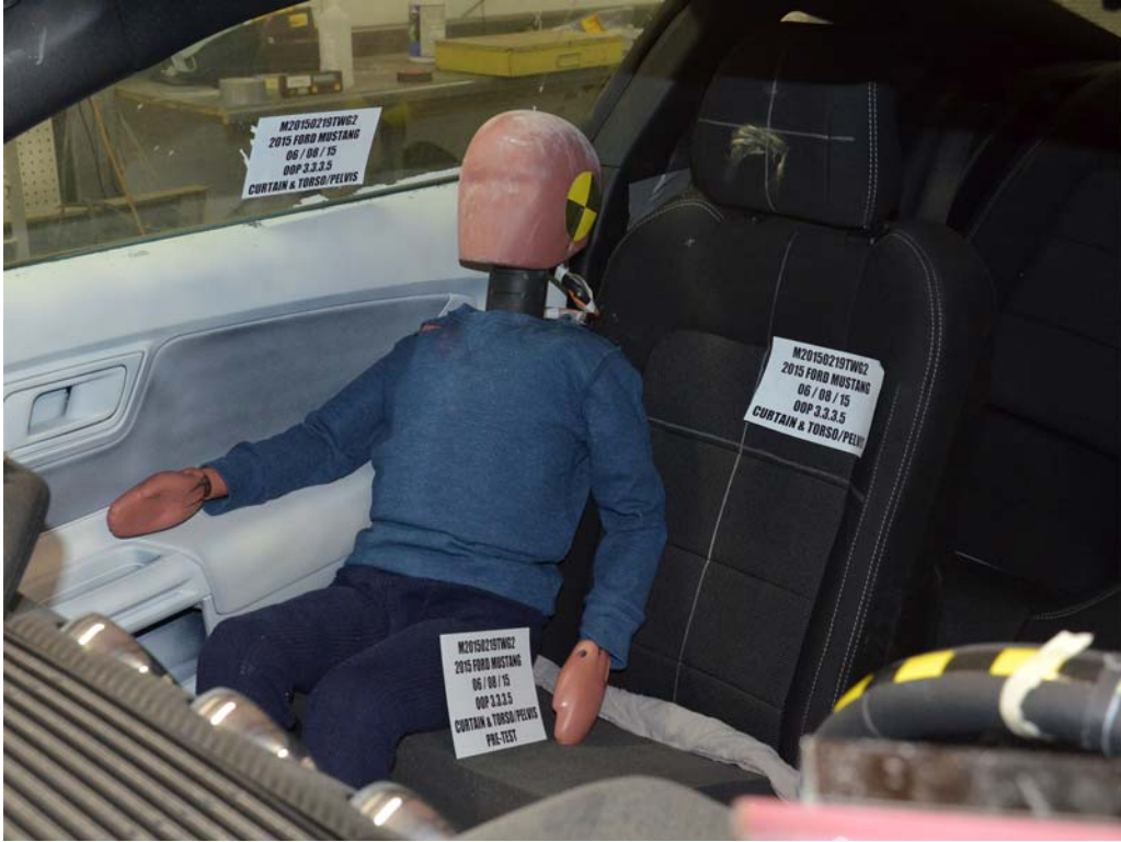
FIGURE 9. Pre-Test Dummy Position, \frac{3}{4} View
