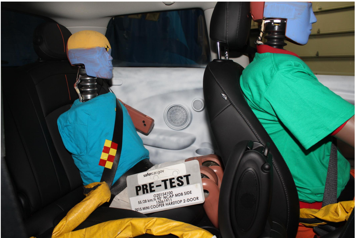
Photo No. 071 - Pre-Test Right Side View of Rear Passenger Dummy and Rear Seat Occupant
