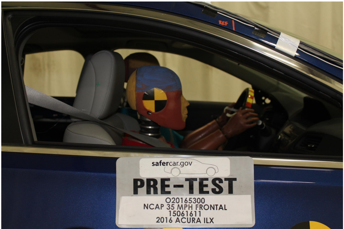
Photo No. 052 - Pre-Test Passenger Dummy Window View
