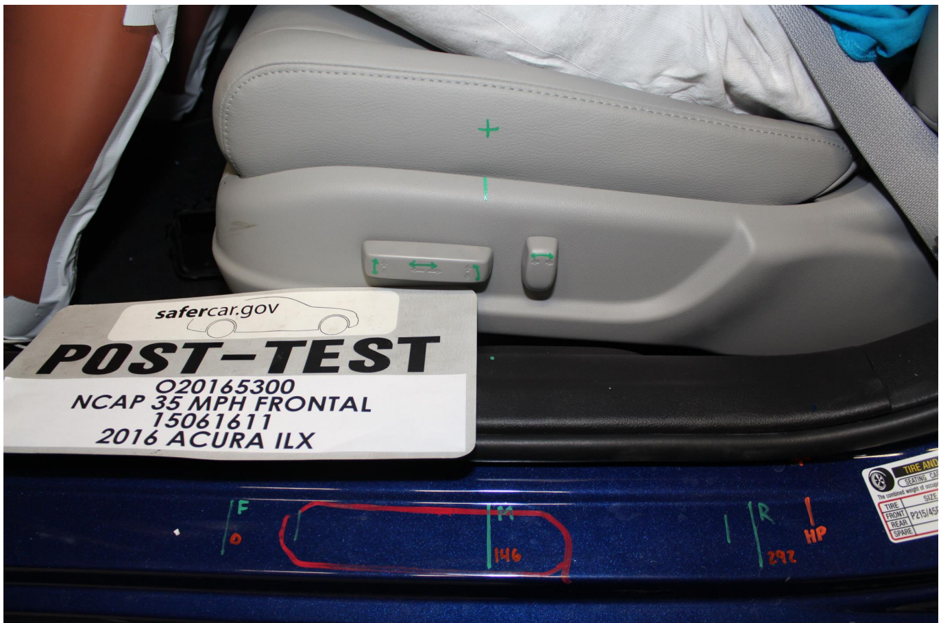
Photo No. 036 - Post-Test Driver's Seat Fore-Aft Markings
