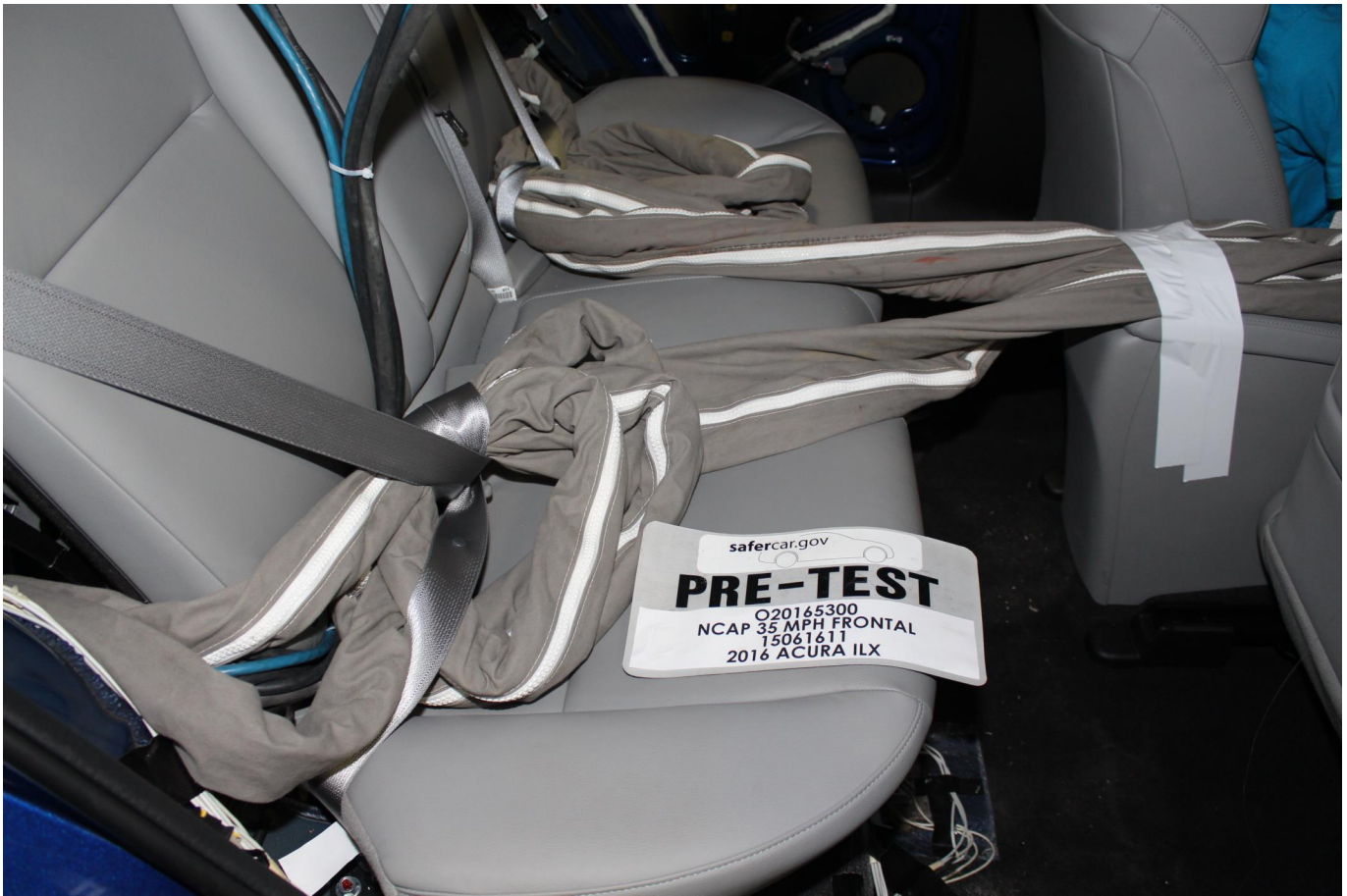
Photo No. 027 - Pre-Test Dummy Cable Routing
