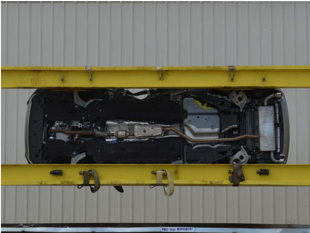
FIGURE 66. FMVSS No. 301 Static Rollover 270 Degrees
