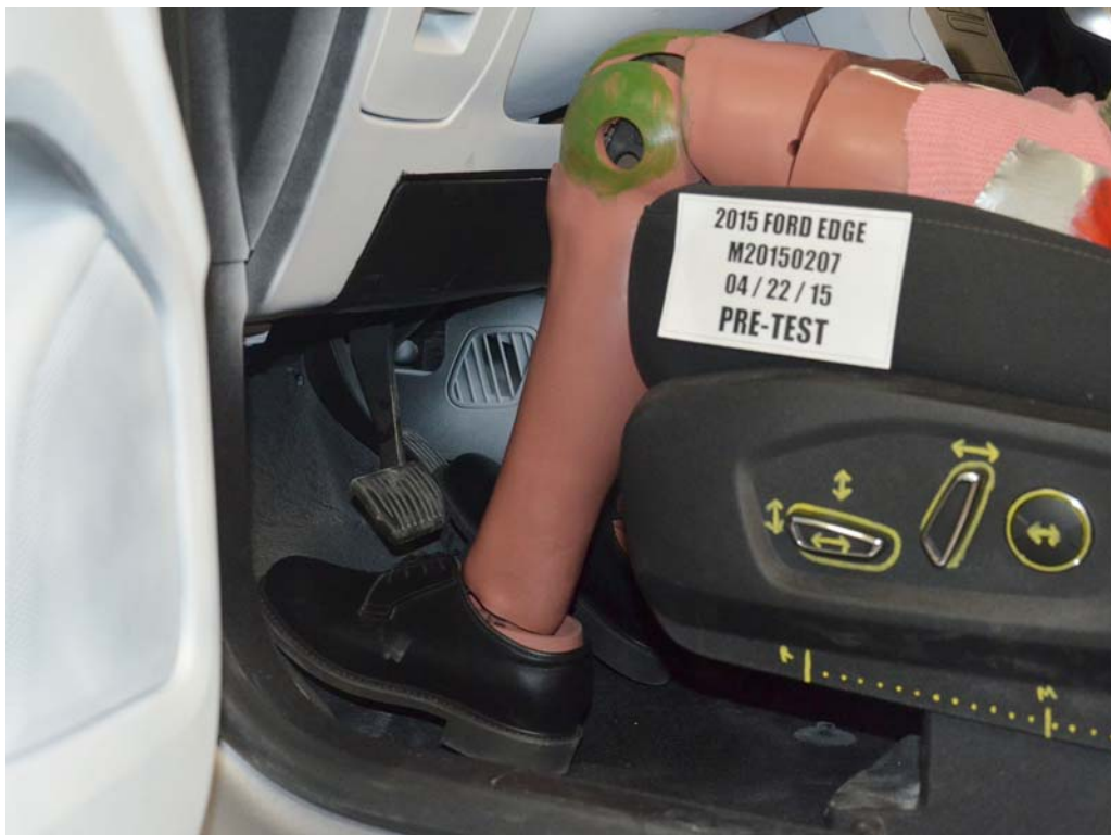
FIGURE 32. Pre-Test Placement of Dummy's Feet
