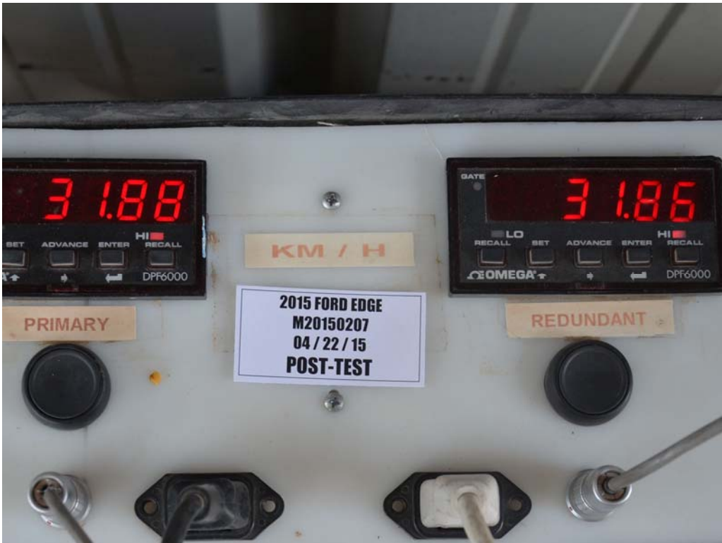
FIGURE 62. Post-Test Primary and Redundant Speed Trap Read-Out
