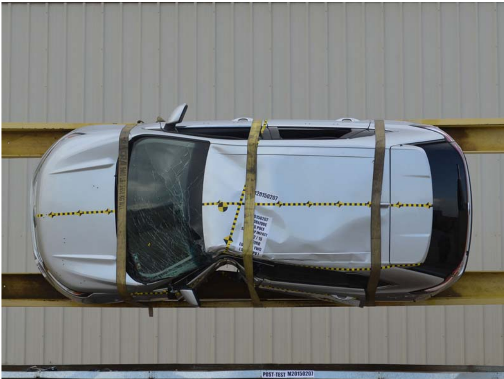
FIGURE 64. FMVSS No. 301 Static Rollover 90 Degrees
