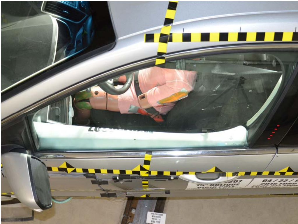
FIGURE 40. Pre-Test Dummy and Door Clearance View
