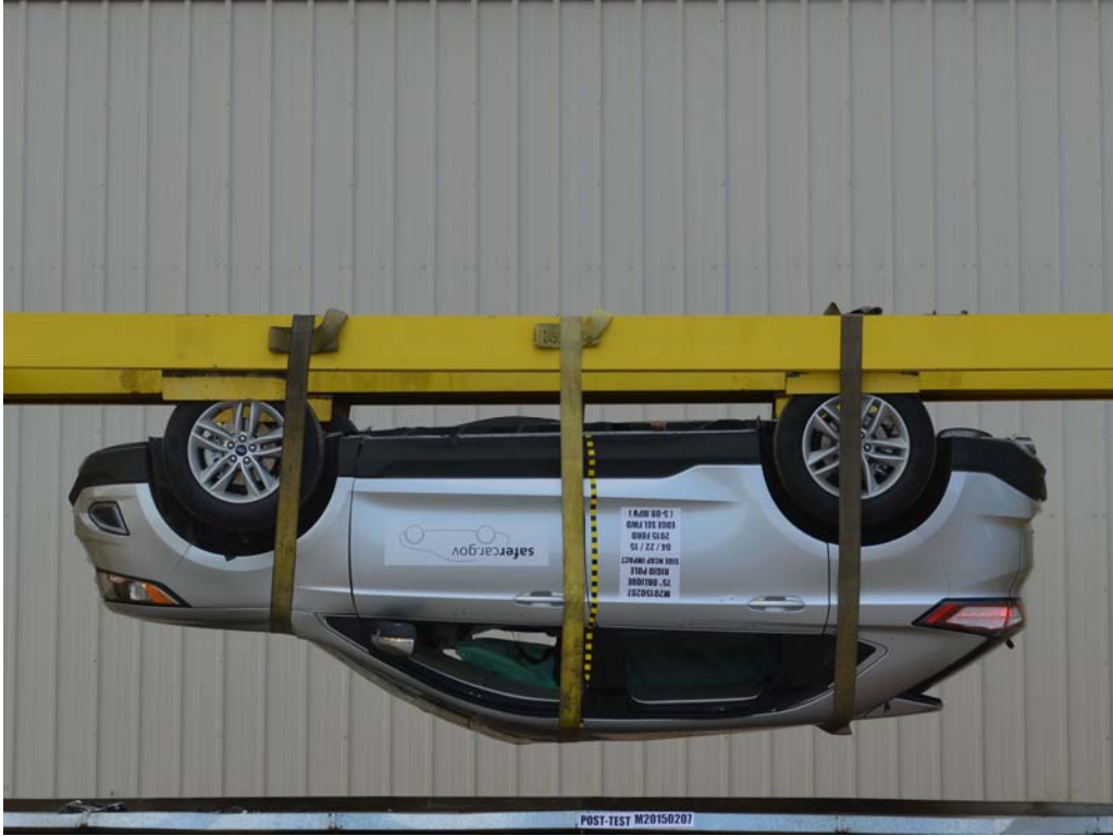
FIGURE 65. FMVSS No. 301 Static Rollover 180 Degrees
