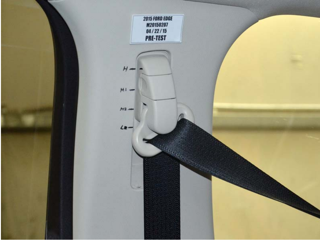
FIGURE 33. Pre-Test View of Belt Anchorage for Dummy
