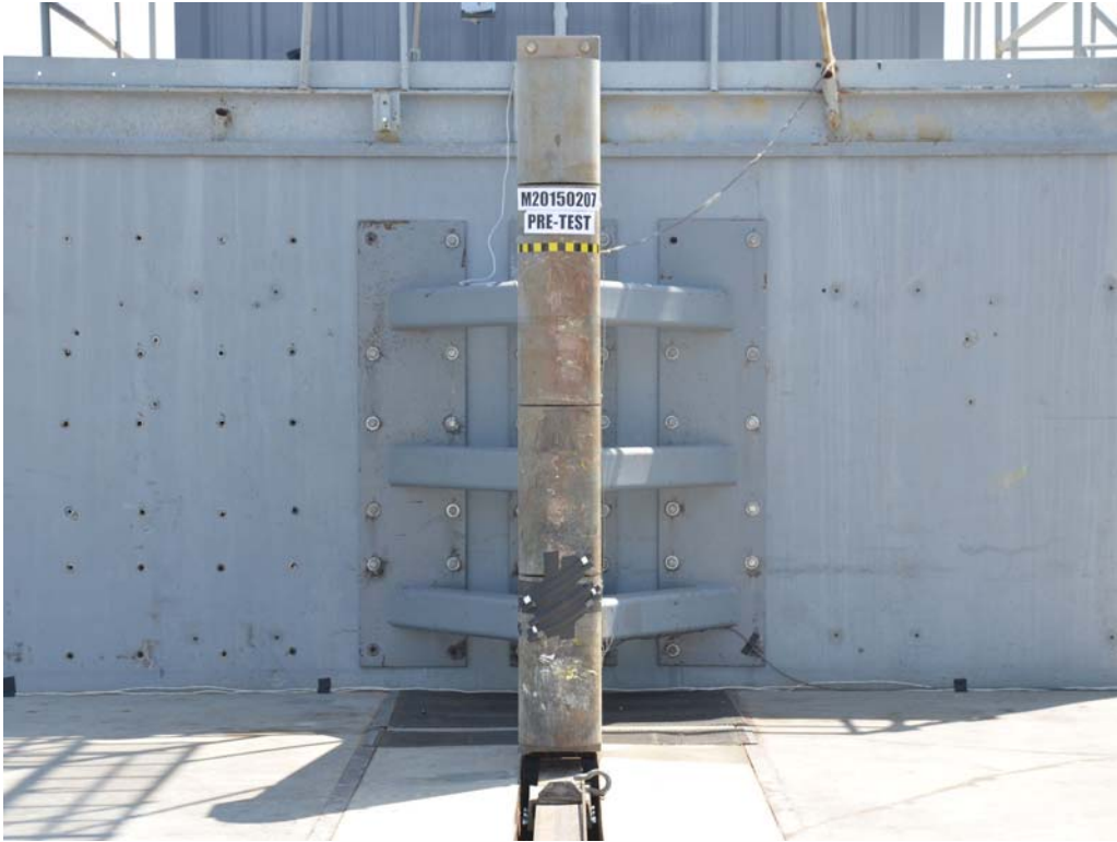
FIGURE 57. Pre-Test Pole Barrier Front View
