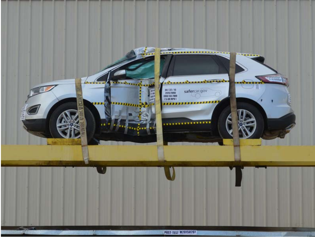
FIGURE 67. FMVSS No. 301 Static Rollover 360 Degrees
