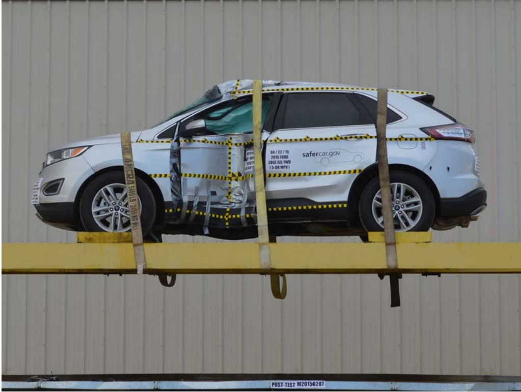
FIGURE 63. FMVSS No. 301 Static Rollover 0 Degrees
