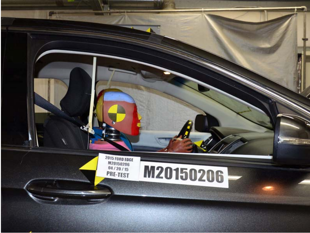
FIGURE 52. Pre-Test Passenger Dummy Window View
