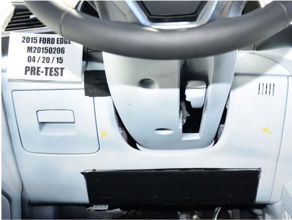
FIGURE 41. Pre-Test Driver's Side Knee Bolster
