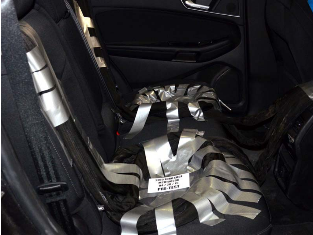
FIGURE 27. Pre-Test Dummy Cable Routing
