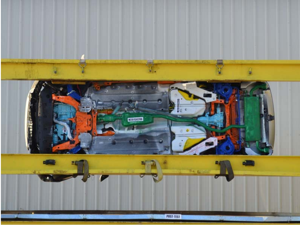
FIGURE 75. Vehicle at 270° on Static Rollover Device
