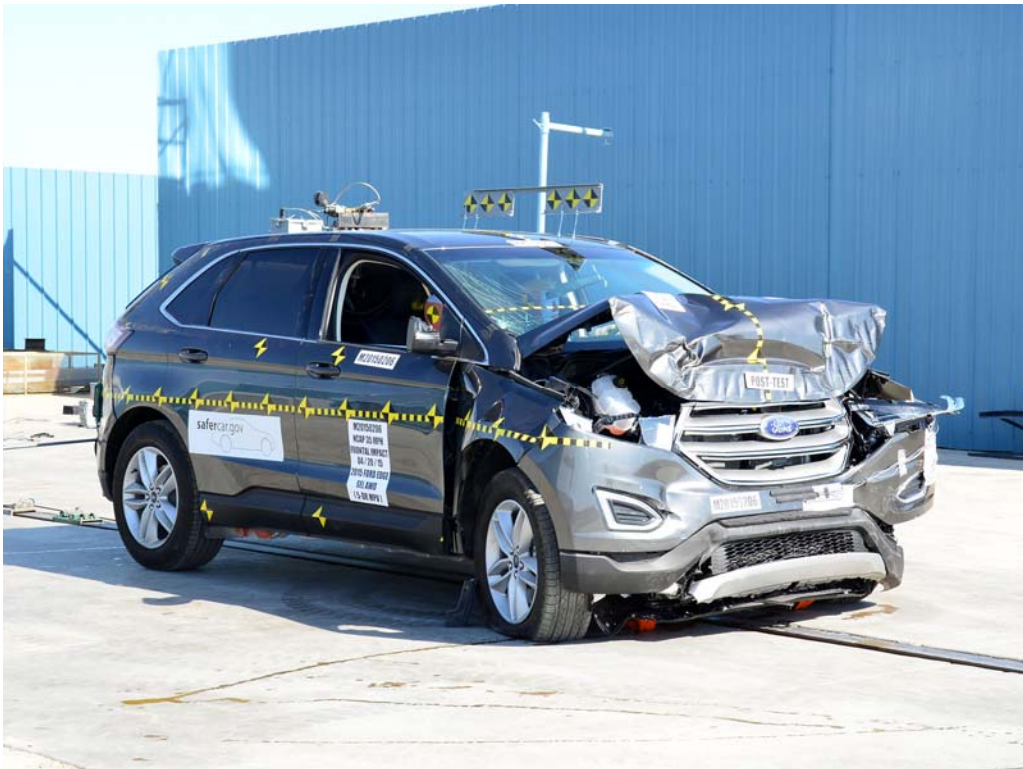
FIGURE 14. Post-Test Right Front \frac{3}{4} View
