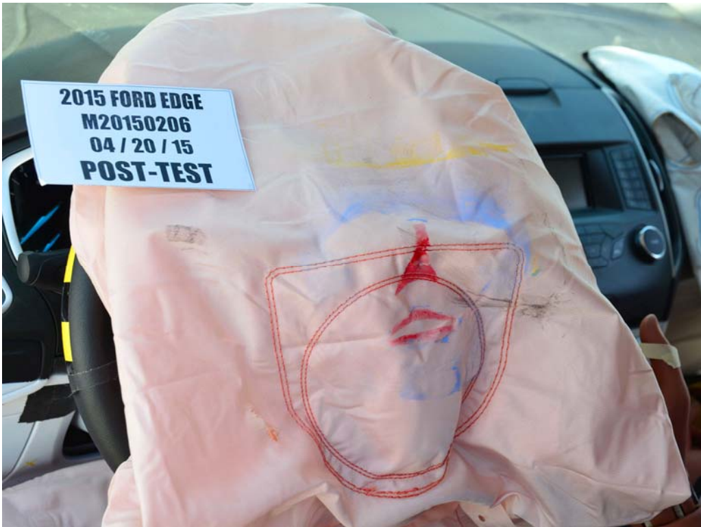
FIGURE 46. Post-Test Driver Dummy Contact with Airbag
