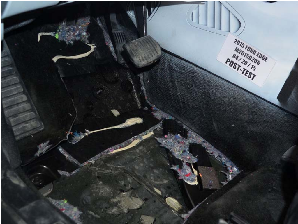
FIGURE 44. Post-Test Driver's Side Floorpan
