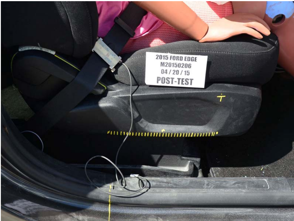
FIGURE 57. Post-Test Passenger's Seat Fore-Aft Markings
