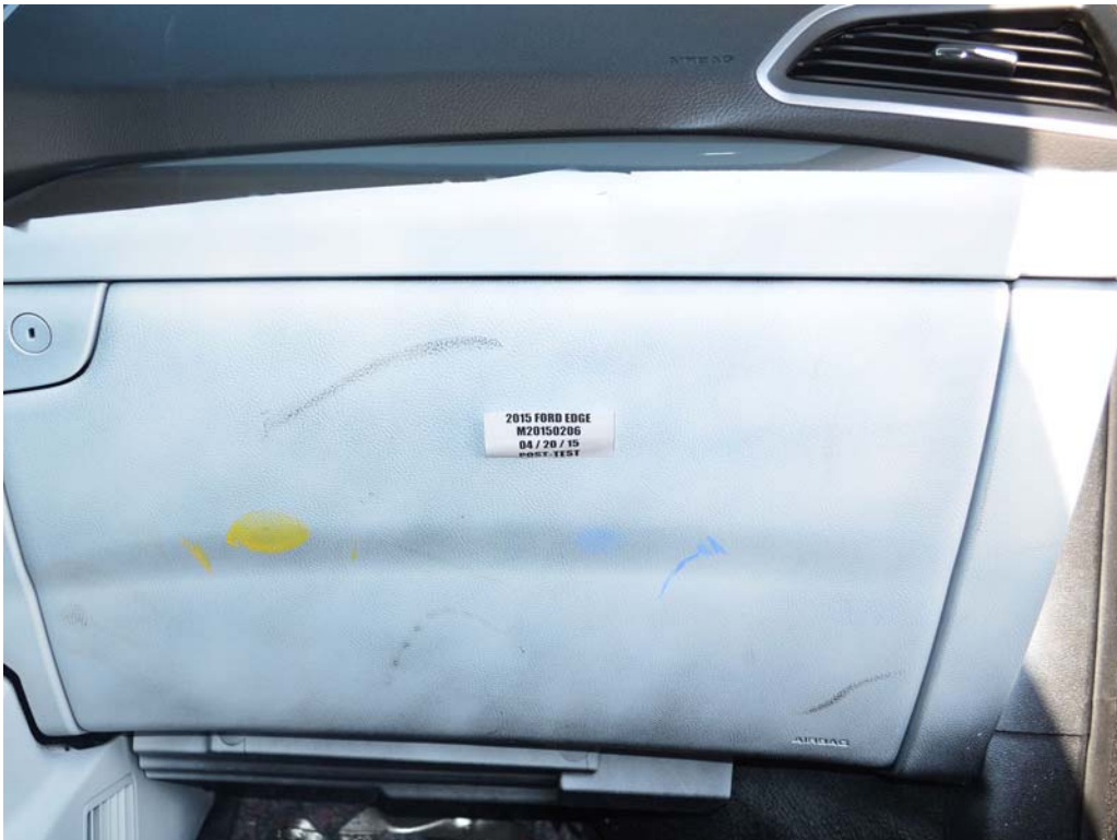
FIGURE 68a. Post-Test Passenger Dummy Contact with Glovebox
