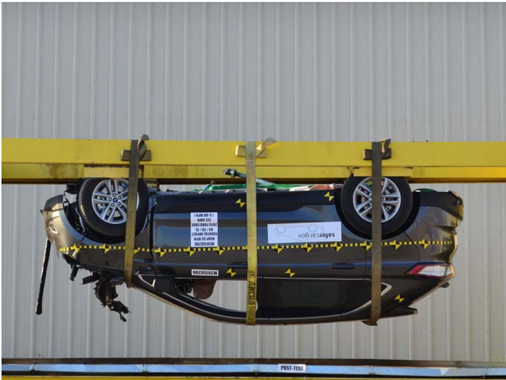
FIGURE 74. Vehicle at 180° on Static Rollover Device
