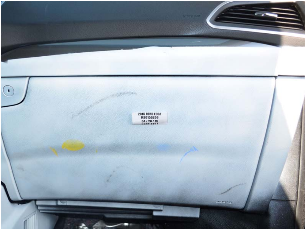
FIGURE 63. Post-Test Passenger's Side Knee Bolster
