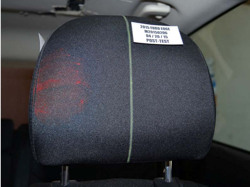
FIGURE 47. Post-Test Driver Dummy Contact with Headrest
