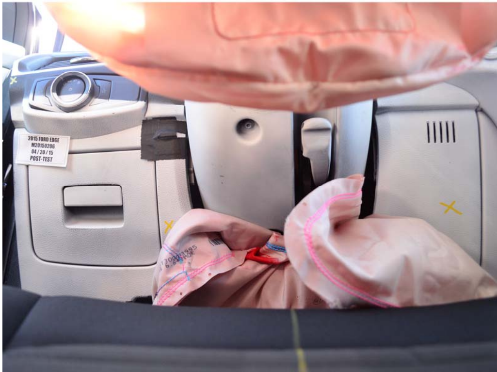
FIGURE 42. Post-Test Driver's Side Knee Bolster
