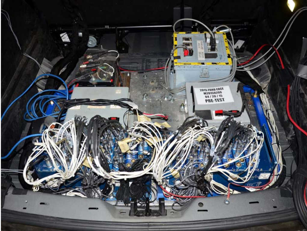
FIGURE 69. Photograph of Ballast Installed in Vehicle
