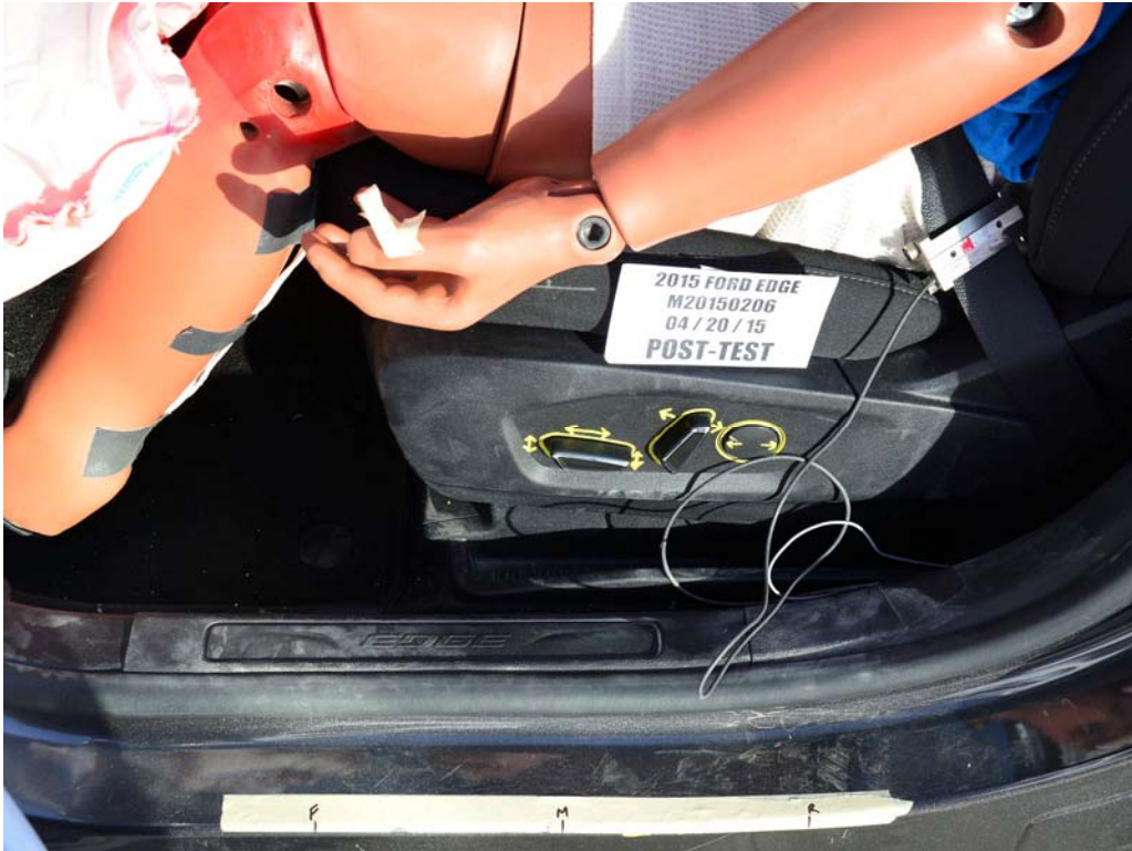
FIGURE 36. Post-Test Driver's Seat Fore-Aft Markings
