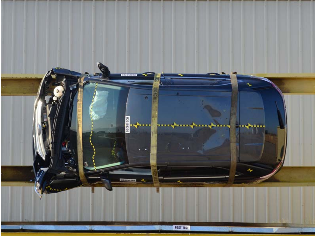
FIGURE 73. Vehicle at 90° on Static Rollover Device
