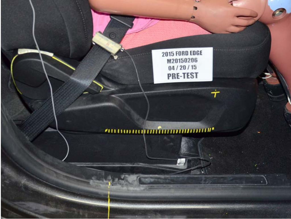
FIGURE 56. Pre-Test Passenger's Seat Fore-Aft Markings
