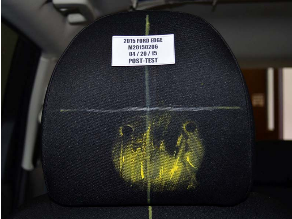
FIGURE 68. Post-Test Passenger Dummy Contact with Headrest
