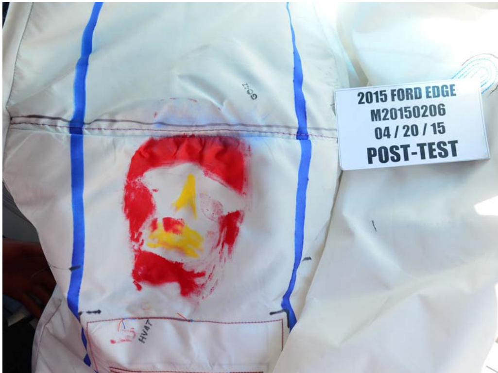
FIGURE 67. Post-Test Passenger Dummy Contact with Airbag
