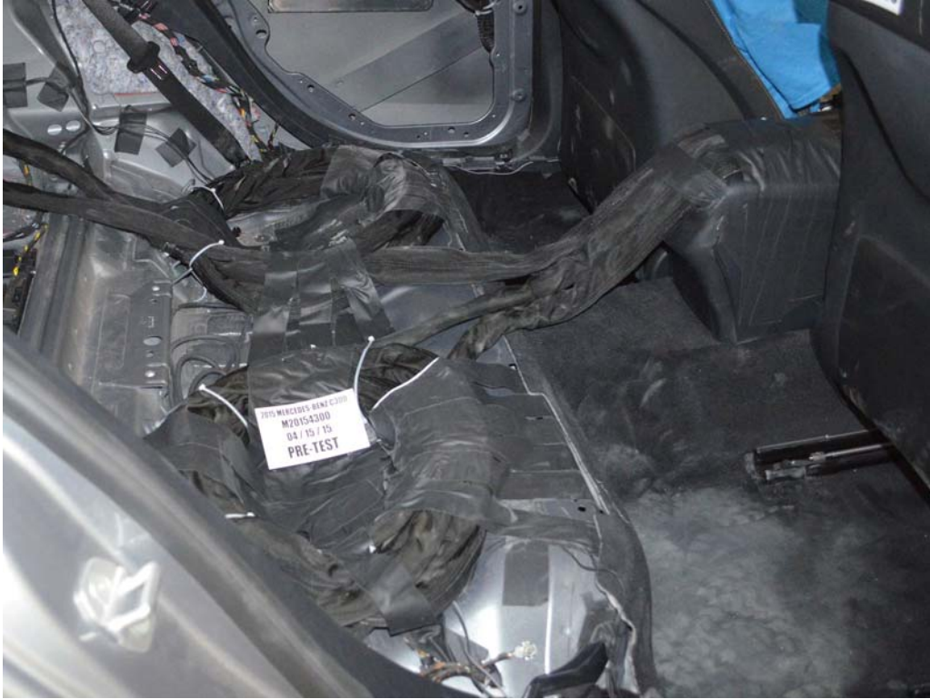
FIGURE 27. Pre-Test Dummy Cable Routing
