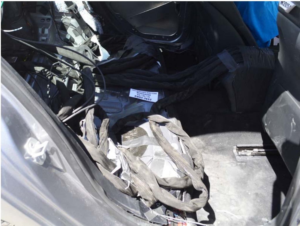
FIGURE 28. Post-Test Dummy Cable Routing
