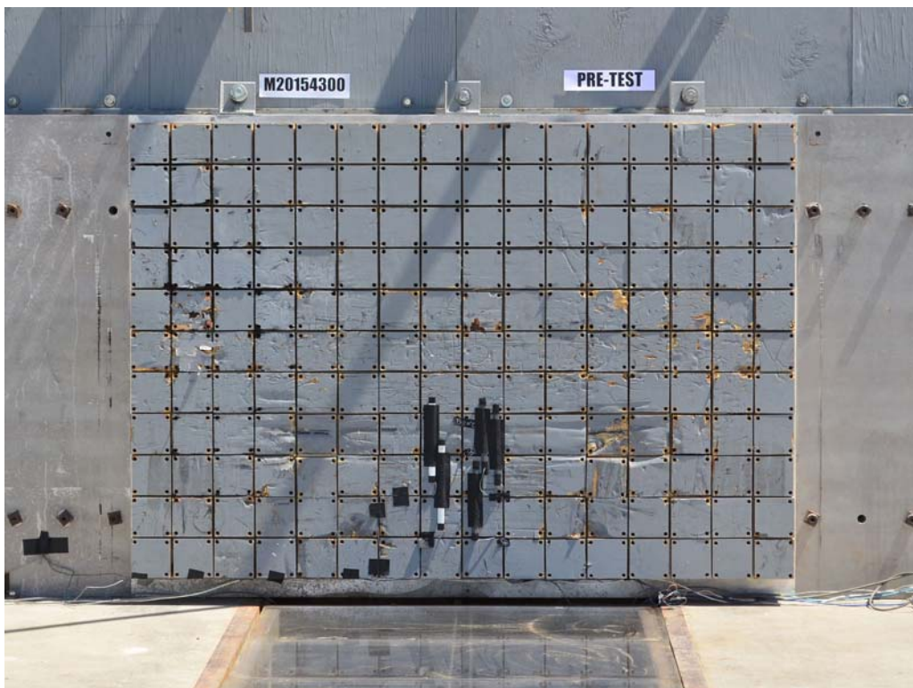
FIGURE 2. Load Cell Wall
