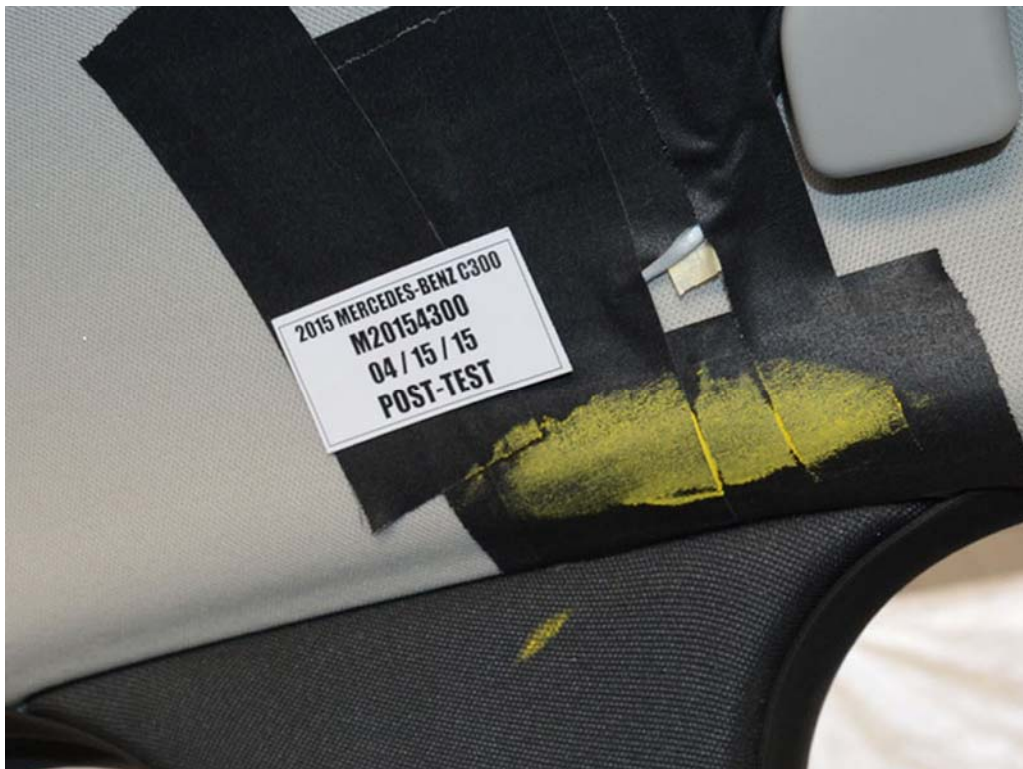
FIGURE 47a. Post-Test Driver Dummy Contact with Headliner
