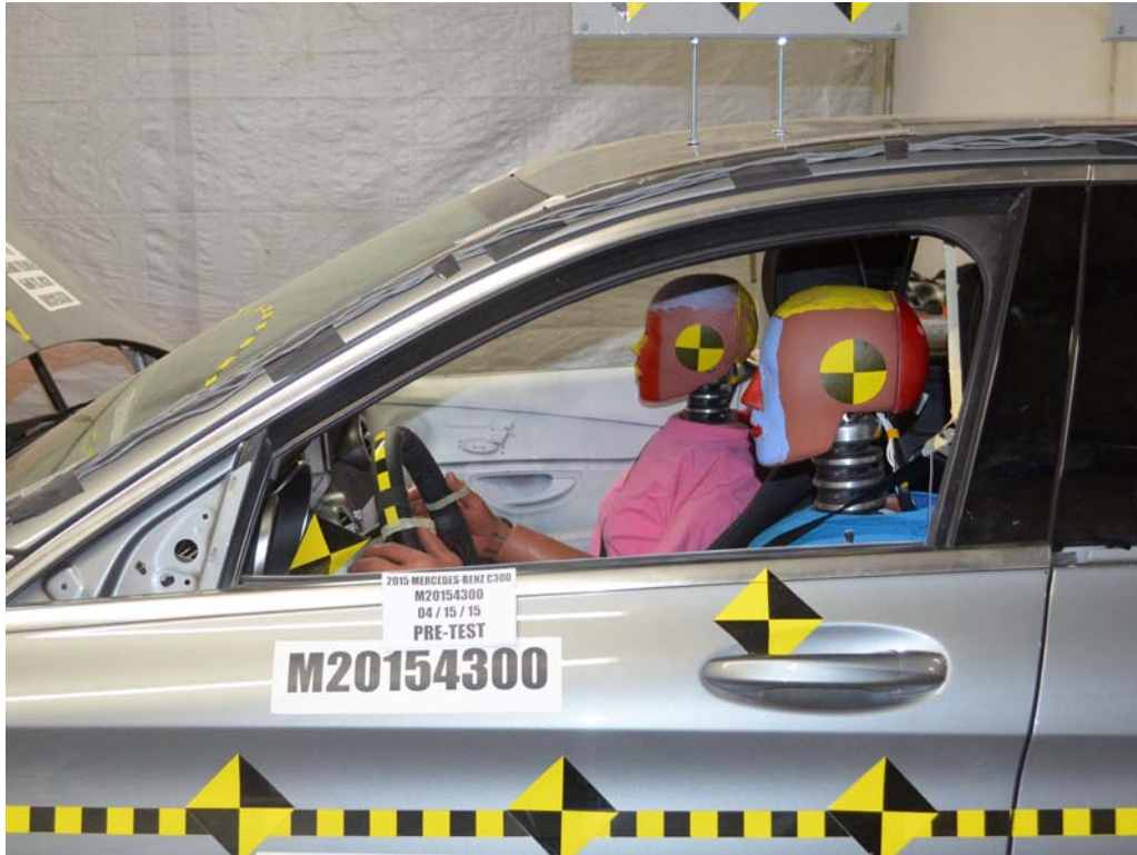
FIGURE 31. Pre-Test Driver Dummy Window View
