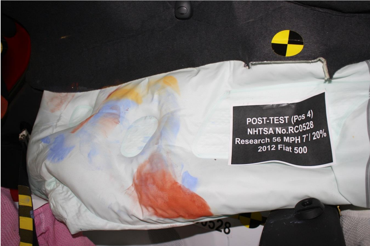
No. 100 Post-Test View of Passenger Dummy Head contact with Airbag
