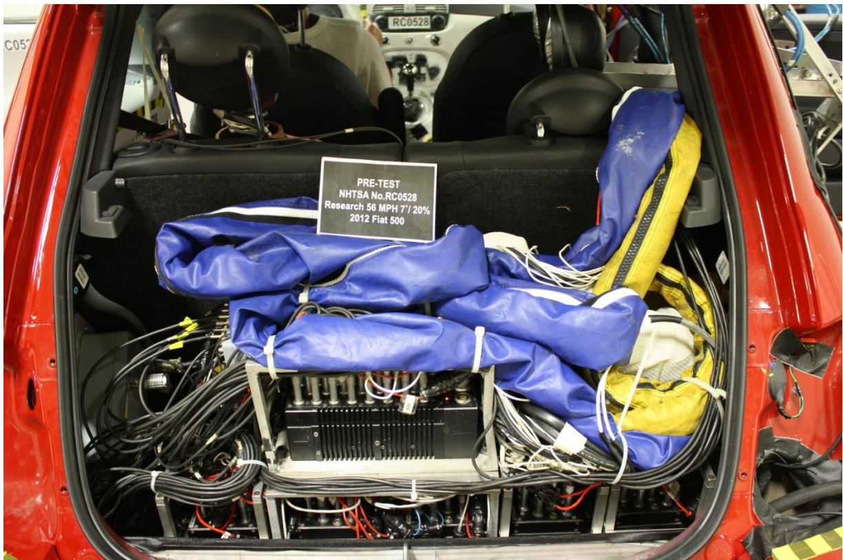
No. 103 Pre-Test Ballast Locations
