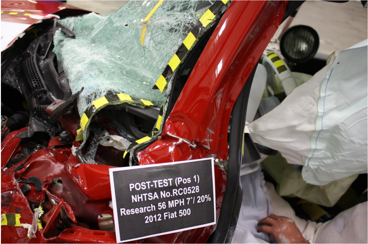
No. 127 Post-Test View of Windshield Separation
