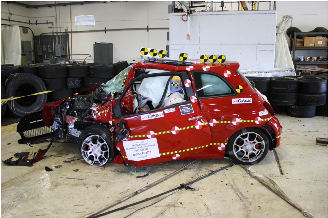
No. 010 Post-Test Left Side View of Test Vehicle
