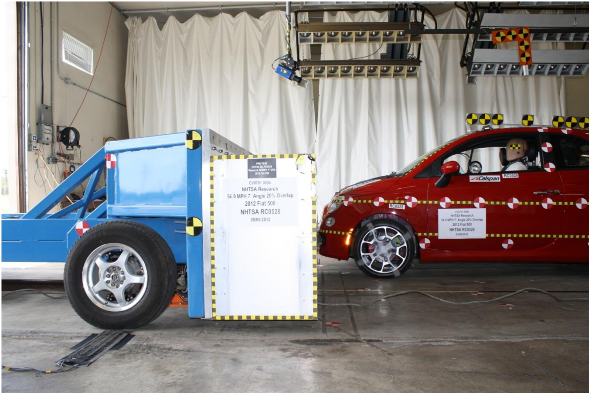
No. 021 Pre-Test Right Side View of RMDB against target vehicle at ideal Impact Point
