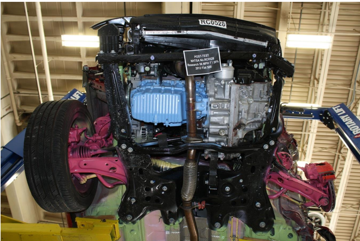
No. 116 Post-Test View of Front Sub-Frame Deformation
