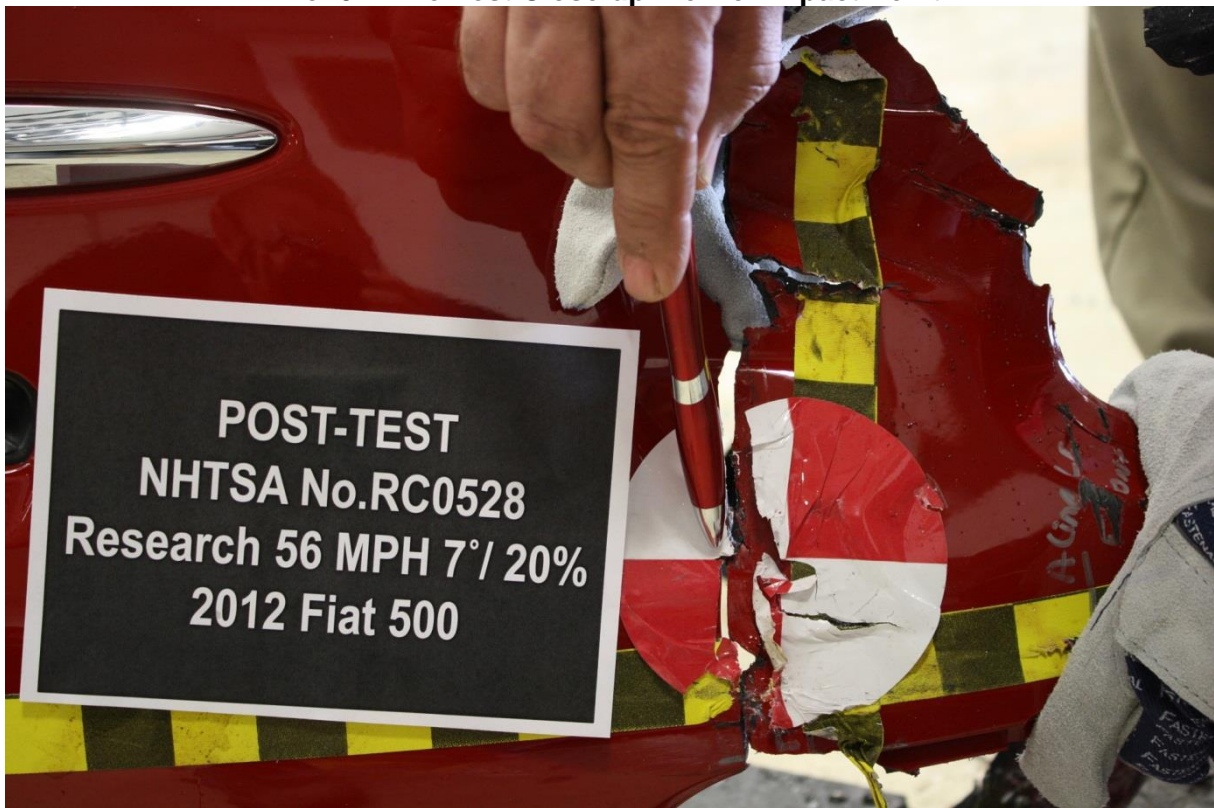
No. 023 Post-Test Close-up View of Impact Point
