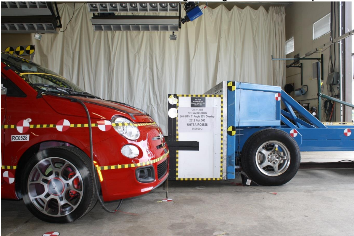
No. 020 Pre-Test Left Side View of RMDB against target vehicle at ideal Impact Point
