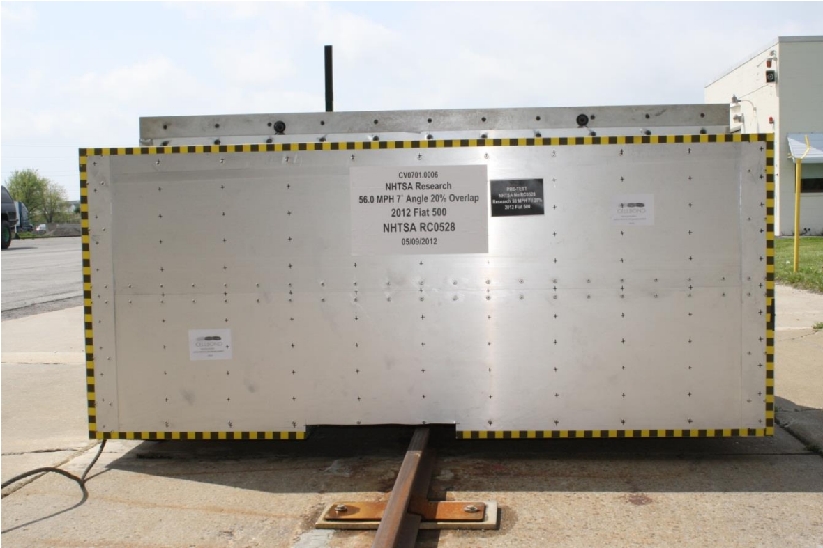
No. 134 Pre-Test Front View of RMDB
