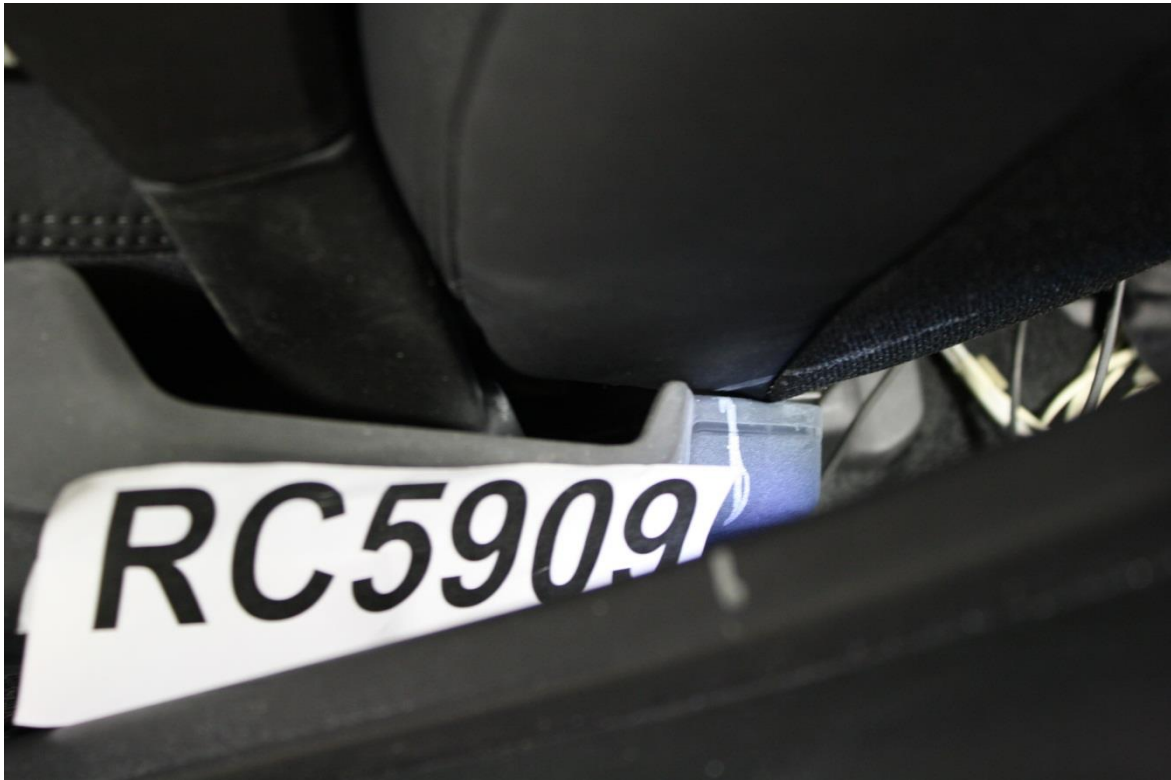
No. 064 Pre-Test Driver Seat Back Position markings
