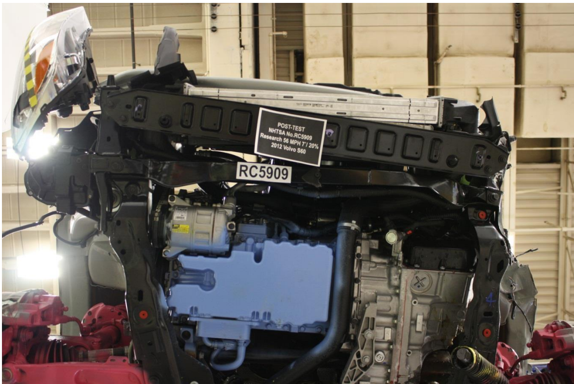
No. 116 Post-Test View of Front Sub-Frame Deformation
