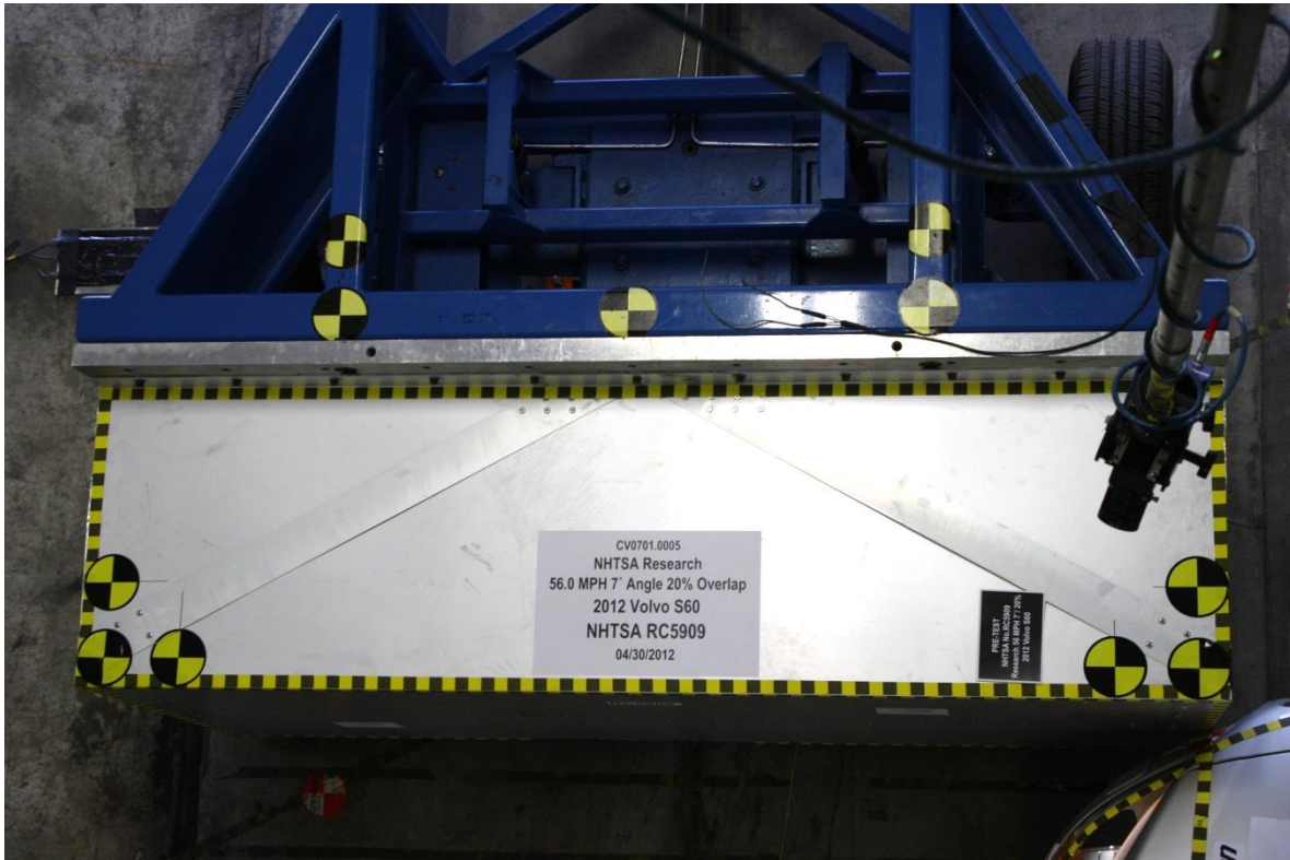
No. 132 Pre-Test Top View of RMDB
