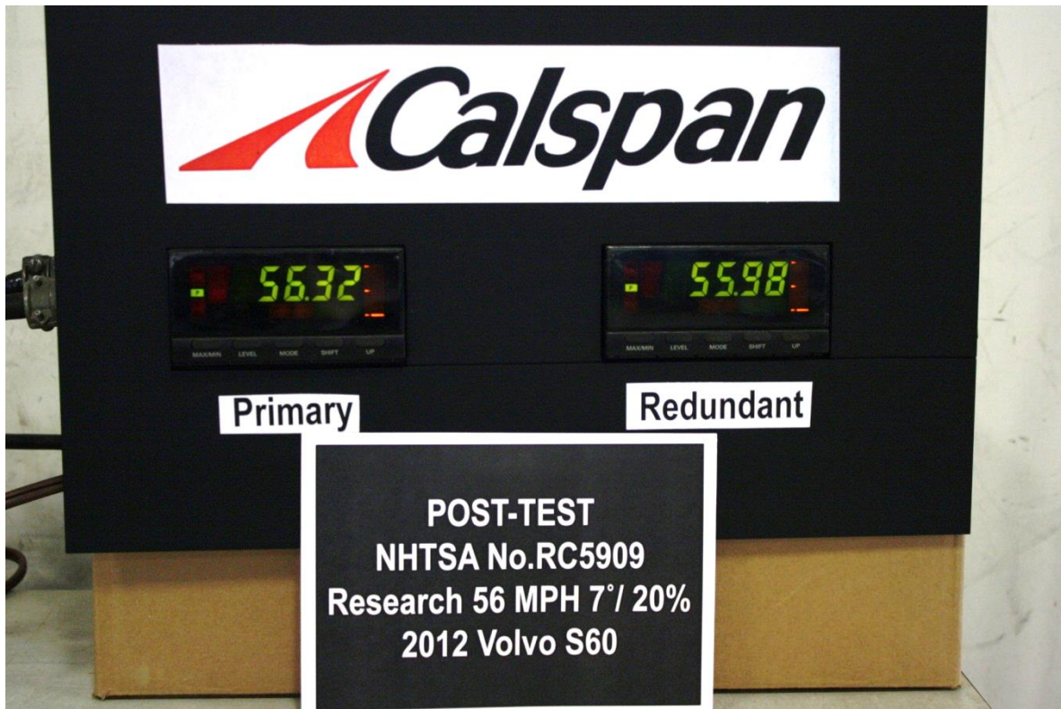
No. 104 Post-Test Speed Trap Readout
