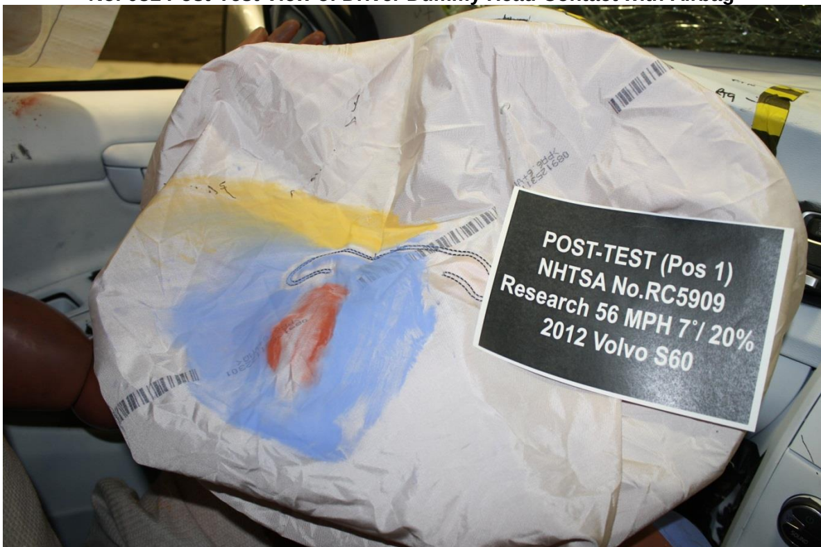
No. 081a Post-Test View of Driver Dummy Head Contact with Airbag
