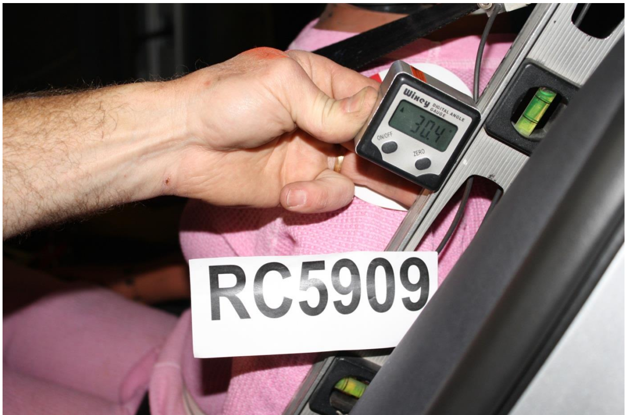
No. 095 Pre-Test Passenger Seat Back Angle
