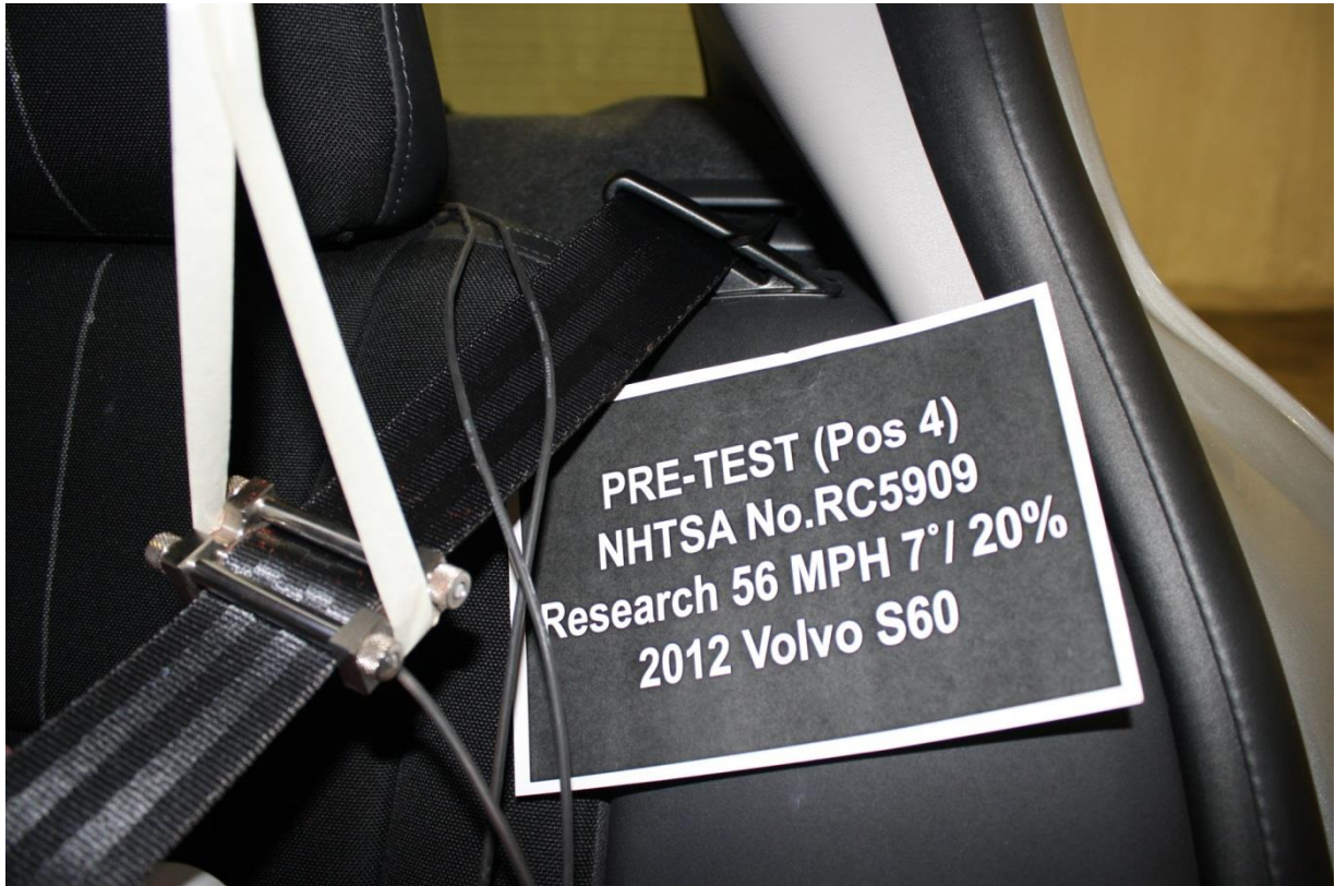
No. 097 Pre-Test Passenger Adjustable D-ring
