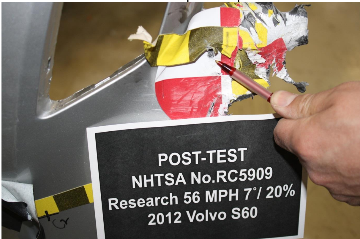
No. 023 Post-Test Close-up View of Impact Point
