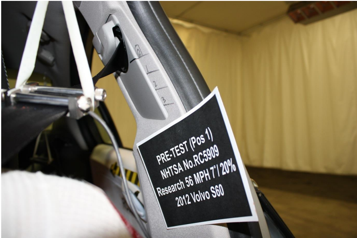
No. 068 Pre-Test Driver Adjustable D-ring
