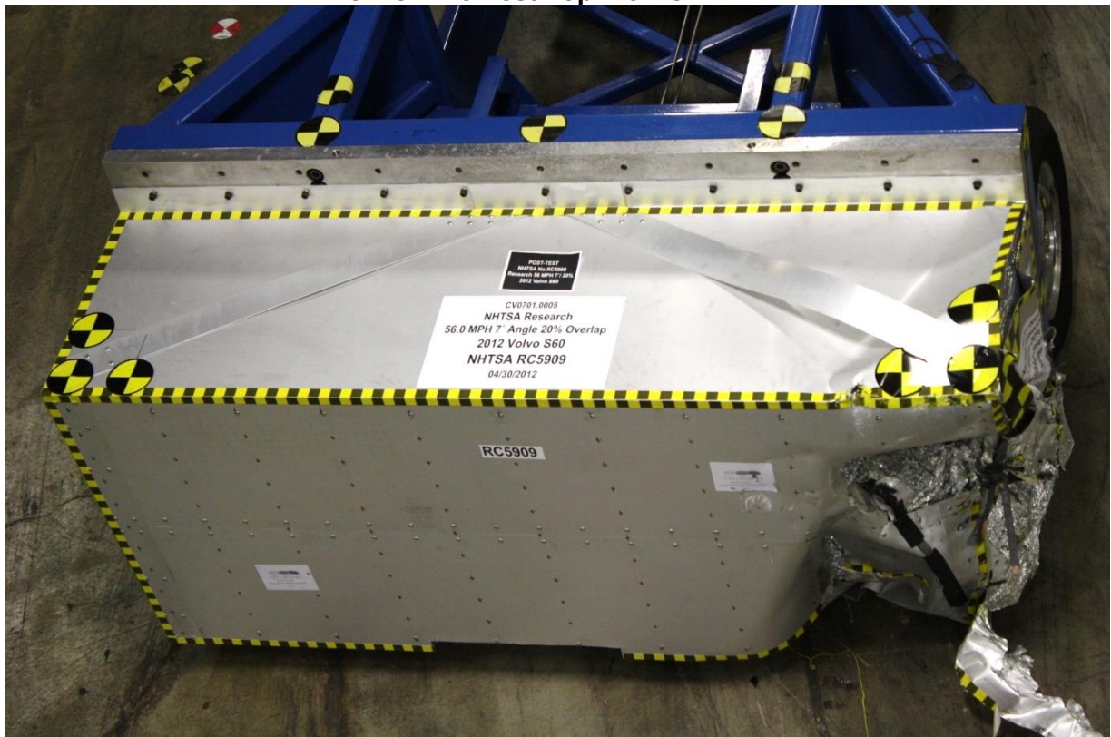
No. 133 Post-Test Top View of RMDB
