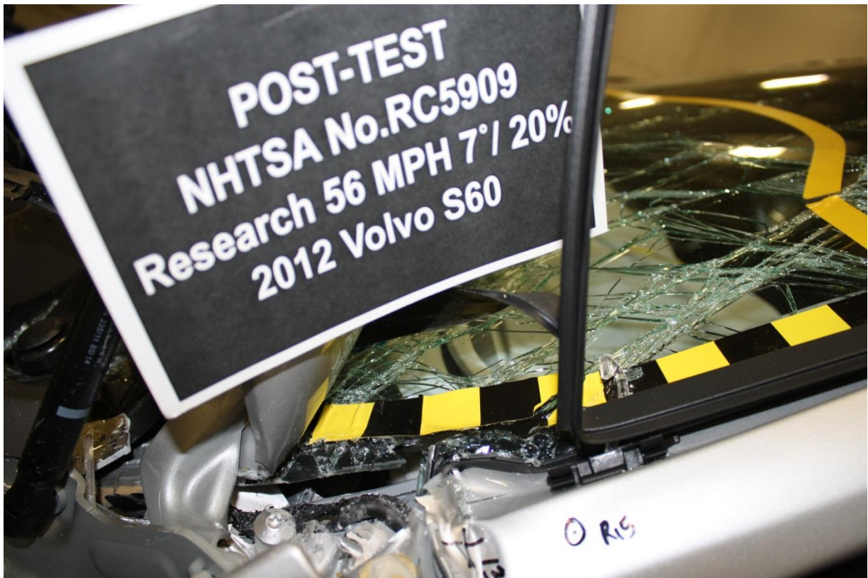
No. 127 Post-Test View of Windshield Separation
