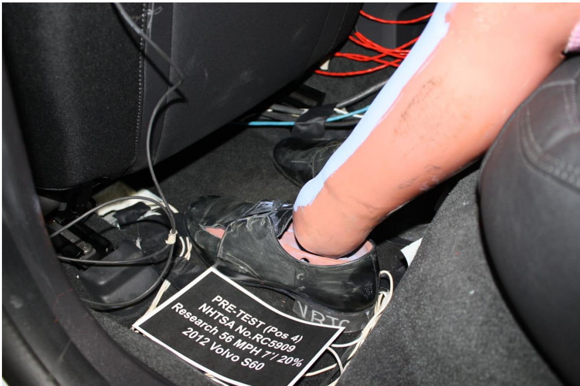
No. 098 Pre-Test View of Passenger Dummy Feet
