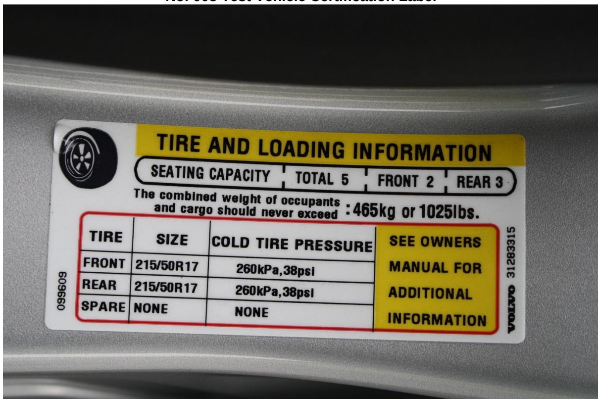
No. 004 Test Vehicle Tire Placard
