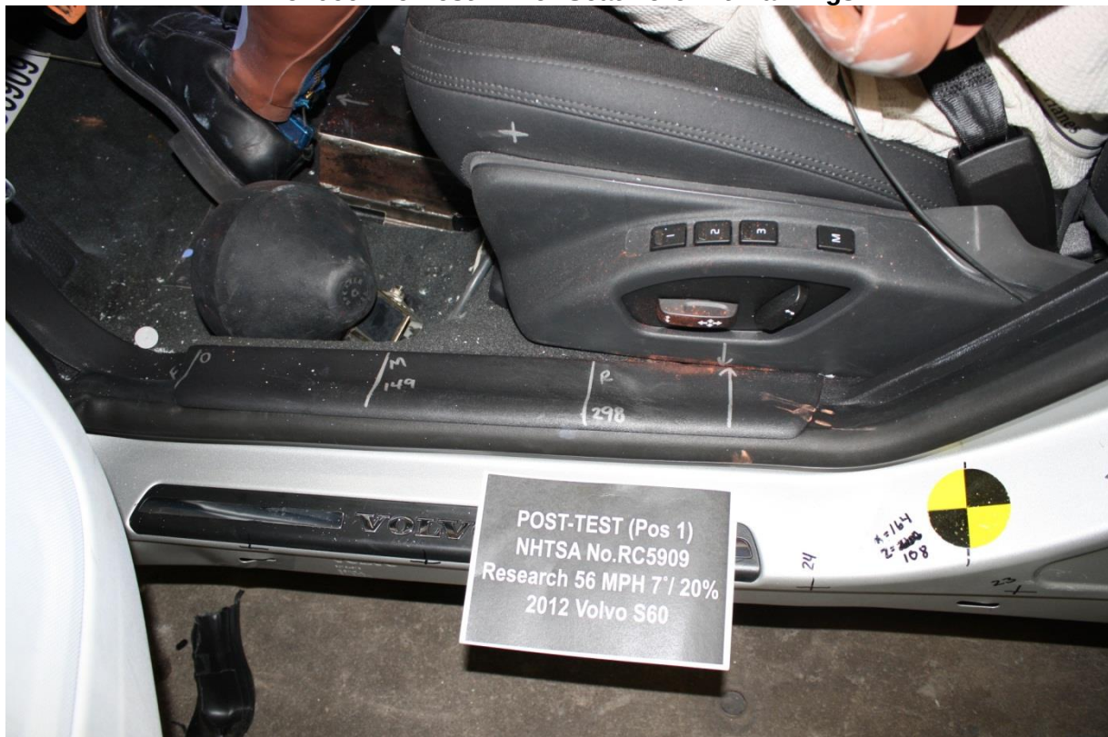
No. 067 Post-Test Driver Seat Fore Aft Markings
