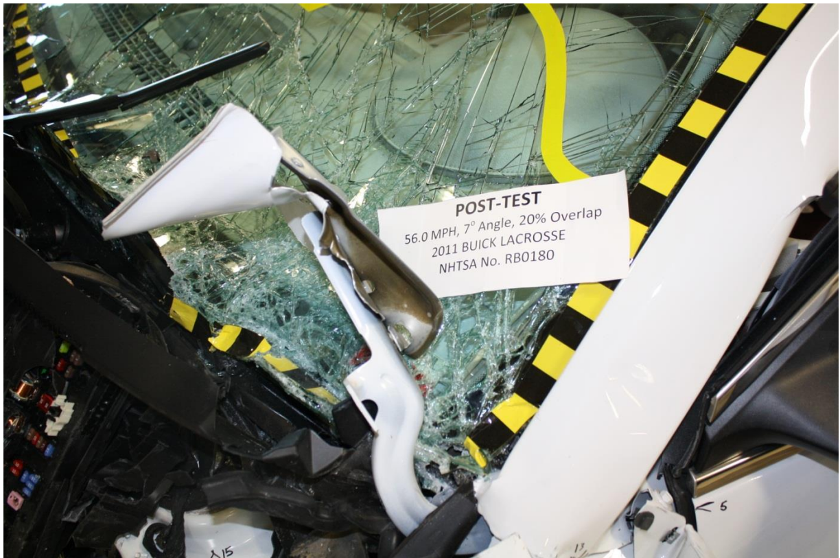
No. 127 Post-Test View of Windshield Separation
