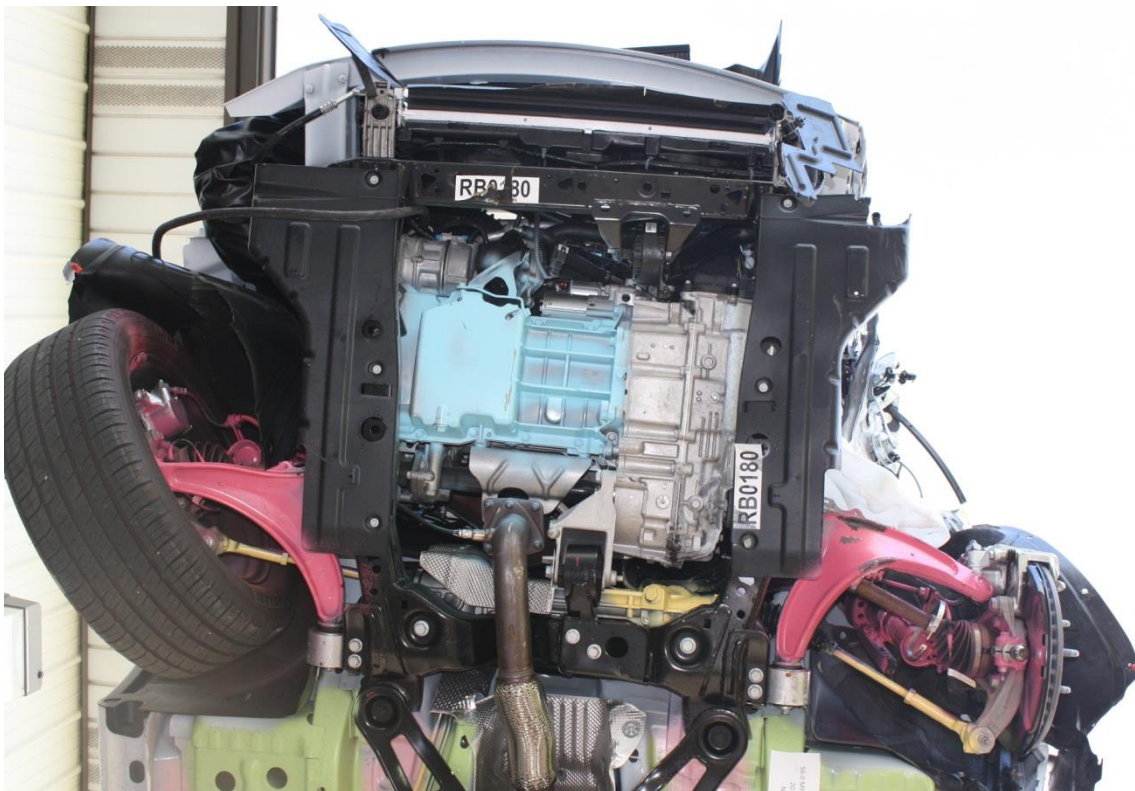
No. 116 Post-Test View of Front Sub-Frame Deformation
