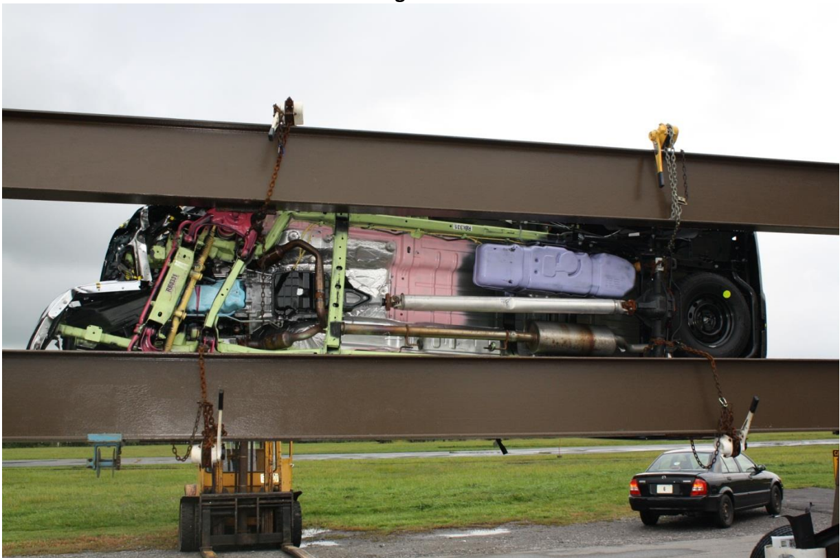
No. 139 Vehicle at 270 Degrees on Static Rollover Device
