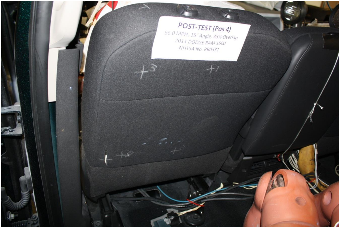
No. 102 Post-Test View of Passenger Dummy Knee Contact with Seatback
