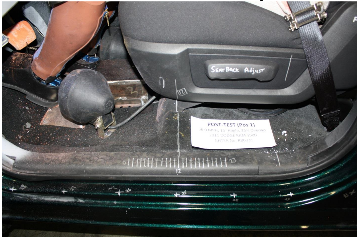
No. 067 Post-Test Driver Seat Fore Aft Markings
