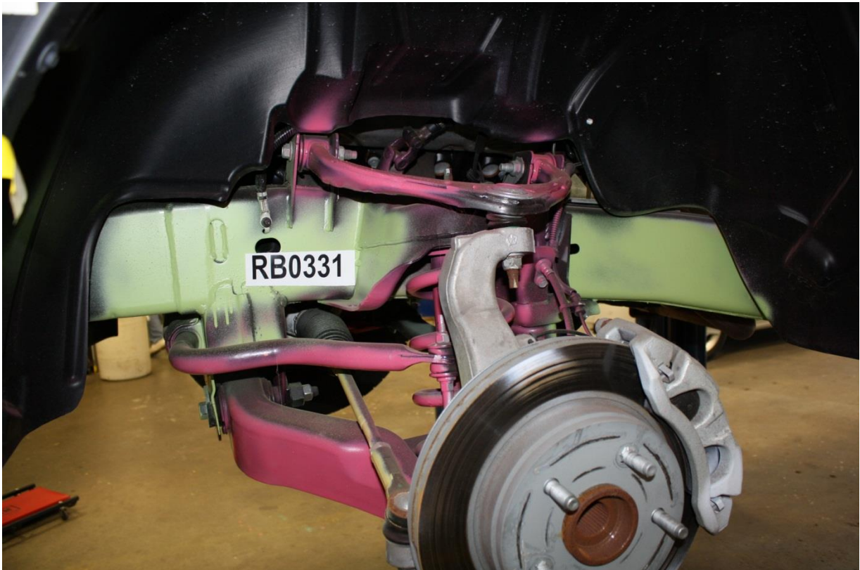
No. 117 Pre-Test Frame Rail with tire removed
