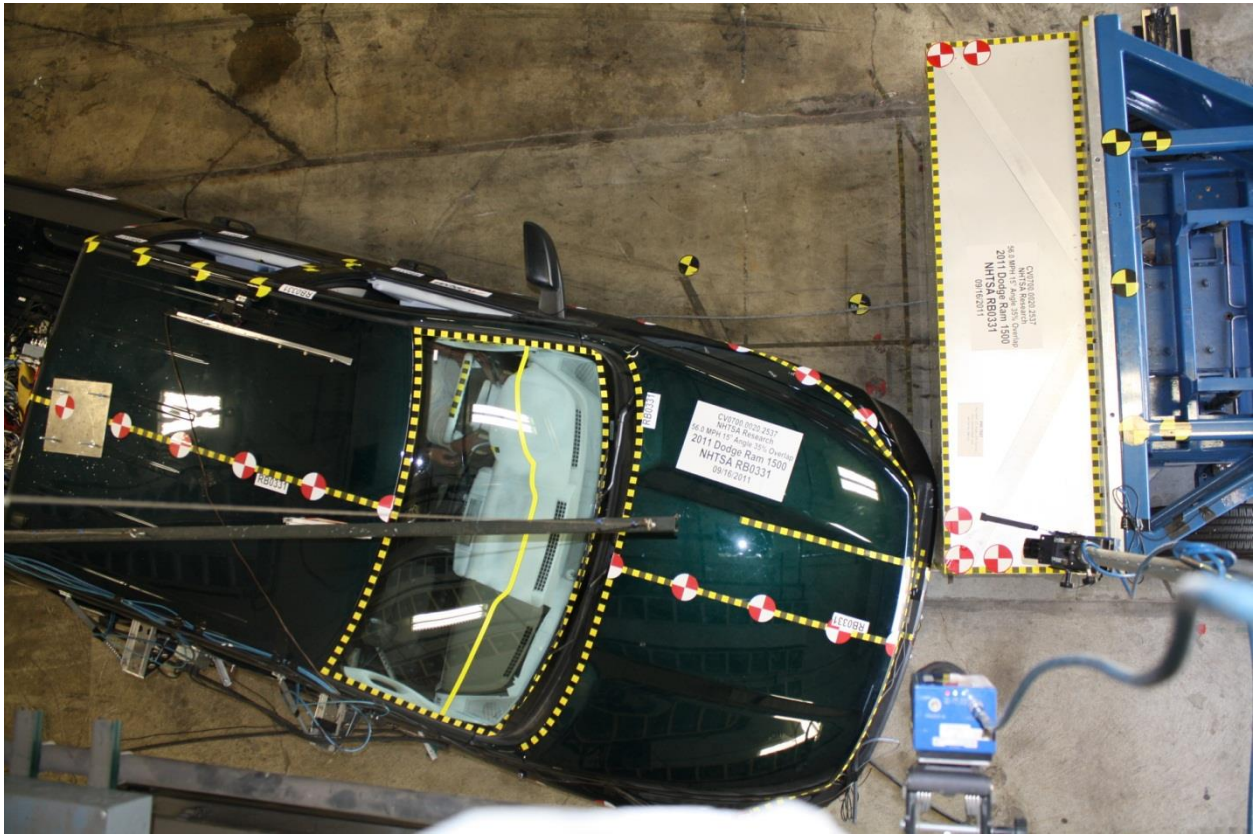
No. 019 Pre-Test Overhead View of RRMDB against target vehicle at ideal Impact Point
