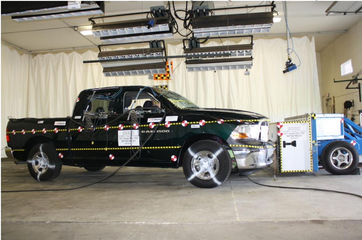
No. 020 Pre-Test Left Side View of RRMDB against target vehicle at ideal Impact Point
