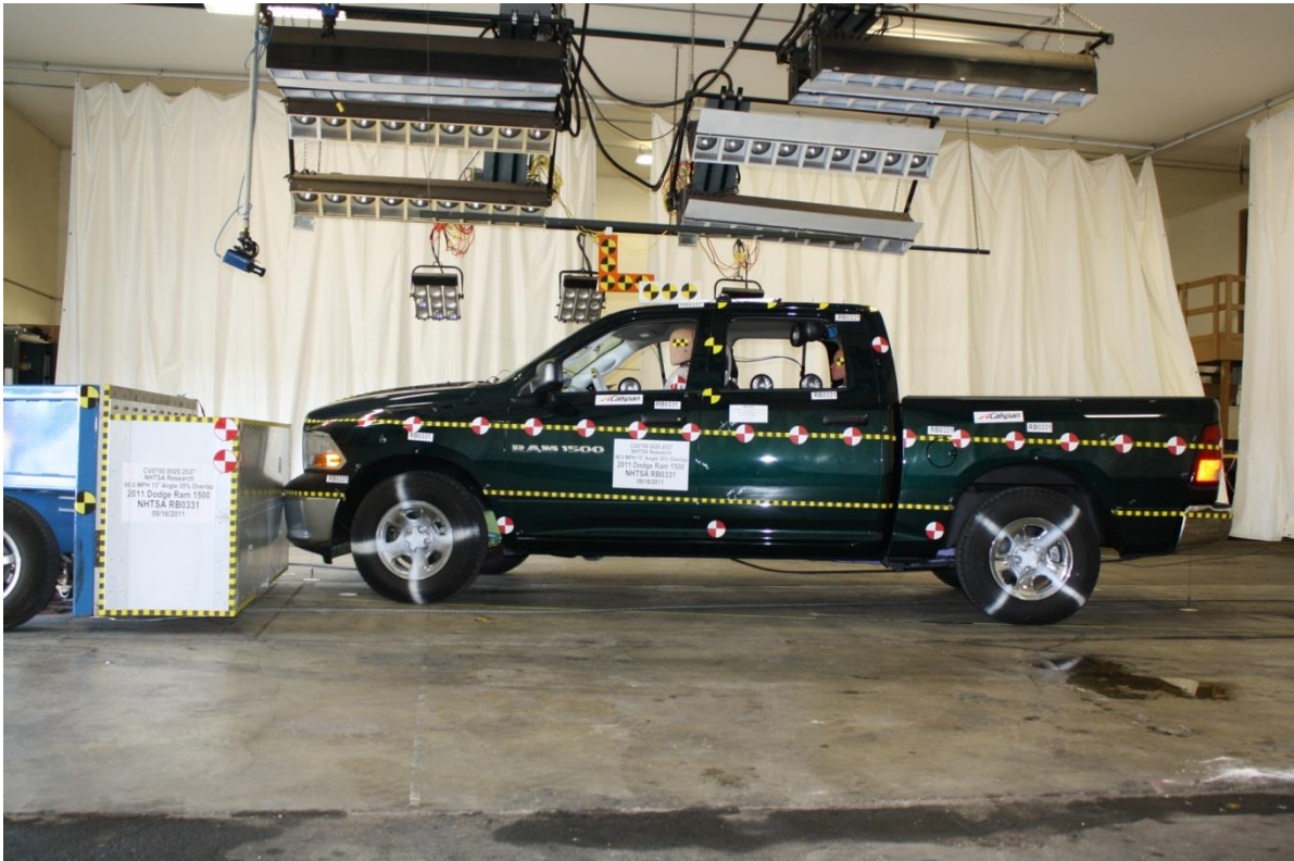
No. 021 Pre-Test Right Side View of RRMDB against target vehicle at ideal Impact Point
